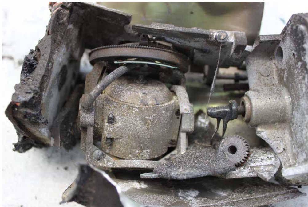
Figure 10: Photograph depicts the rotor housing installed in the gimball ring.
