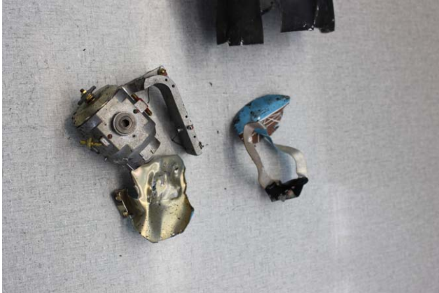
Figure 3: Photograph depicting the rotor housing, fractured and only remaining portion of the gimball ring support.
