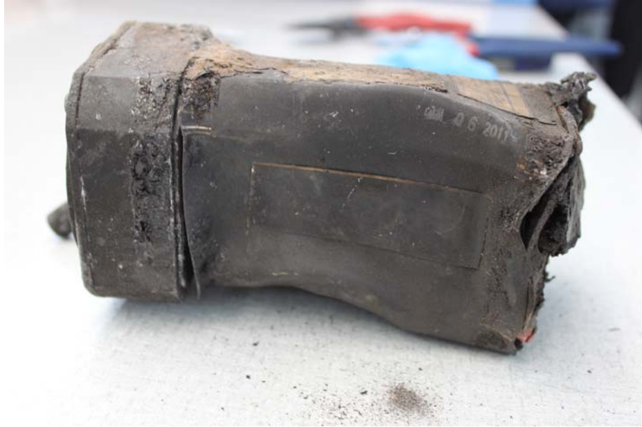
Figure 7: Photograph depicts the impact damage to the side of the directional gyro.
