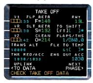
The previous takeoff data (V1, VR, V2, FLX TO values) appear in small blue font beside the corresponding fields. The PFD takeoff speeds are removed from the PFD speed scale. The FLAPS/THS, THR RED/ACC and ENG OUT ACC data, if entered, will remain.
