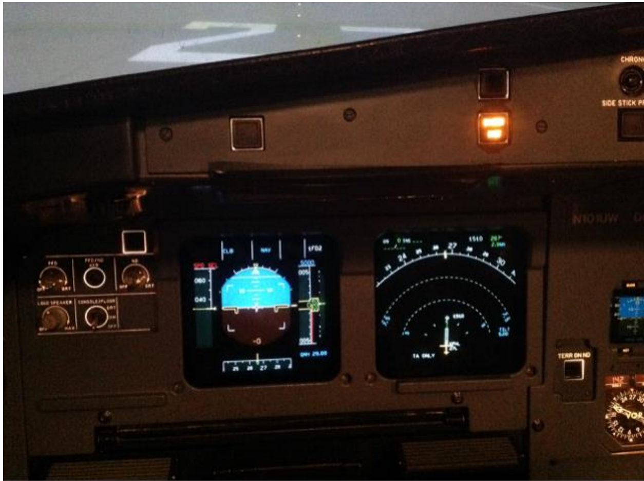
Photo 12: Forward displays (with master caution) when Flex thrust set without an assumed temperature.
