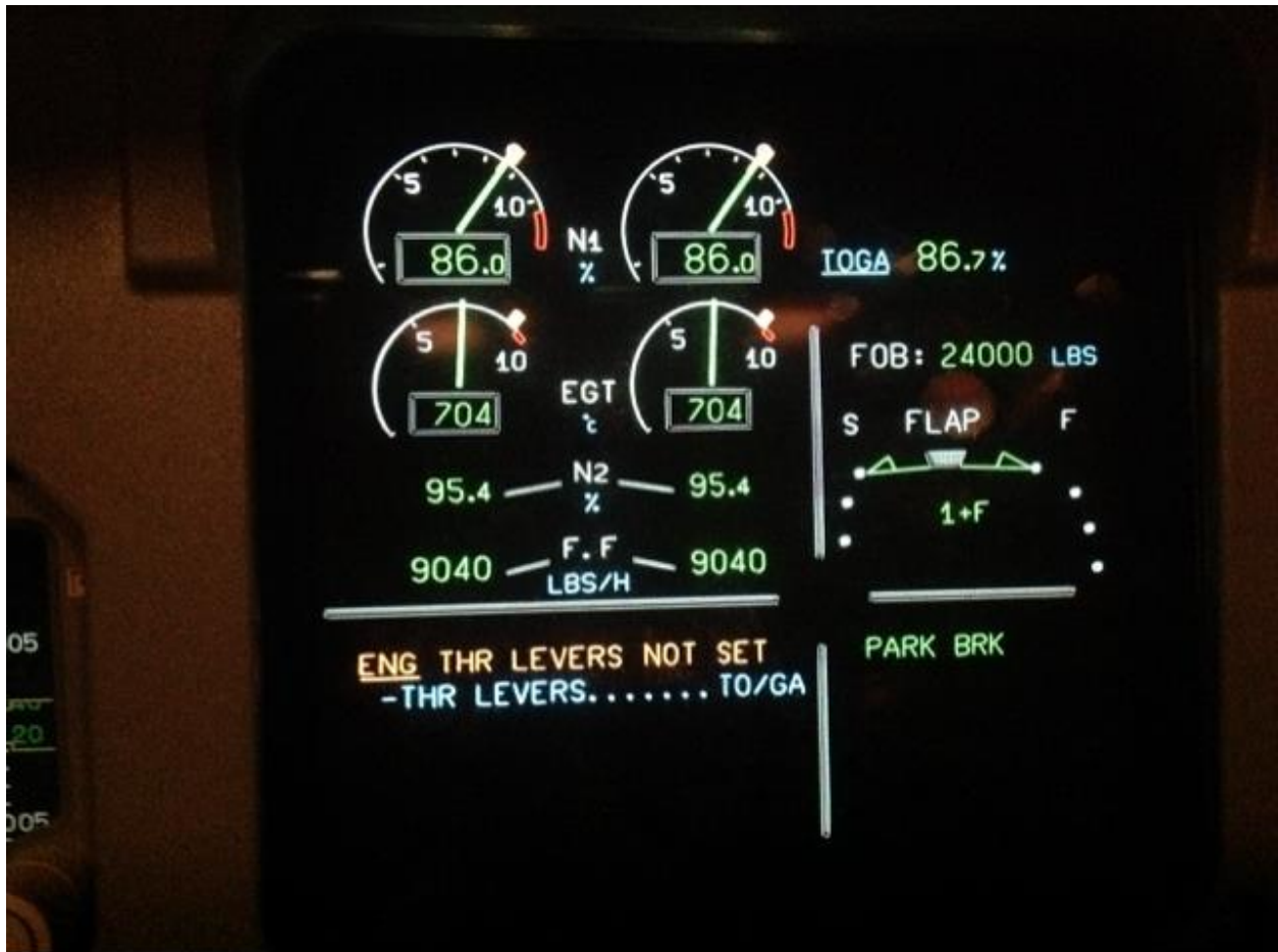
Photo 13: Upper ECAM when Flex thrust set without an assumed temperature.
