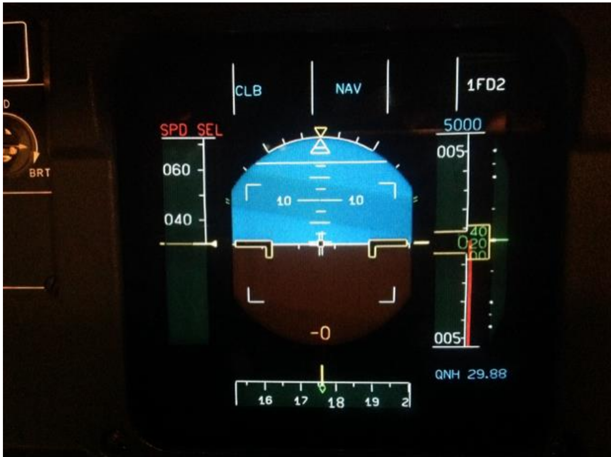
Photo 8: PFD with no V-speeds inserted.
