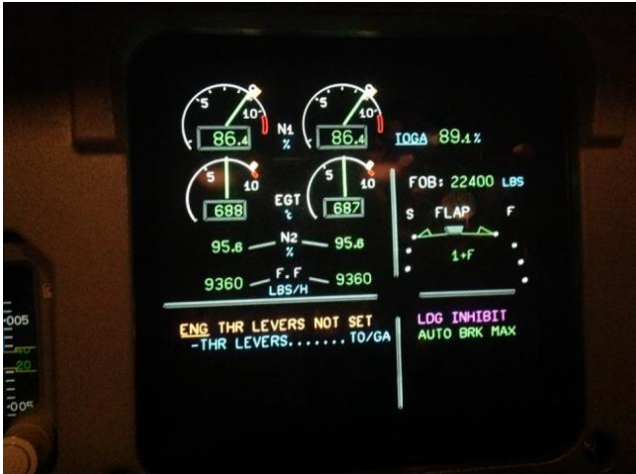
Photo 14: Upper ECAM when thrust set to Flex without assumed temperature as airplane reaches 80 knots and the “retard” aural alert sounded.
