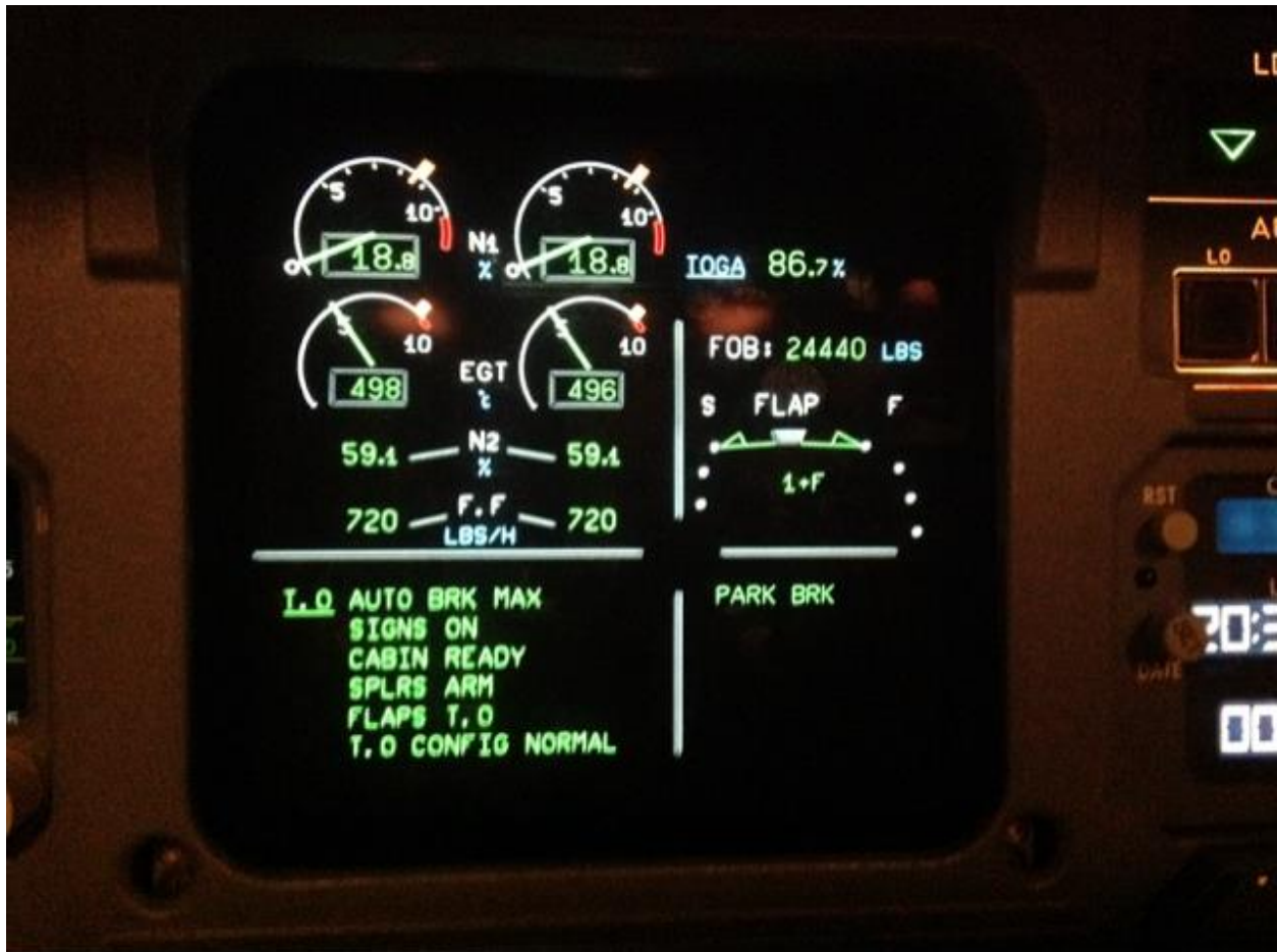
Photo 10: Upper ECAM without Assumed temperature inserted.
