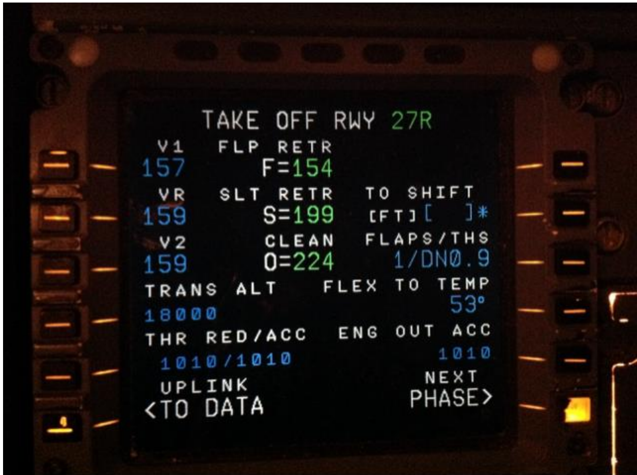
Photo 2: MCDU Takeoff page with V-speeds and Assumed Temperature inserted for PHL runway 27R.
