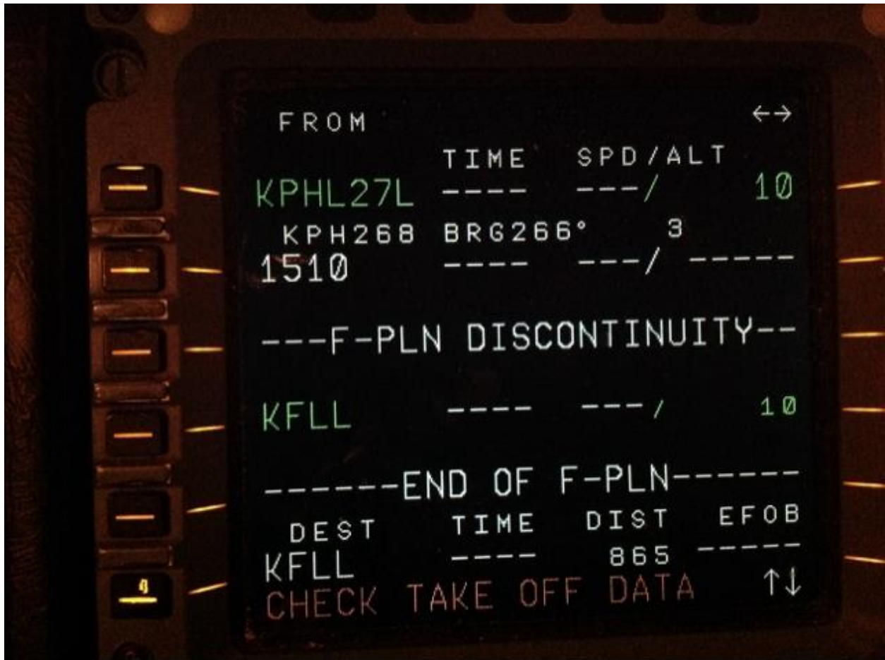
Photo 7: MCDU Takeoff page with 27L inserted and no V-speeds.
