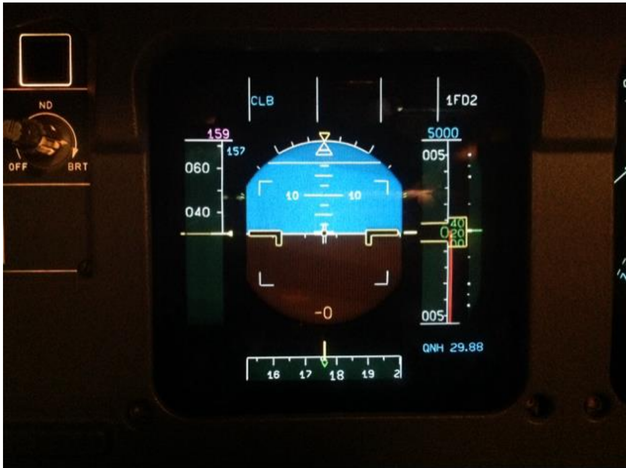
Photo 3: PFD with V-speeds inserted.
