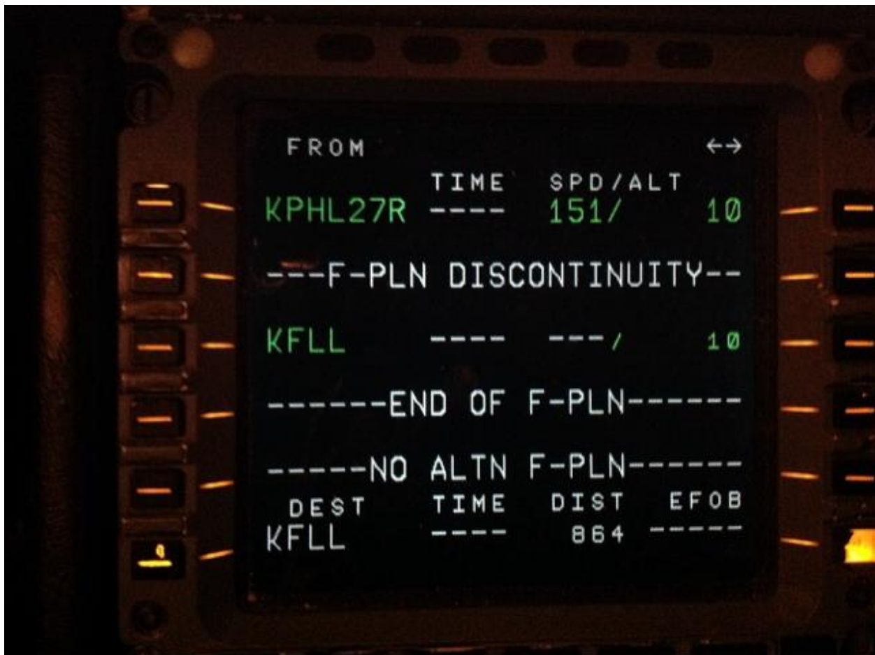
Photo 1: MCDU with PHL runway 27R inserted in the flight plan page.
