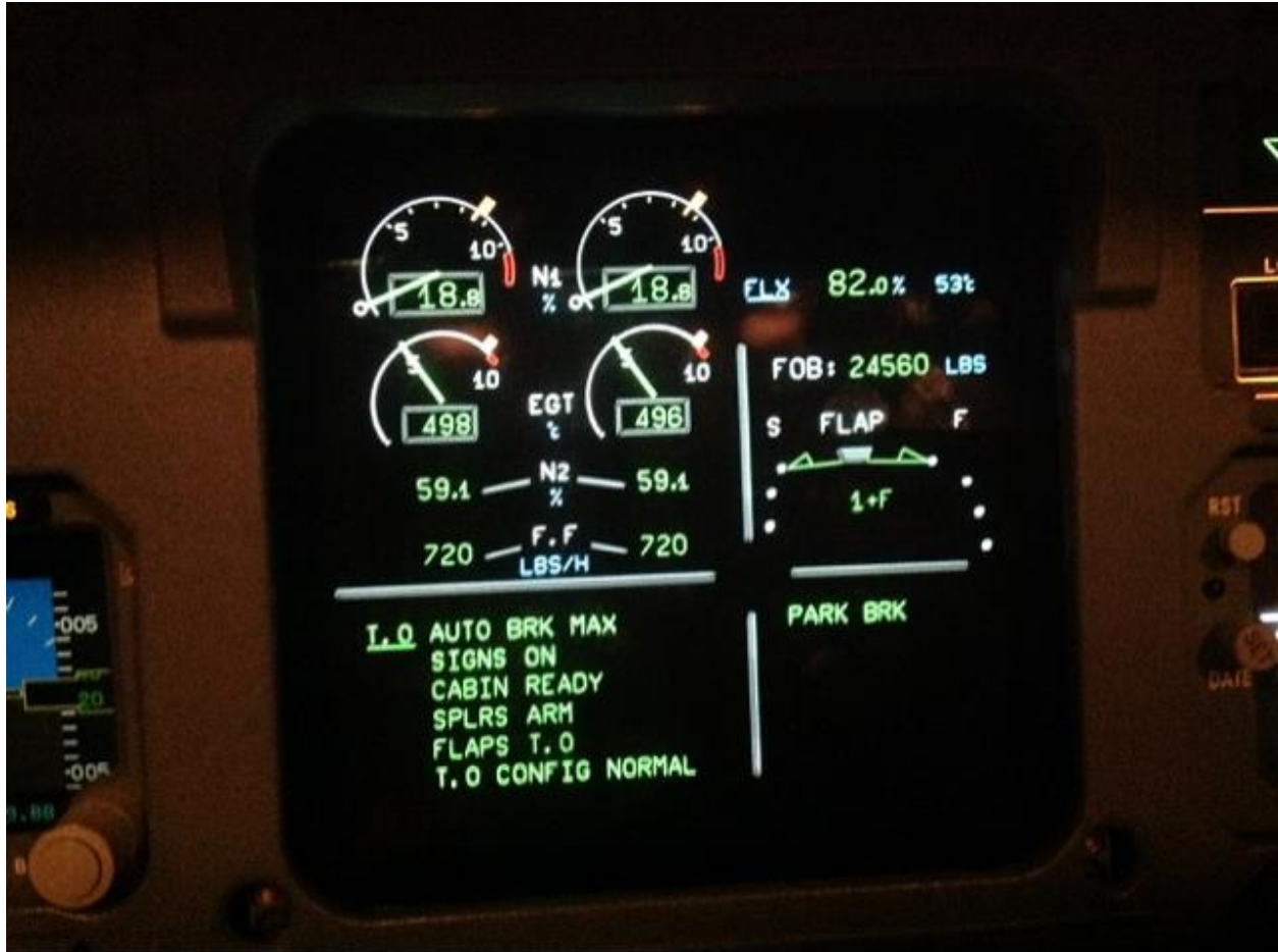
Photo 4: Upper ECAM with Assumed temperature inserted.
