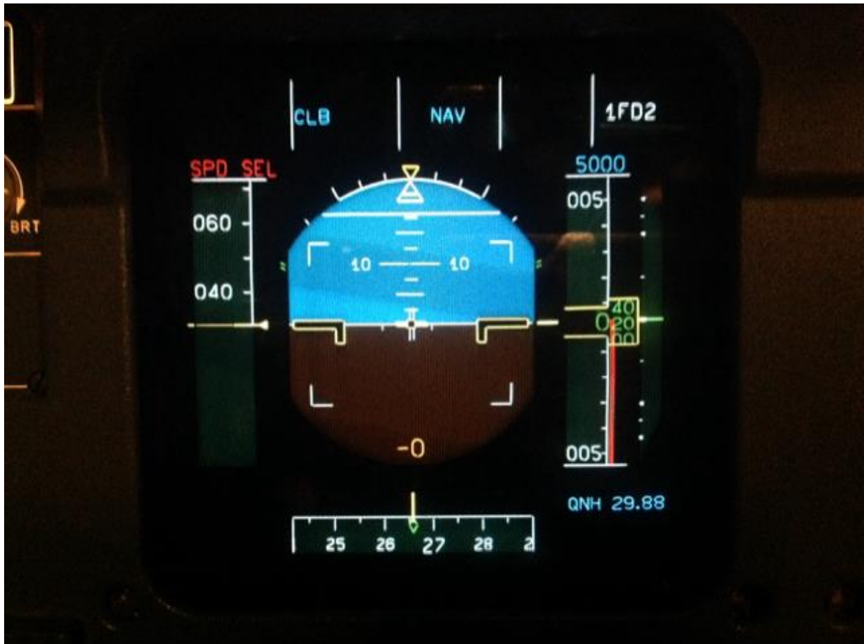
Photo 11: PFD without the V-speeds inserted.
