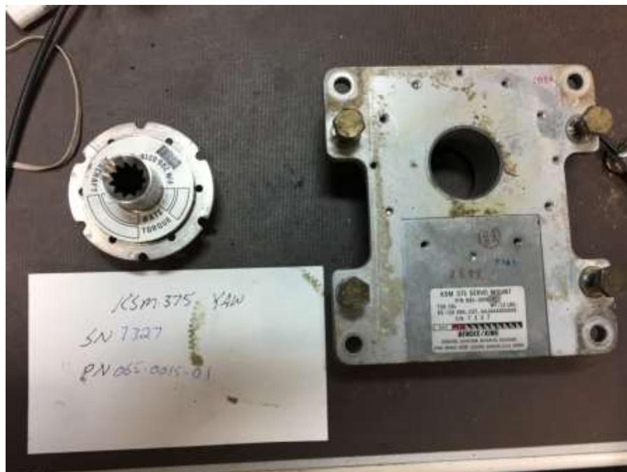
KSM 375 SN 7327 Mounting plate and clutch
