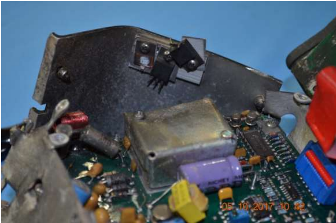
KCP 220 SN 1898 Interior view showing damage to the power supply circuitry.
