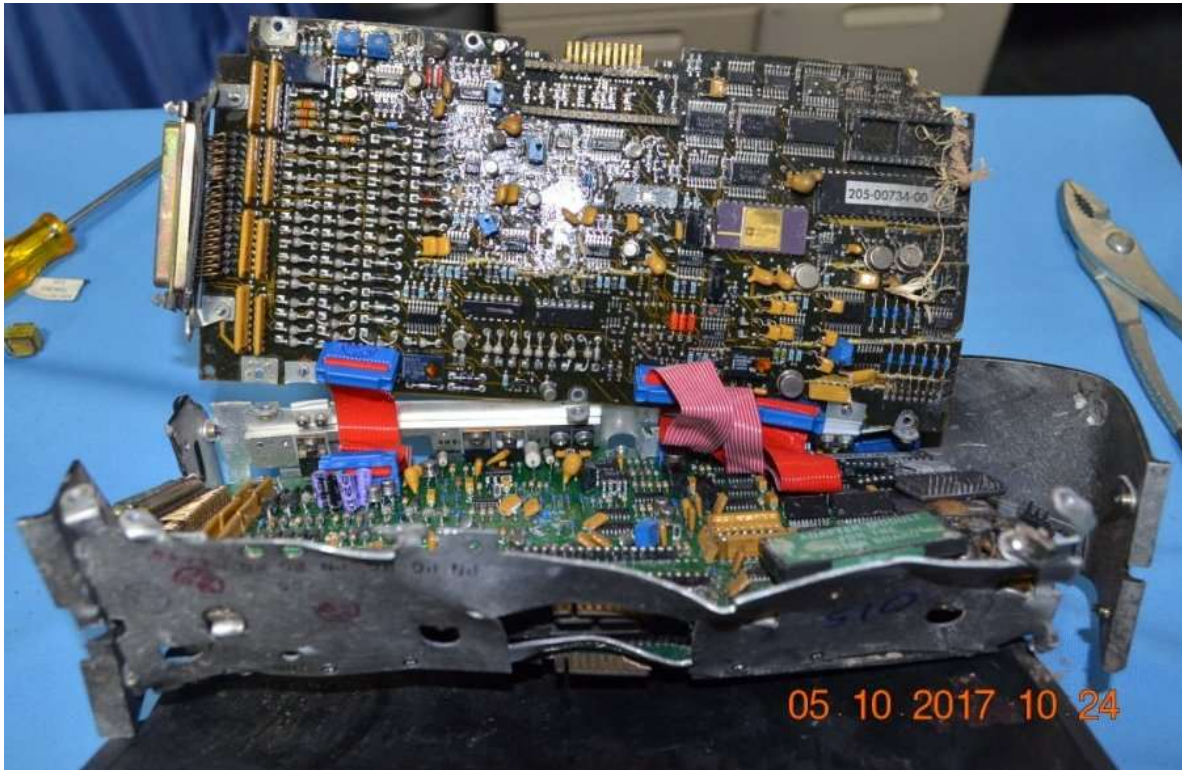
KCP 220 SN 1898 Interior view showing dislodged components and cracked circuit boards.
