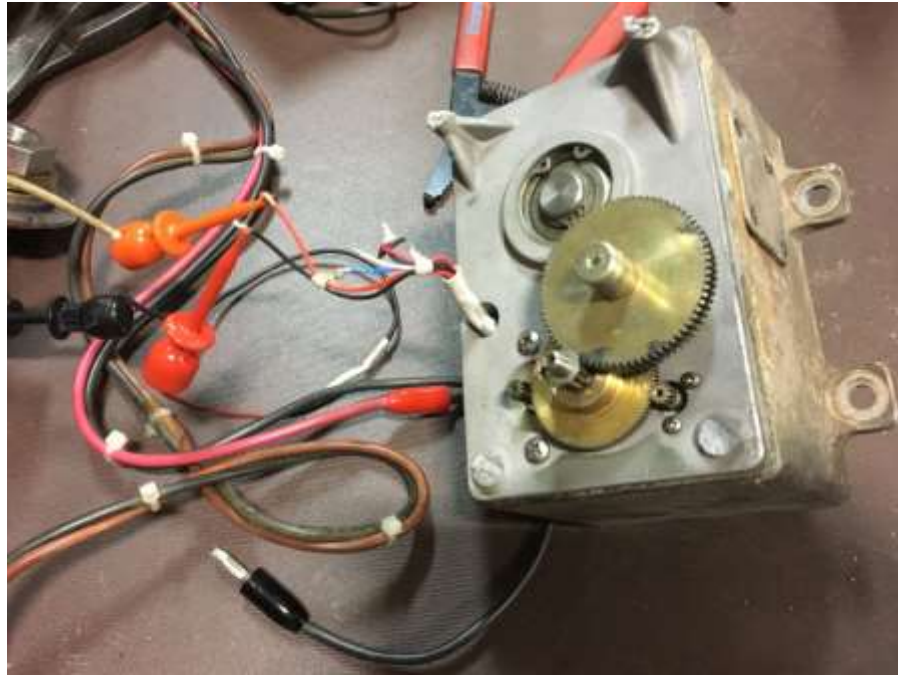
KSA 372 SN 3600 testing of the servo motor and clutch solenoid.
