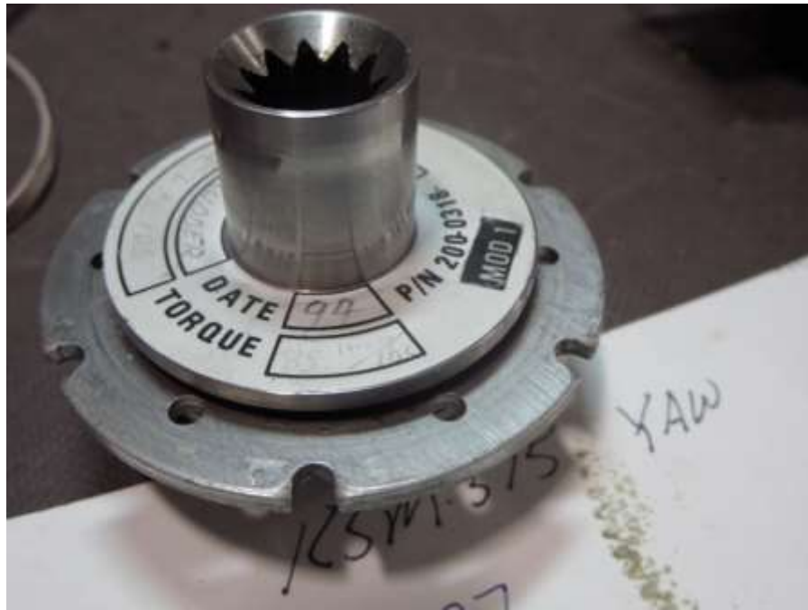
KSM 375 SN 7327 Mounting plate and clutch
