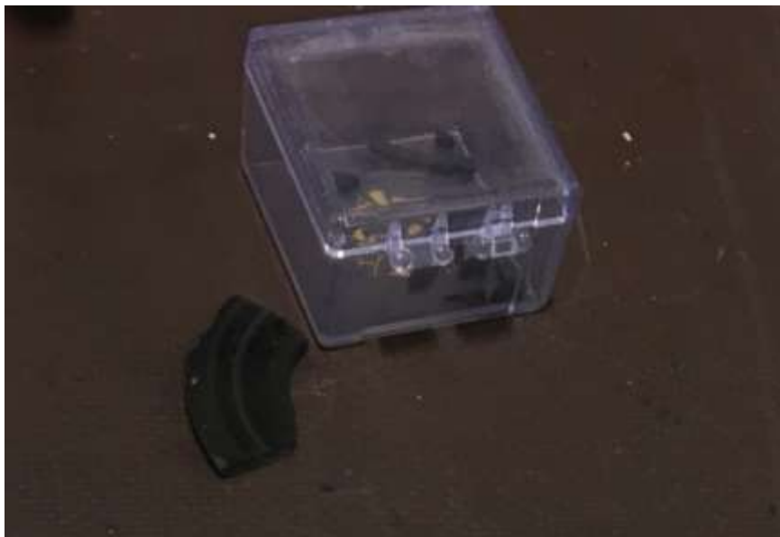
KSM 375 SN 7301 Collected portions clutch disk.
