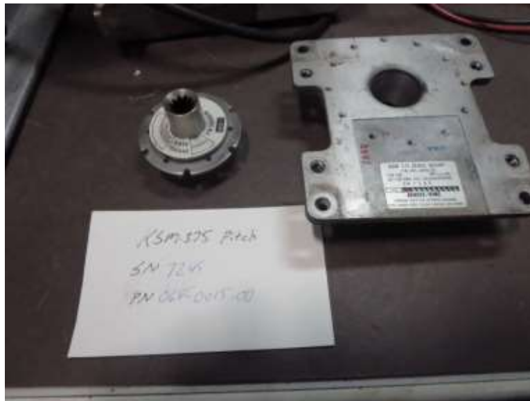
KSM 375 SN 7245 Servo mount with clutch removed for testing
