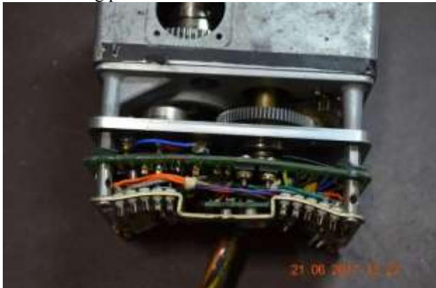
Side view of servo with dust cover removed. The rear component mounting plate bent inward toward circuit board.
