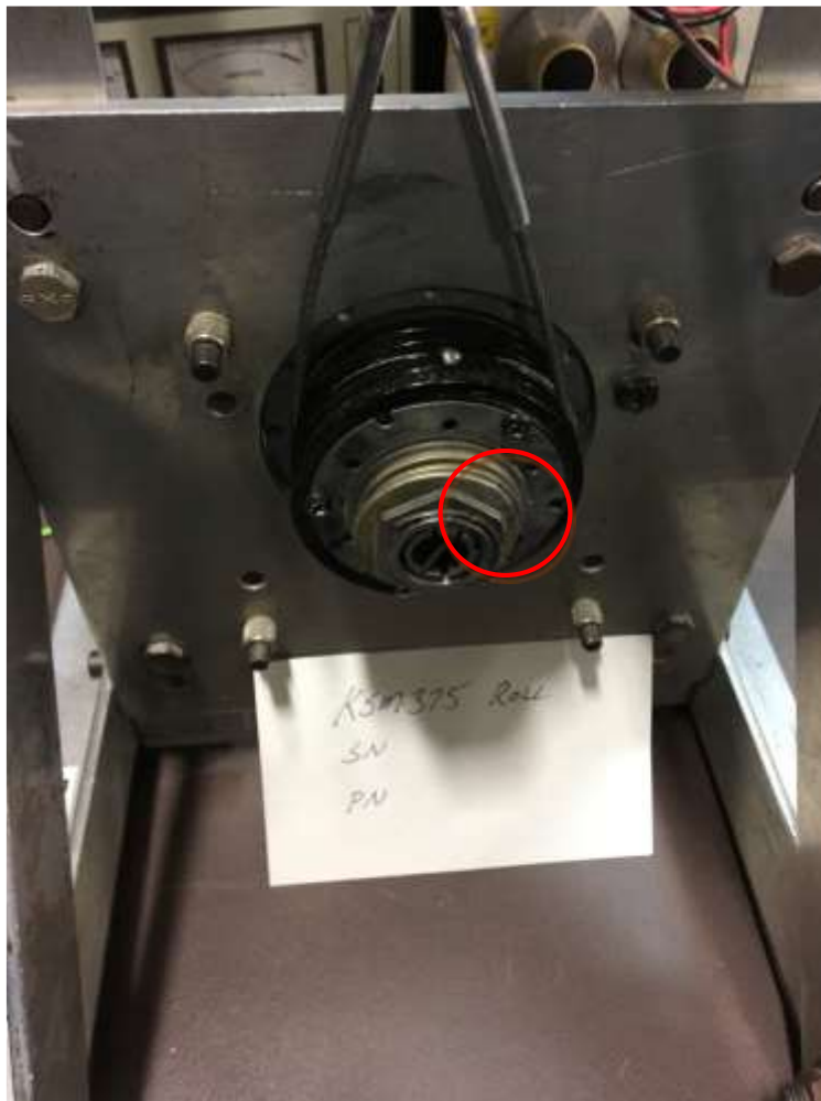
KSM 375 SN 7301 Impact damage to clutch
