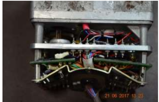
Opposite side view of the rear component mounting plate bent inward toward circuit board.
