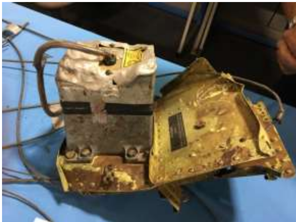
Crush damage at rear of the dust cover. Tear in dust cover.
