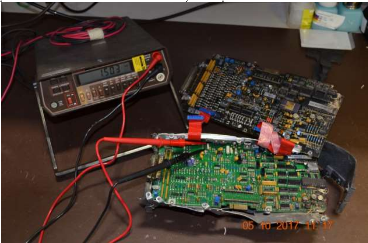
KCP 220 SN 1898 Interior view showing R 259 (attached to clip leads).
