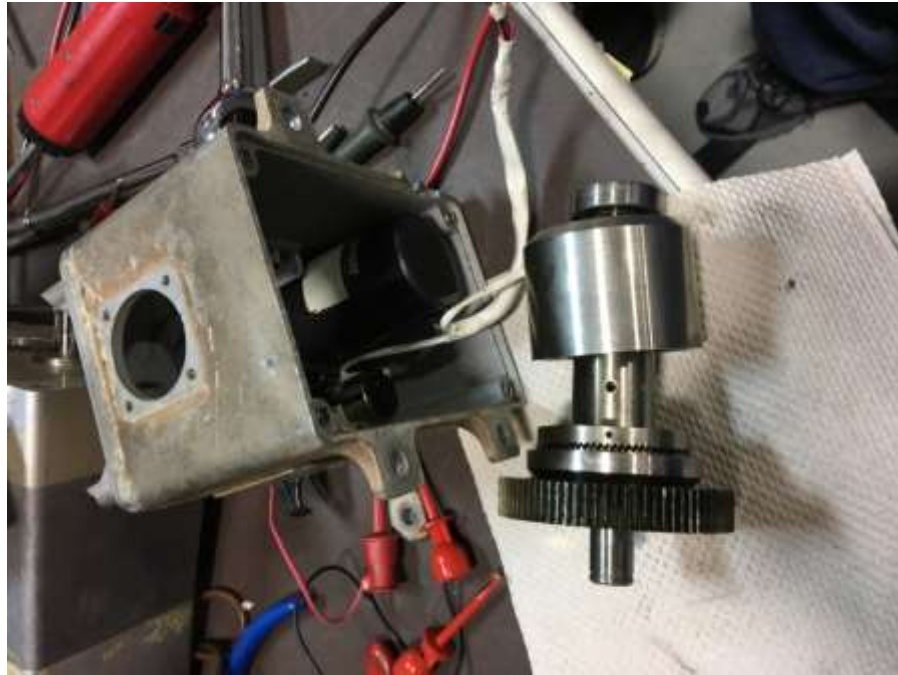
KSA 372 SN 3600: Gear train removed for examination.
