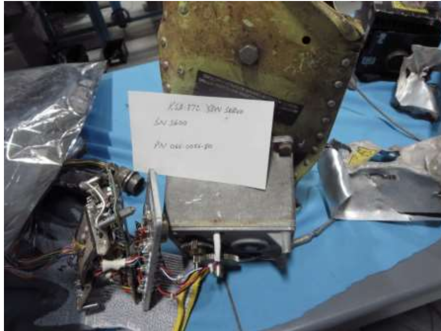
KSA 372 SN 3600 with dust cover removed.
