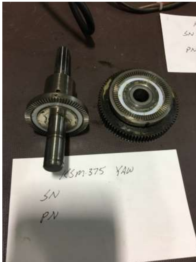
KSA 372 SN 3600: Gear train disassembled to examine “poker chip” gear face.
