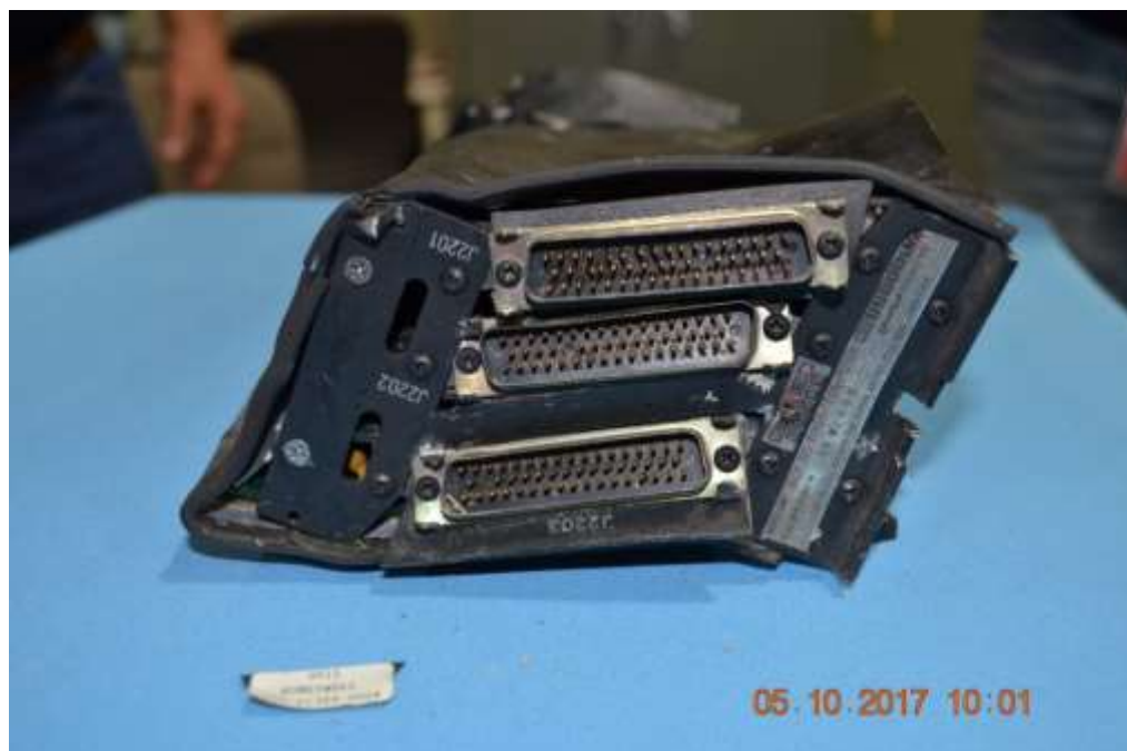
KCP 220 SN 1898 End view showing unit twisting.
