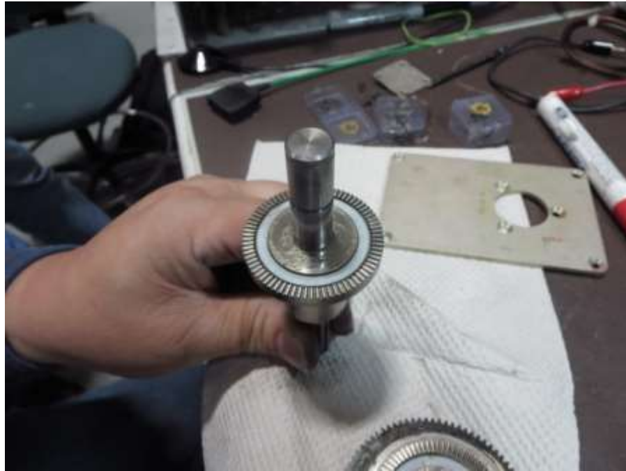
KSA 372 SN 3600: Gear train disassembled to examine “poker chip” gear face.
