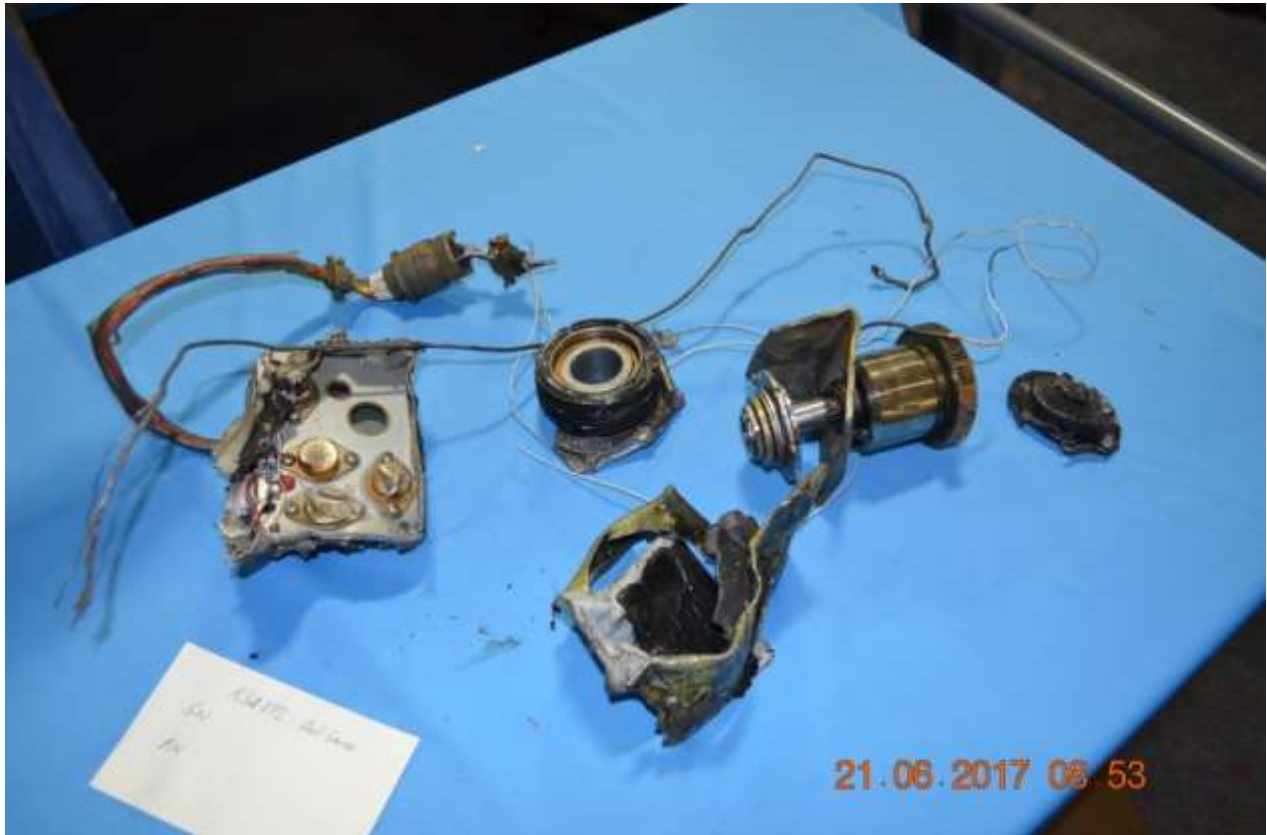
KSA 372 Roll Servo mounting plate and clutch
