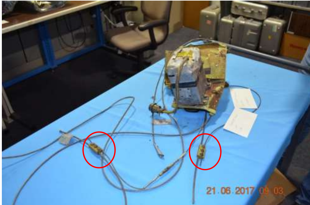
Bridal cable control clamps are intact.
