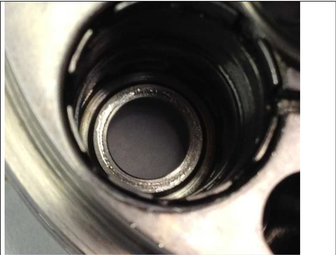
relief valve seat wear detail (Damper S/N 1660B)
