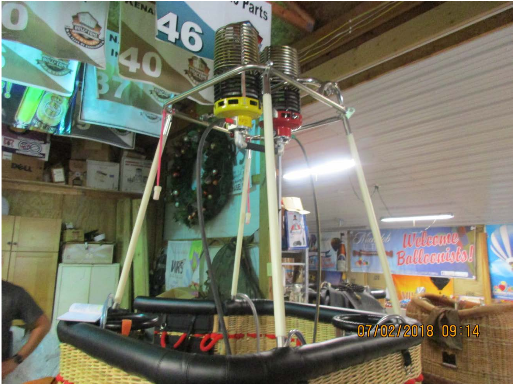
Photo 4 – Balloon Basket and Burners
