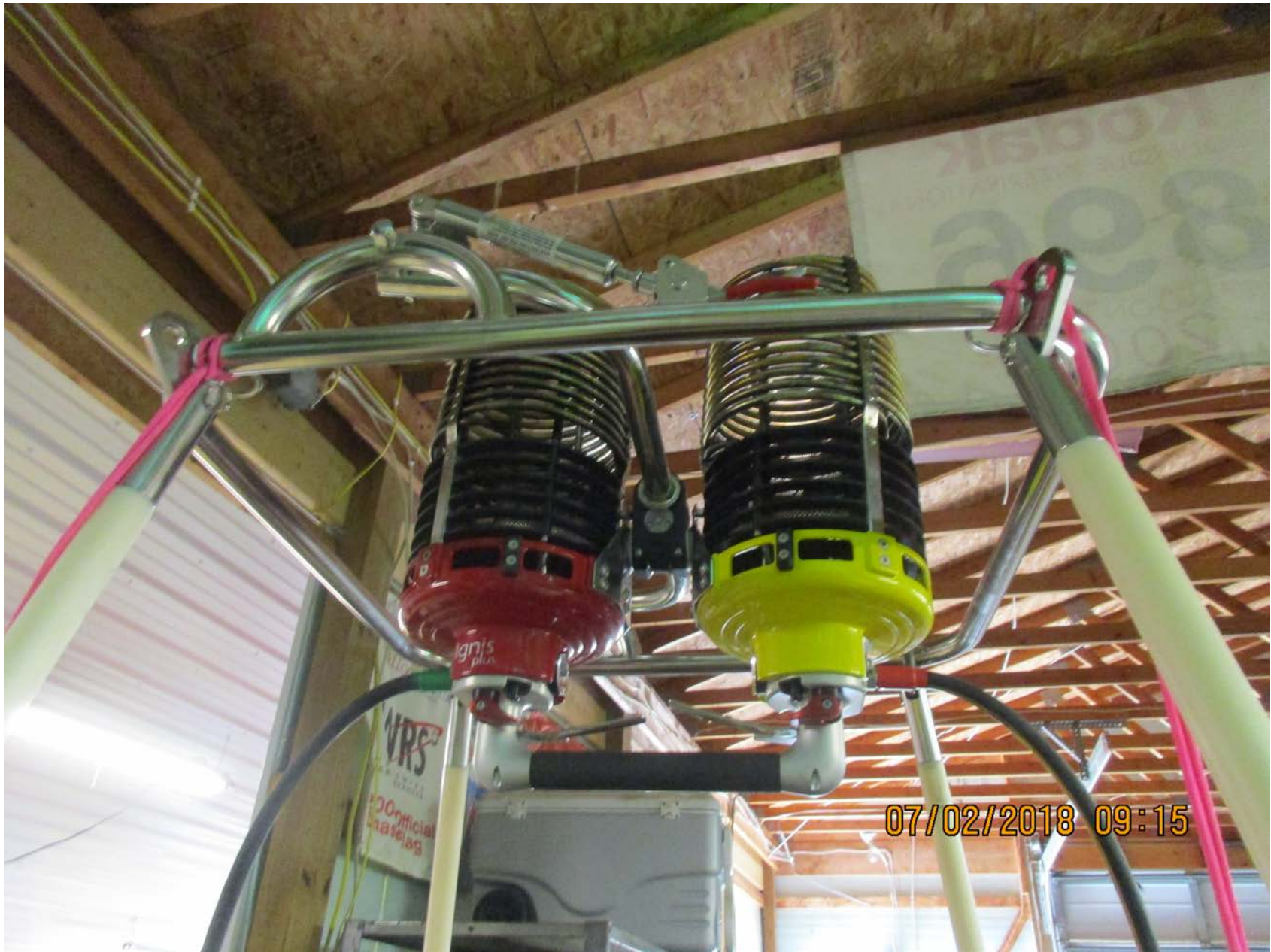
Photo 5 – Balloon Burner System
