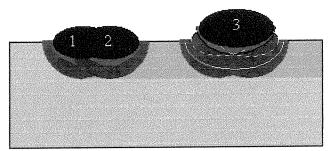
The first layer of weld should consist of small beads, deposited using low heat input to ensure minimum penetration into the parent metal. This can be achieved by using small electrodes, welding in the horizontal position, and adjusting the angle of the electrode or torch to minimise penetration. Great care must be taken to avoid hydrogen cracking and lack of fusion defects.
