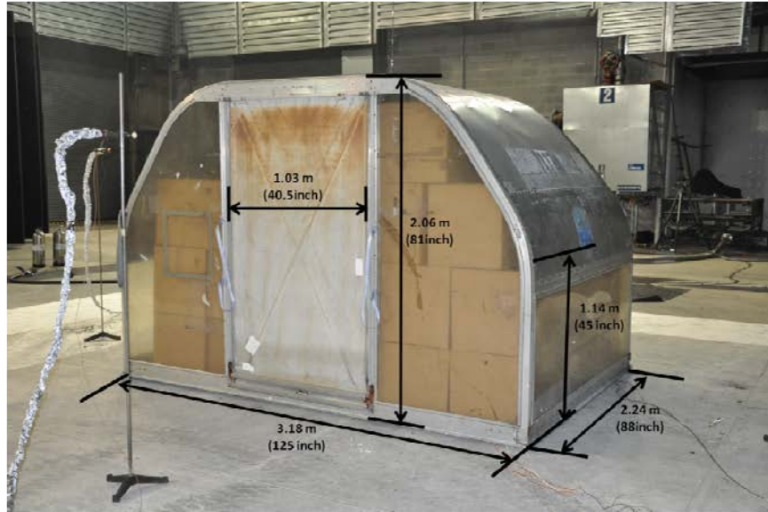
Figure 3. Test setup for Test 1 and Test 2 (6561_201149.JPG)
