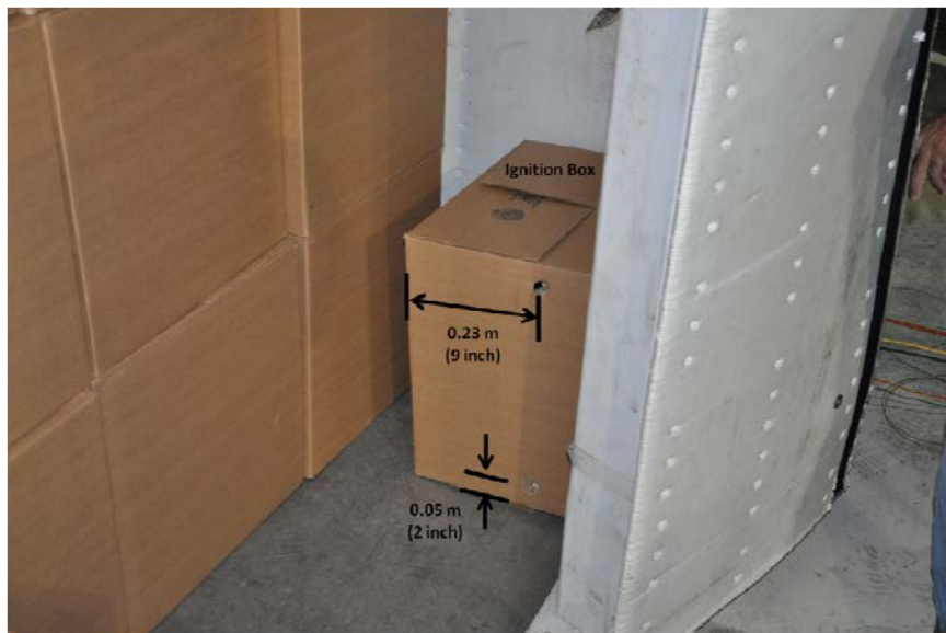
Figure 6. Ignition box (6564_201516.JPG)
