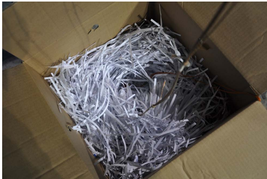
Figure 3. Shredded paper (6 mm wide) in box for Test 4 (6555_200689.JPG)
