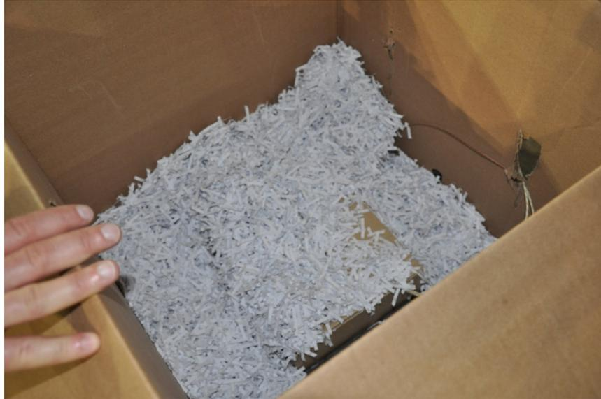
**Figure 7. Configuration of fuel load in ignition box in Test 4 (6558\_200977.JPG)**
