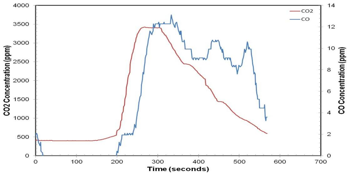
**Figure 126. Carbon monoxide and carbon dioxide concentrations**
