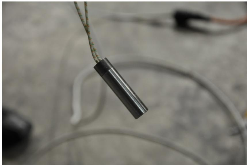
**Figure 10. Cartridge heater (6557\_200845.JPG)**
