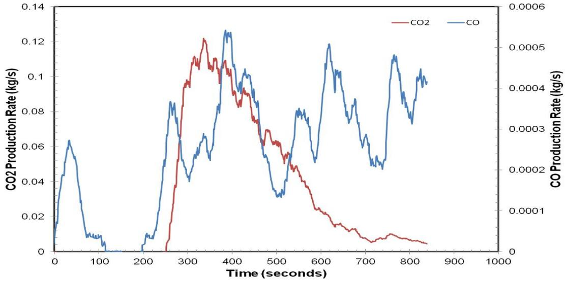
**Figure 20. CO and CO<sub>2</sub> production rates**
