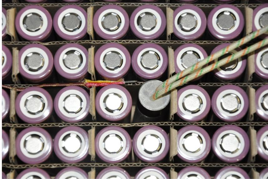
**Figure 11. Cartridge heater location in battery array (6557\_200855.JPG)**
