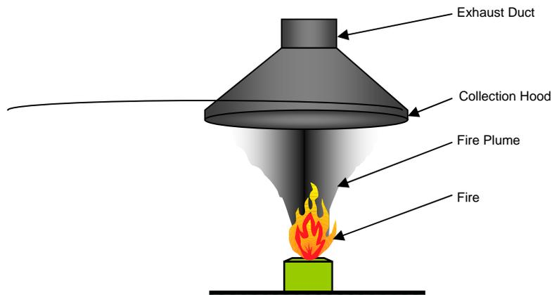
**Figure 13. Typical products collector hood**
