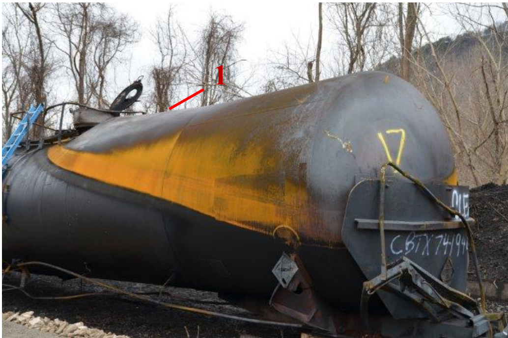
Figure 44: A-end head and vapor space bulging.
