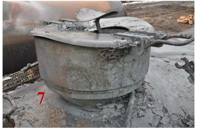
Figure 49: Top fittings protective housing thermal damage.
