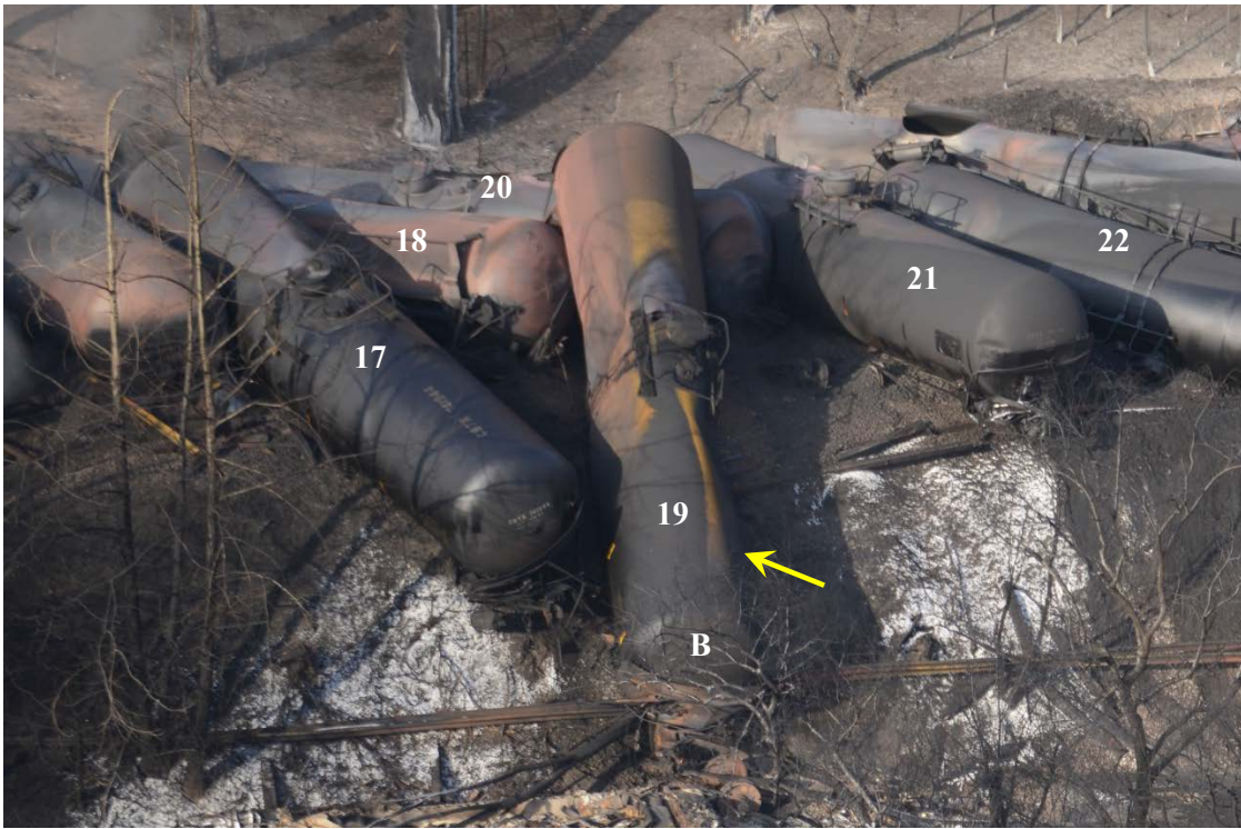
Figure 51: Center of tank car pileup, highlighting location of CBTX 742778, line number 19 (arrow).
