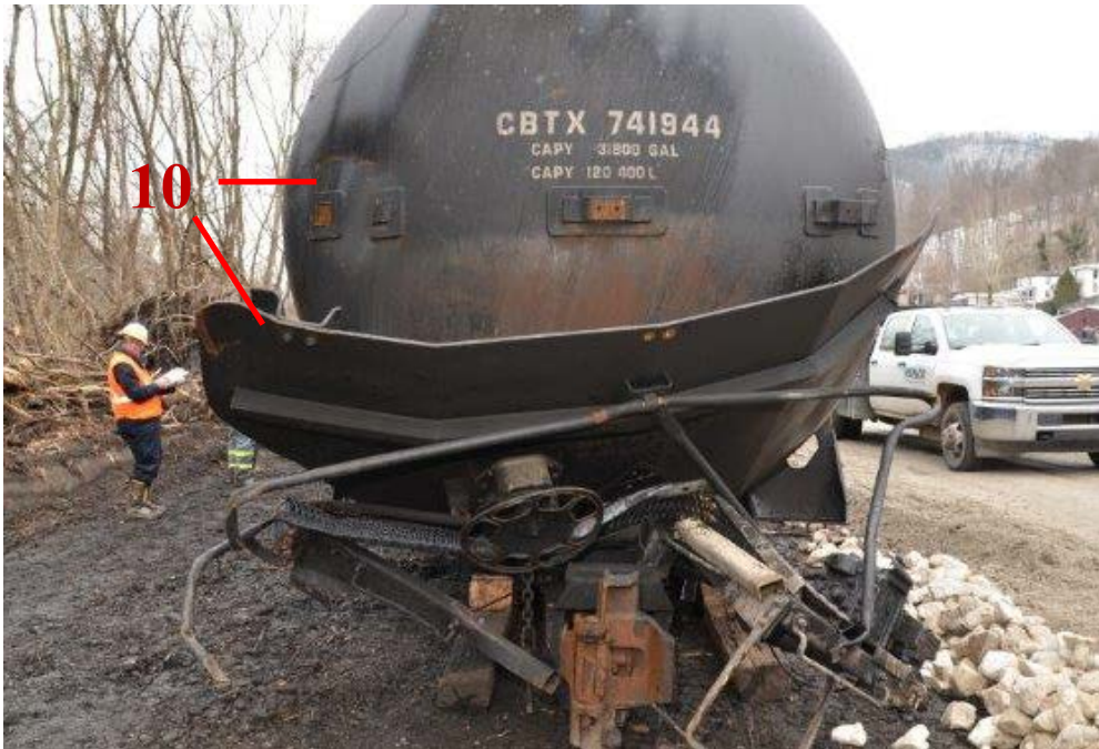
Figure 43: B-end head shield separation.
