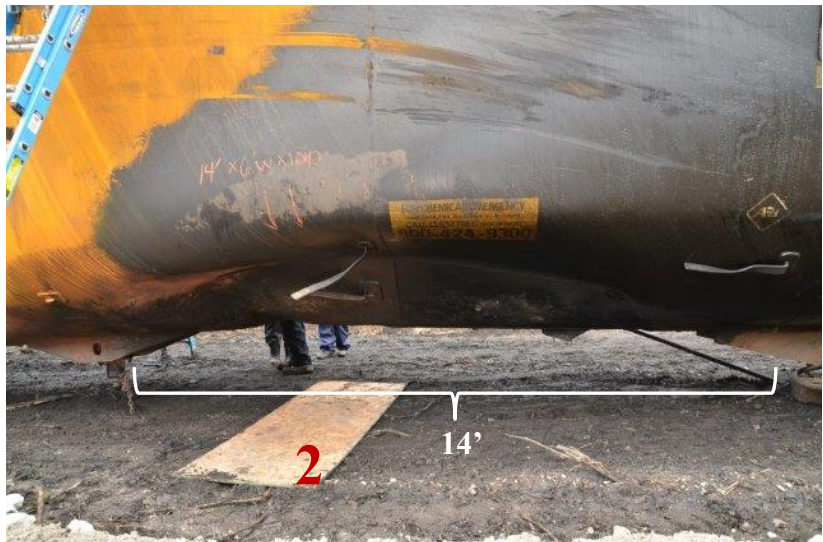
Figure 53: Dent and gouge in bottom left of tank car, B-end side of BOV.
