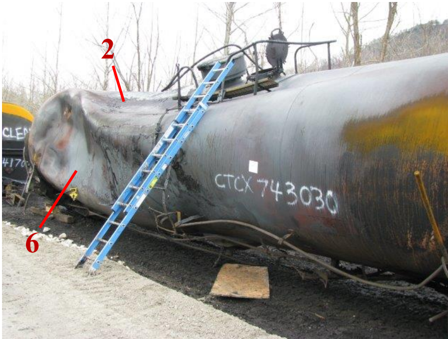
Figure 37: Left side shell compression and top flattening.
