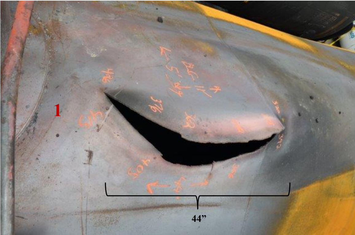
Figure 61: Close up of thermal tear to tank car CBTX741651.
