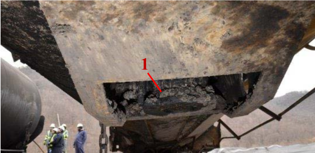
Figure 8: GATX 286241 bottom outlet valve, reclosed by response personnel.
