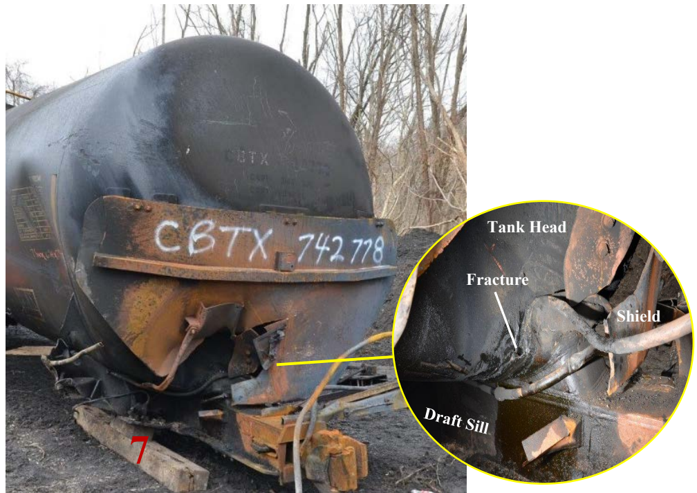
Figure 54: Punctured B-end head shield, and tank head fracture (inset image).
