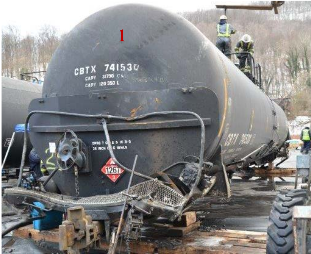
Figure 75: B-end head showing dent above head shield.
