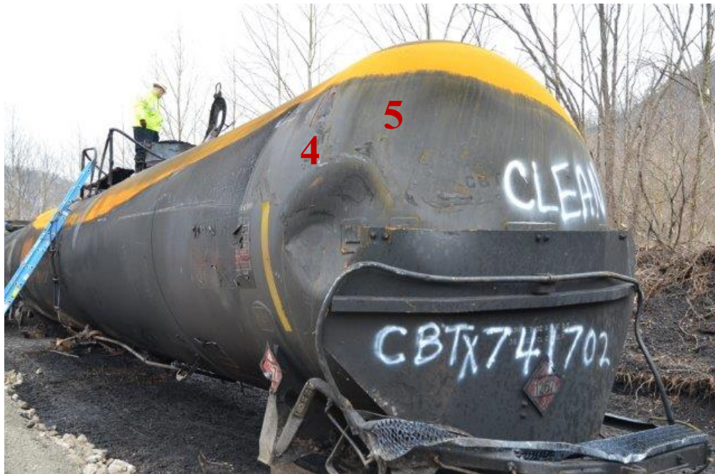
Figure 33: Dent to A-head not intercepted by half-height head shield.
