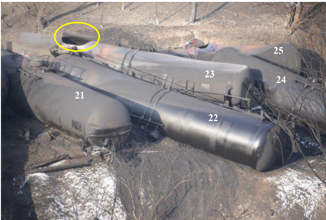
Figure 67: Resting position of CBTX 741946 highlighting the thermal tear (circle).
