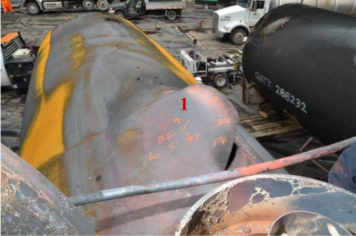
Figure 60: Thermal tear on top of tank car CBTX 741651.
