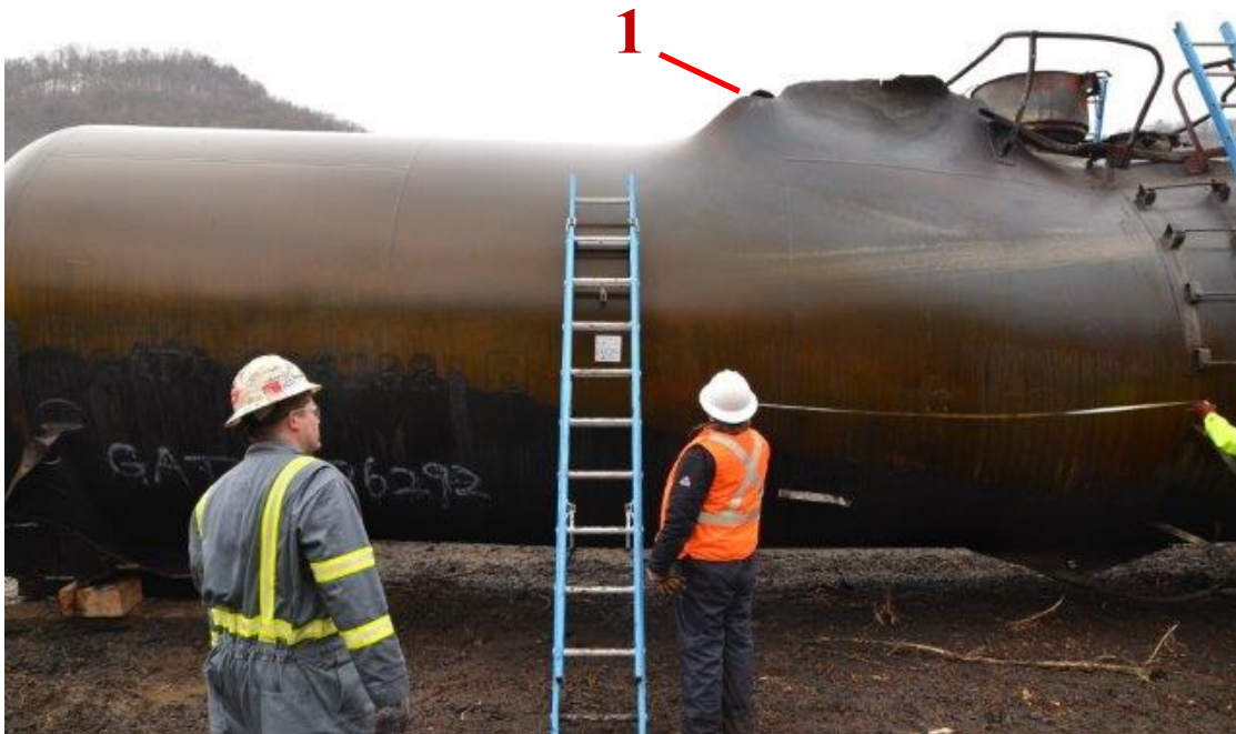
Figure 17: GATX 286292 thermal tear and shell bulging.
