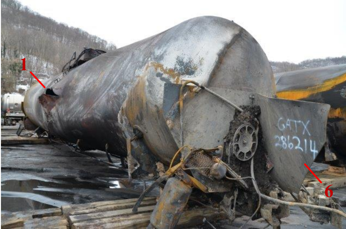
Figure 13: GATX 286214 thermal tear and head shield damage.
