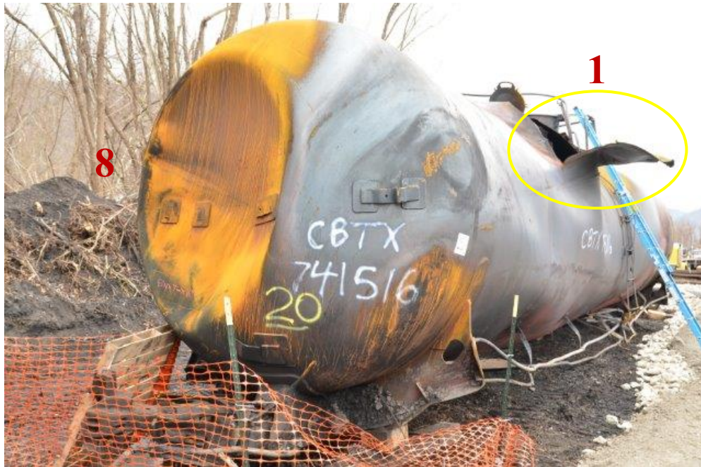
Figure 57: CBTX 741516 A-end head and thermal tear (circled).
