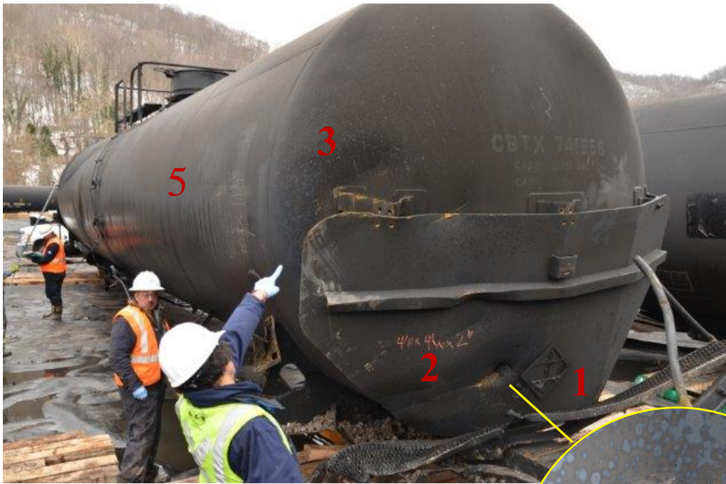
Figure 69: A-end head shield impact location and fracture.
