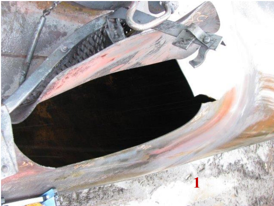
Figure 73: View of thermal tear from above.
