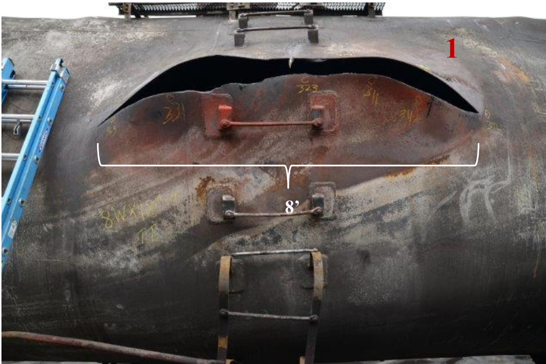
Figure 14: GATX 286214 thermal tear with material thickness measurements.
