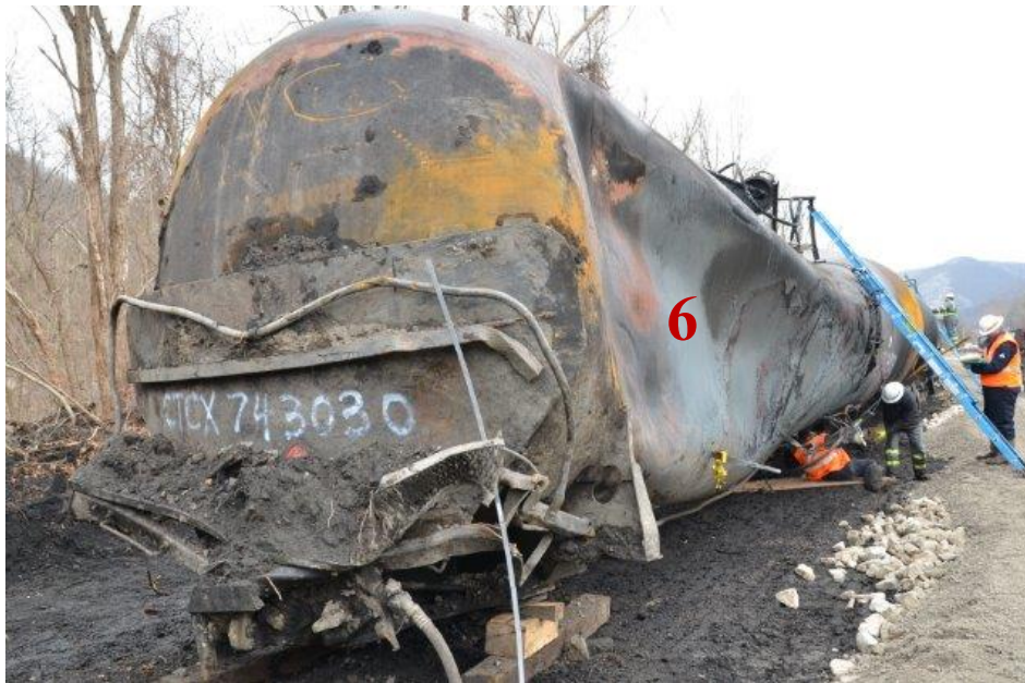
Figure 36: Left side shell compression, and A-end head.
