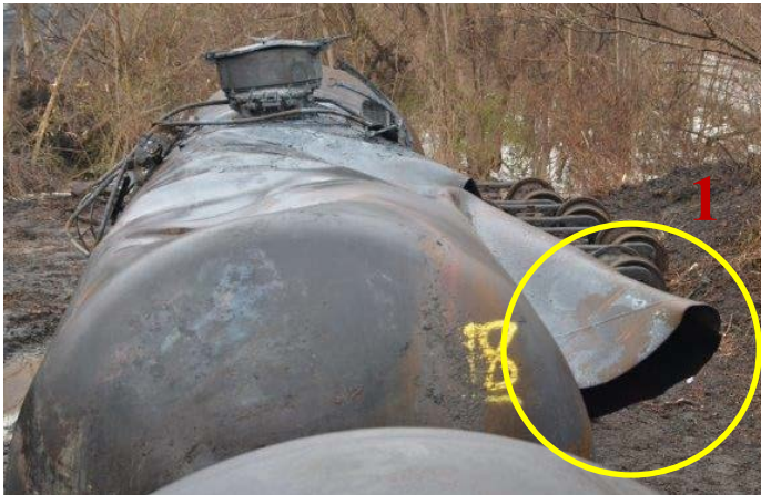
Figure 48: Flap of steel protruding from thermal tear (circled)
