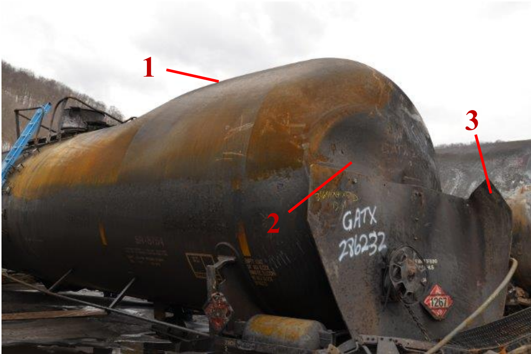
Figure 10: GATX 286232 B-end shell bulging and head damage.
