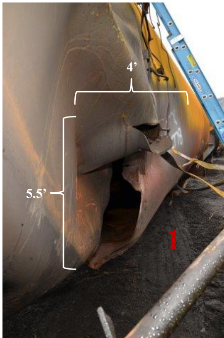
Figure 52: Puncture and fracture surfaces.
