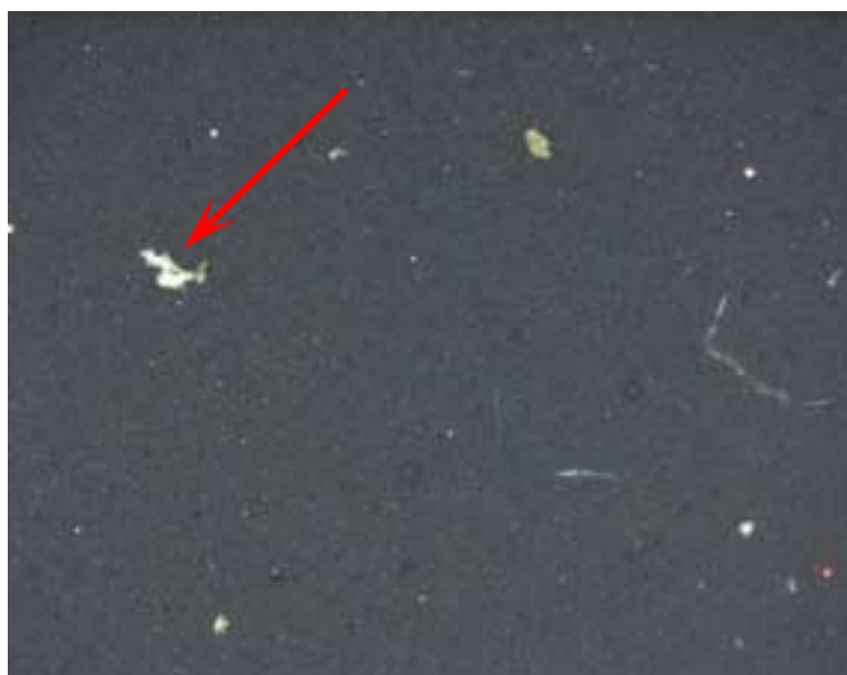
Figure A2. The filtrant from Sample 166, Hawaiian Airlines N709HA. The copper particle shown by the unlabeled arrow is consistent with Acme nut material.
