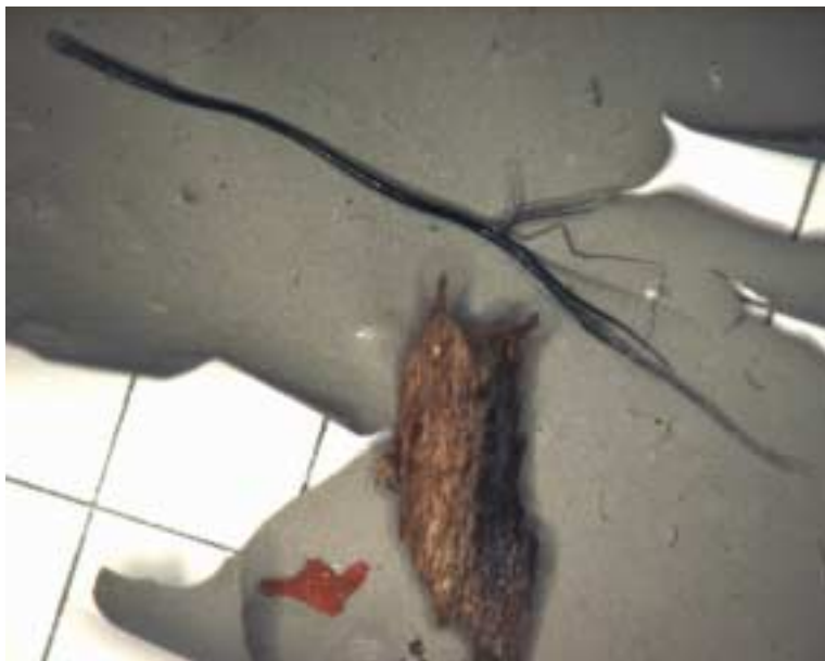
Figure A5. The filtrant from Sample 65, AirTran Airways N919VV. This filtrant included a red pliable particle, a brown fibrous particle that appears to be wood, and a black particle that appears similar to wire.
