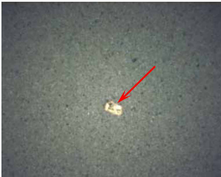
Figure A12. The filtrant from Sample 13, Alaska Airlines N981AS. The copper particle shown by the unlabeled arrow is consistent with Acme nut material.
