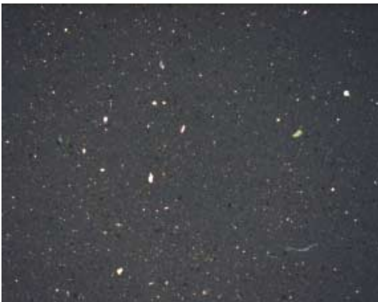
Figure A8. The filtrant from Sample 8, Delta Air Lines N907DA. The copper particles are consistent with Acme nut material.
