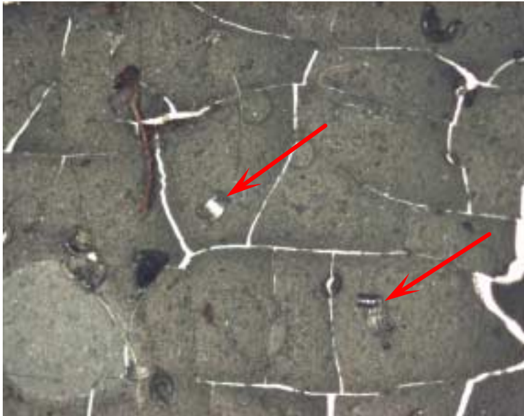
Figure A7. The filtrant from Sample 16, Delta Air Lines N904DA. The particles shown by the unlabeled arrows appear to be drill shavings and are consistent with an iron material.
