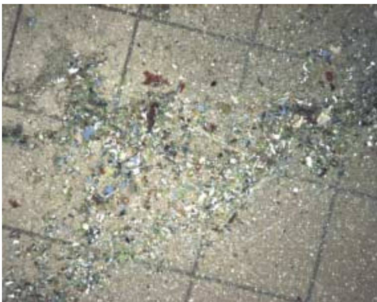
Figure A6. The filtrant from Sample 122, AirTran Airways N919VV. The small particles resemble paint chips, plastic chips, glass particles, and metallic shavings.
