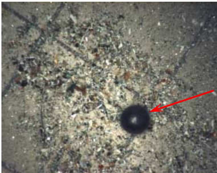
Figure A1. The filtrant from Sample 159, Hawaiian Airlines N662HA. The small particles resemble paint chips, plastic chips, glass particles, sand particles, and metallic shavings. The large dark bead shown by the unlabeled arrow is consistent with an iron material.
