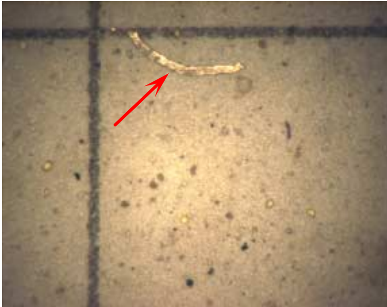
Figure A15. The filtrant from Sample 126, China Northern Airlines part number DGA0024. The particle shown by the unlabeled arrow is consistent with Acme nut material.
