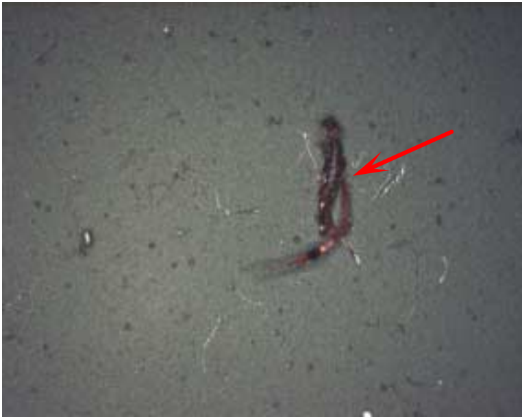
Figure A9. The filtrant from Sample 69, Reliant Airlines N915R. The red particle shown by the unlabeled arrow appears similar to a glass material.
