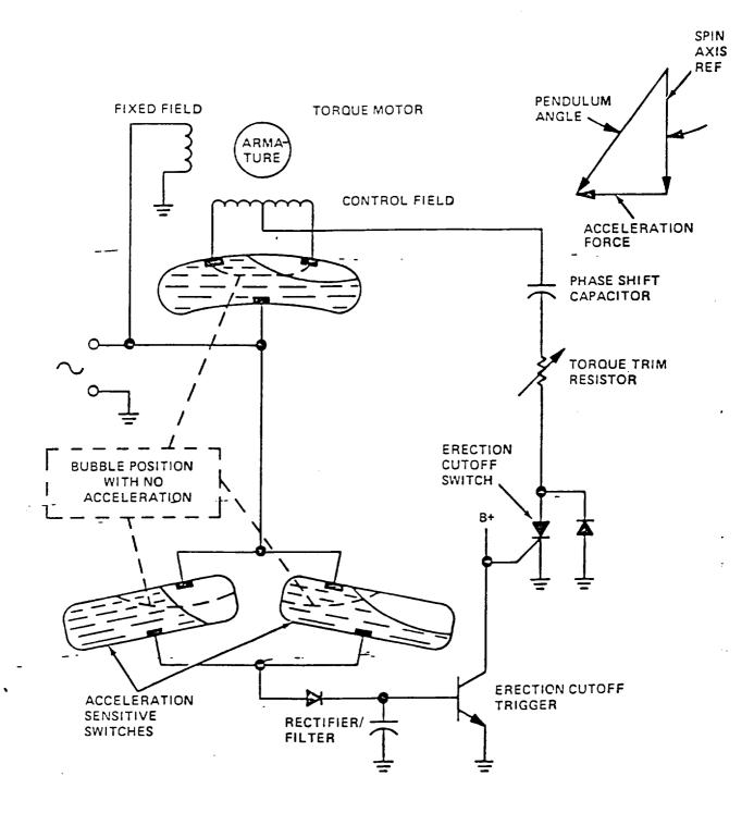
Vertical Gyro Erection Circuit with Erection Cutoff during Acceleration Figure 5
