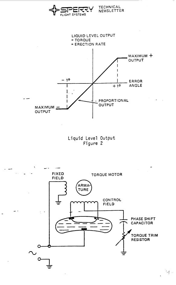
Vertical Gyro Erection Circuit Figure 3
