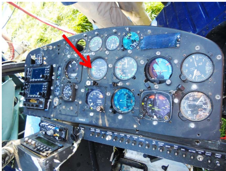
Photo 6: N352LN pilot instrument panel (post-accident). Location of the NF/NR gauge indicated by the red arrow.
