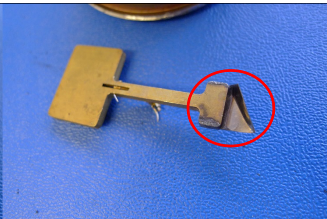
Photo 26- balance plate assy, torn, 1 of 2
