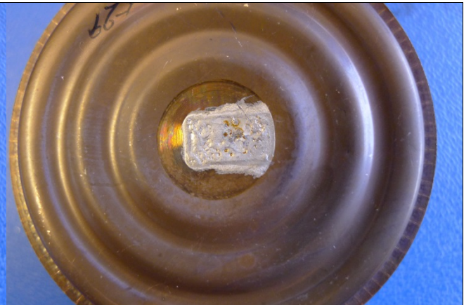
Photo 33- diaphragm solder joint side 2
