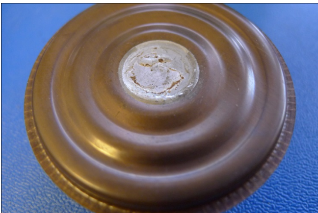
Photo 25- diaphragm assy, detached
