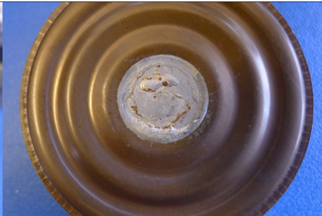
Photo 32- diaphragm solder joint side 1
