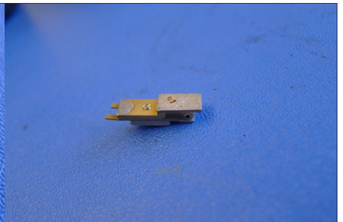
Photo 36- bimetal assy detached from diaph assy 2 of 2
