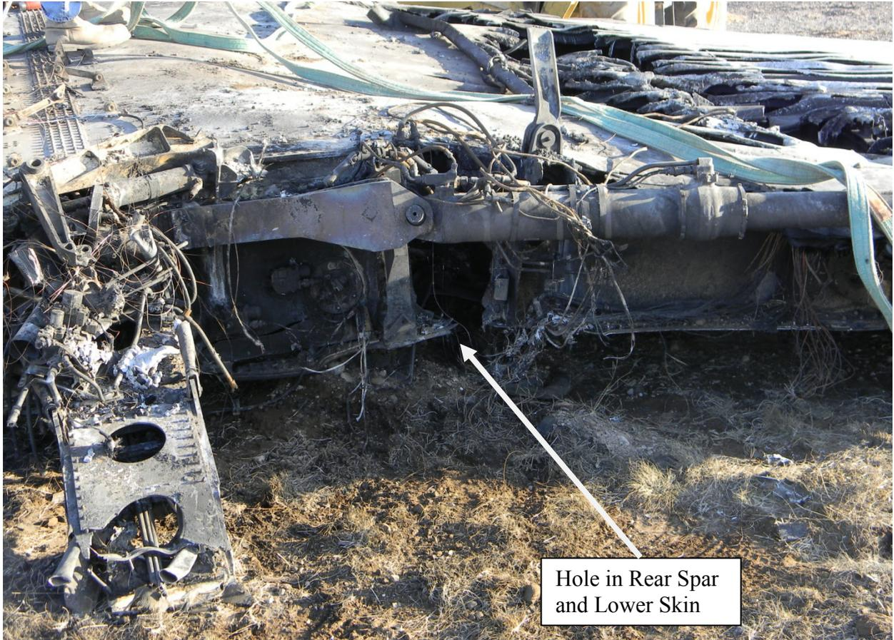
Figure 44 Center Wing Box Aft Spar Damage
