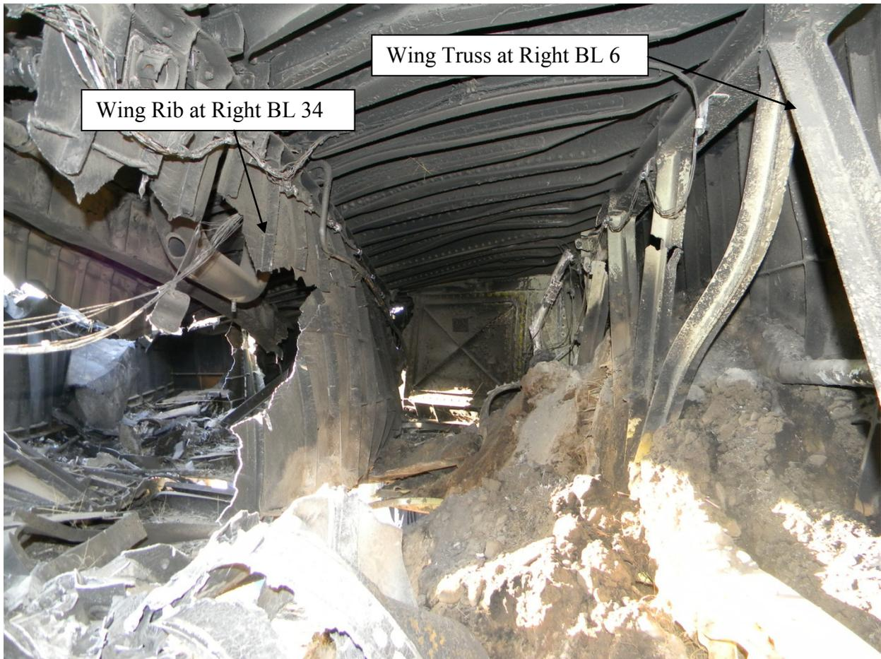
Figure 43 Center Wing Box Internal View looking Aft
