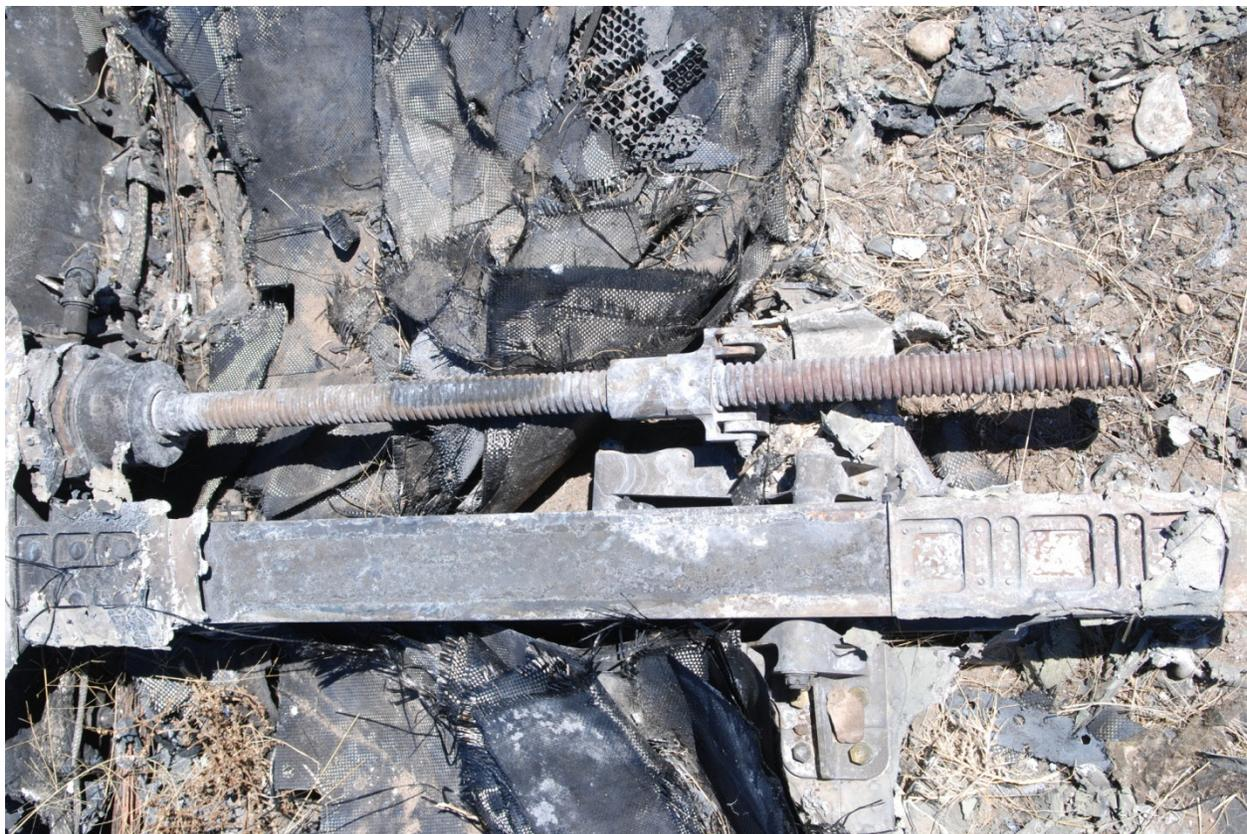
Figure 22 Flap Track B and Jackscrew
