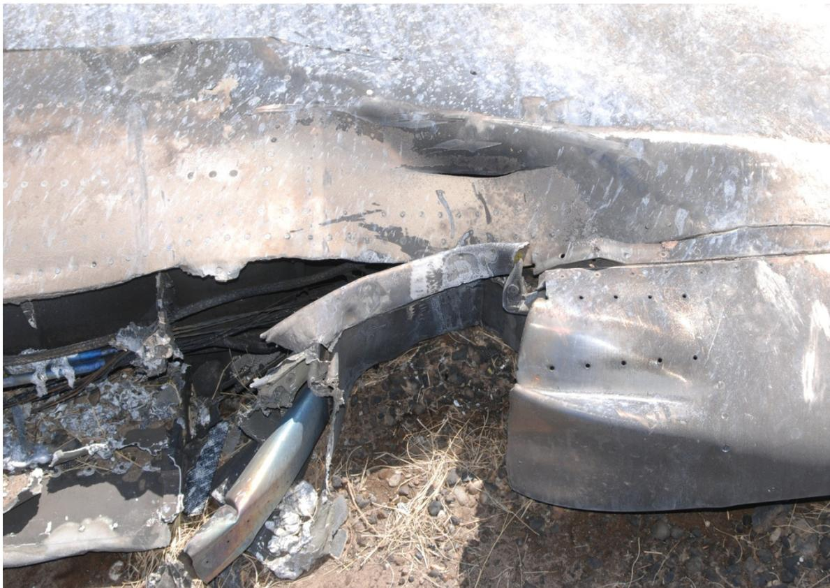
Figure 20 Left Wing Impact Damage
