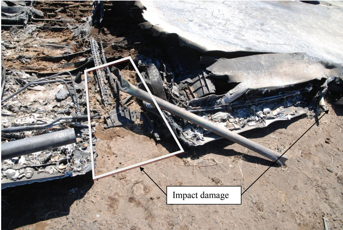
Figure 19 Left Wing Impact damage
