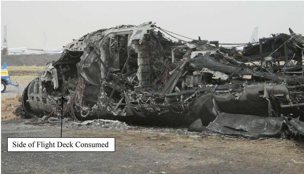
Figure 62 Left Fuselage Forward and Forward Mid Sections
