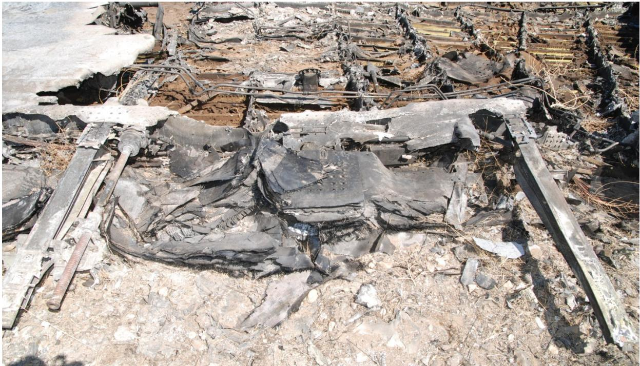
**Figure 28 Left Inboard Spoiler**
