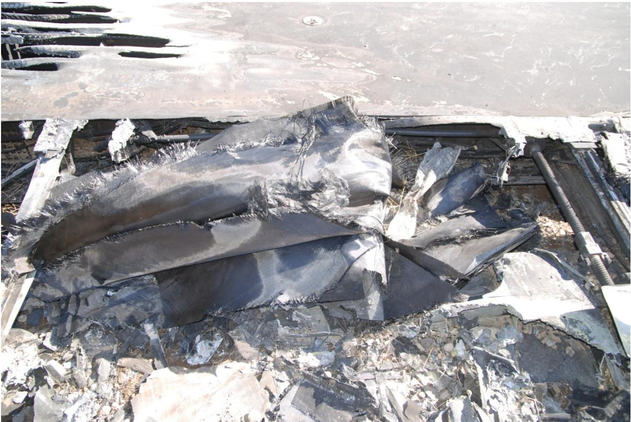
**Figure 36 Right Inboard Spoiler**
