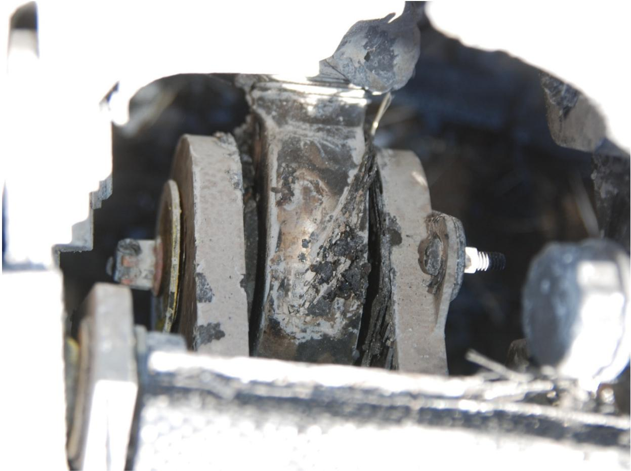
**Figure 27 Left Middle Spoiler Attachment Fitting**
