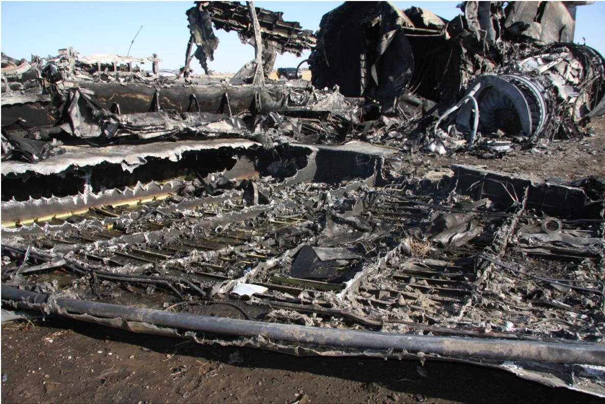
Figure 17 Left Wing Inboard Leading Edge
