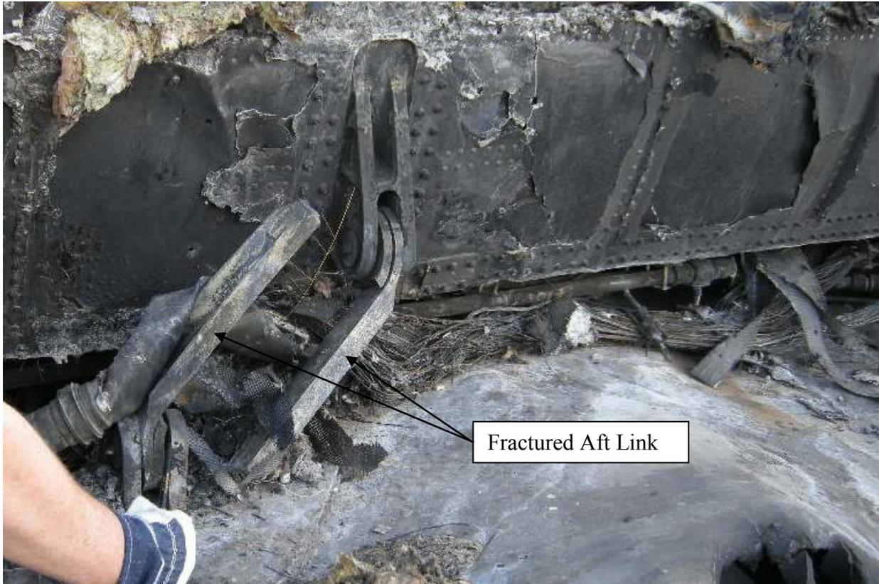
Figure 60 Right Aft Wing to Fuselage Link
