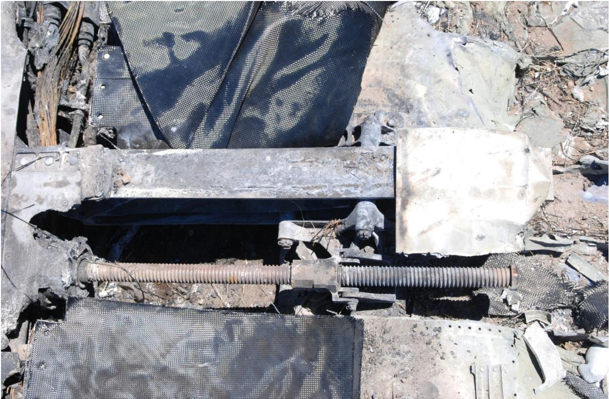
Figure 23 Flap Track C and Jackscrew
