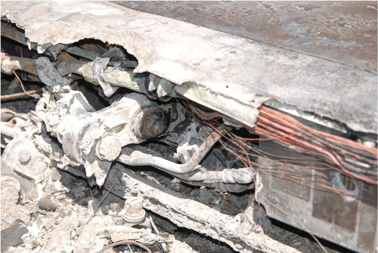
Figure 25 Left Outboard Spoiler Actuator Fittings
