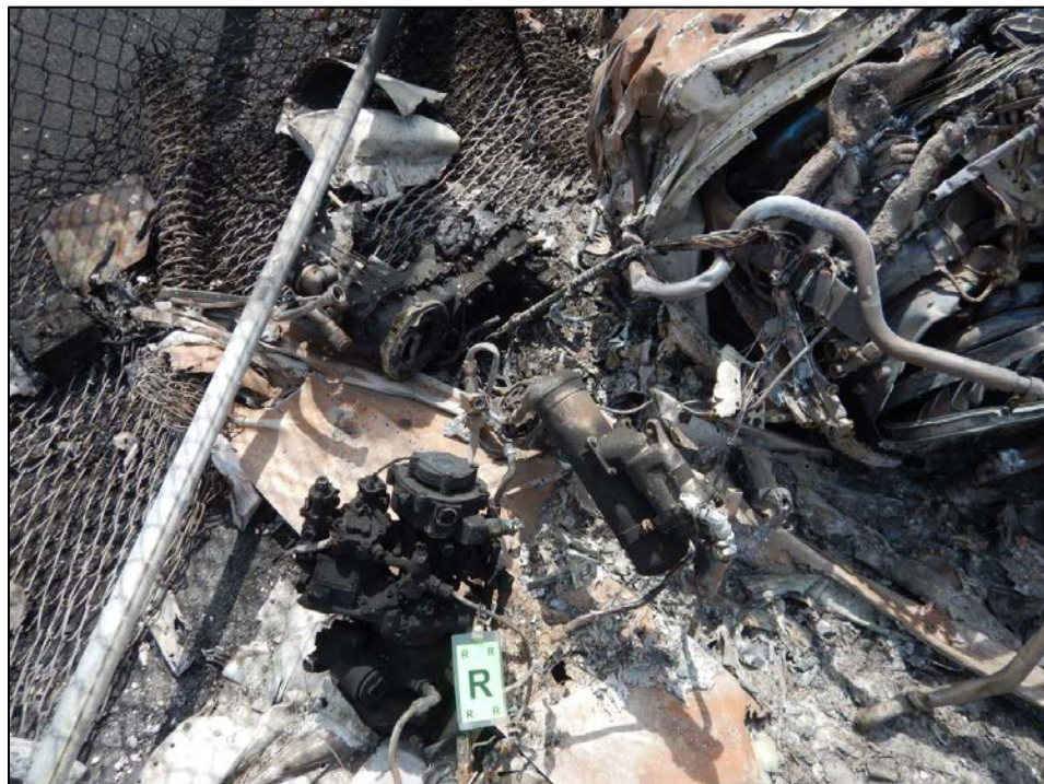
Figure 32: Right engine accessory gearbox and line replaceable unit
