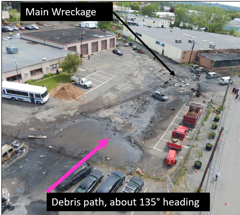
Figure 3: Overhead view looking southeast at the debris path and main wreckage
