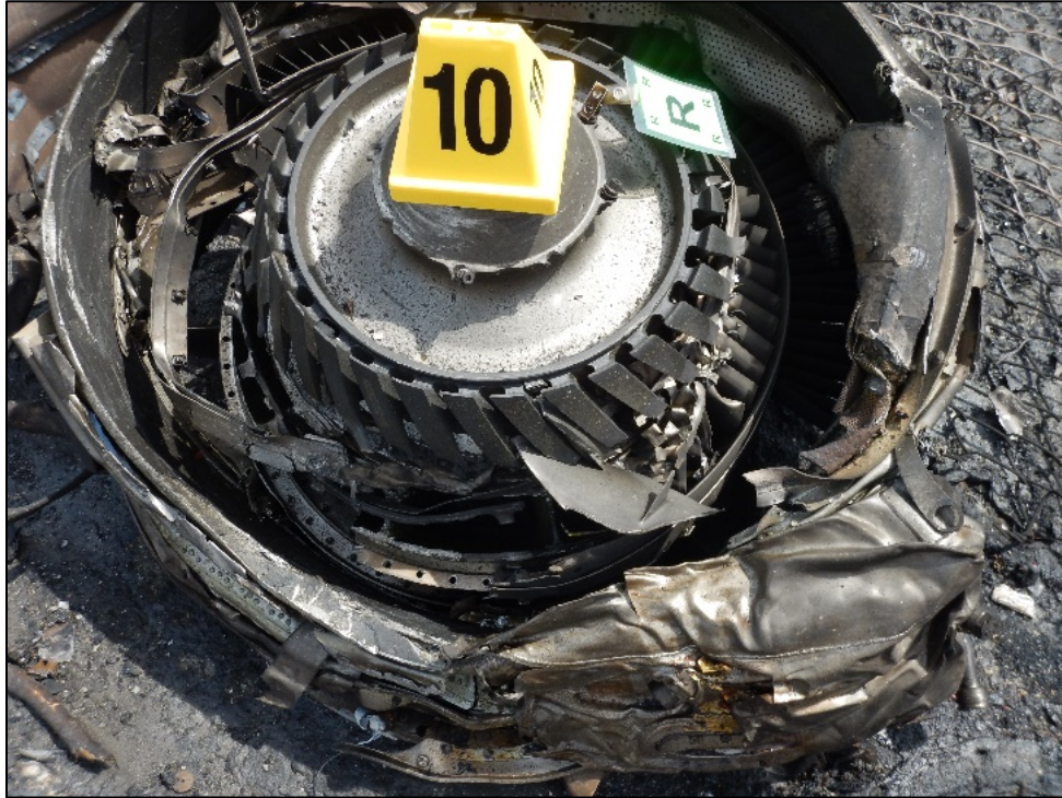
Figure 29: Right engine fan assembly
