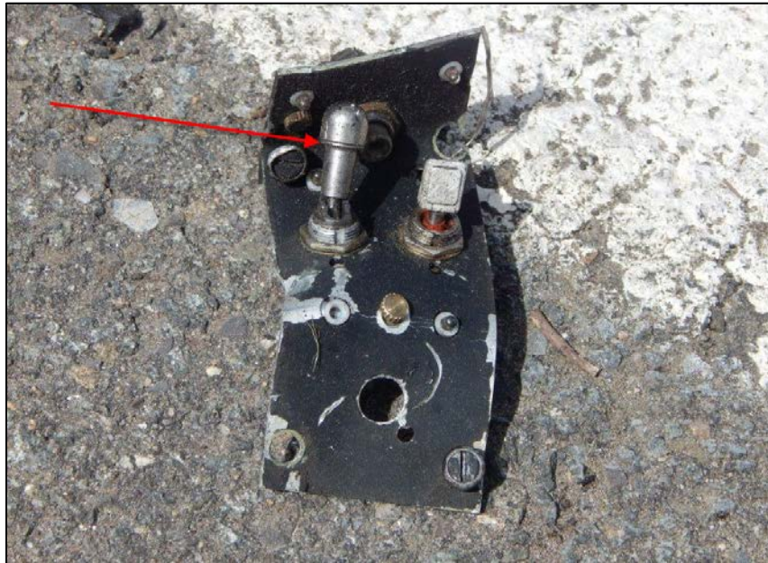
Figure 22: Pitch trim panel switch
