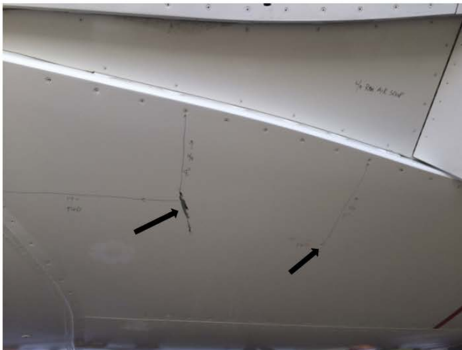
Figure 18 - Damage Found on Left Hand Forward Wing to Body Fairing.
