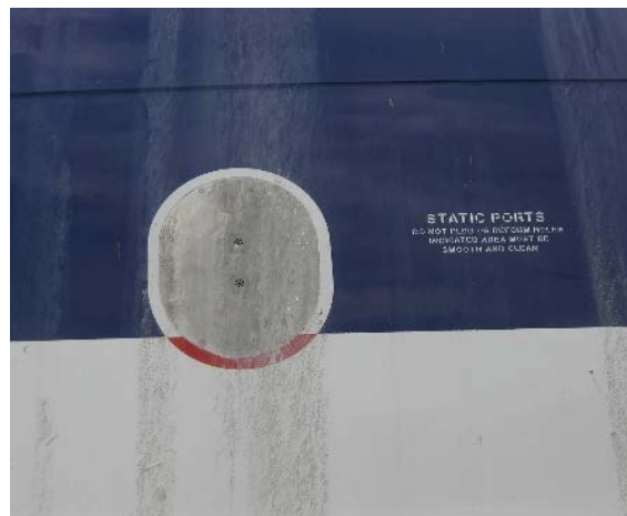
Figure 6 - Example of EMAS debris on Static Port
