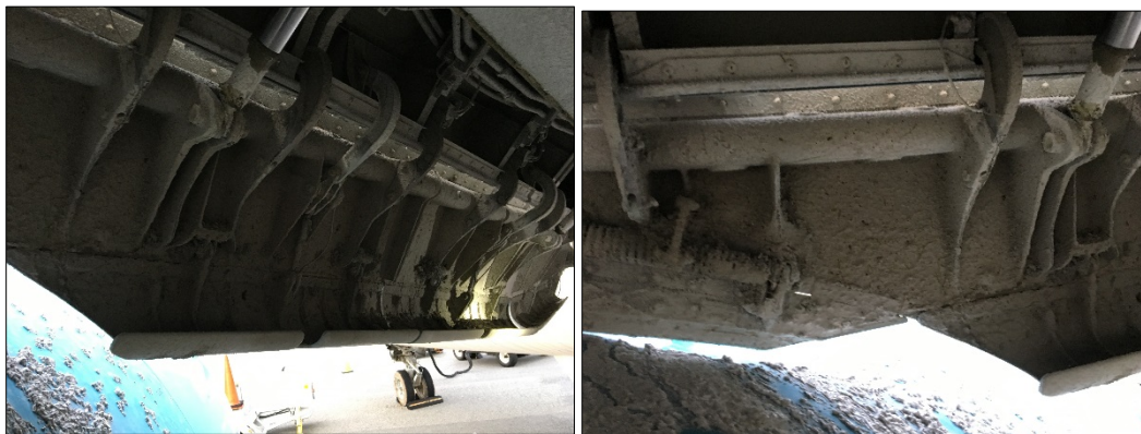
Figure 20 A/B - EMAS debris on the underside and interior of wing leading edge.
