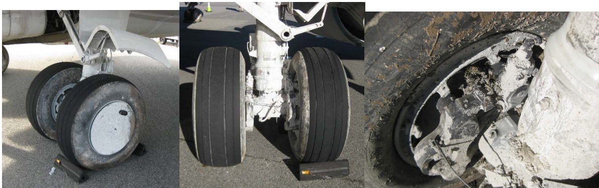
Figure 11A, B, and C - Right Main Landing Gear and EMAS Debris
