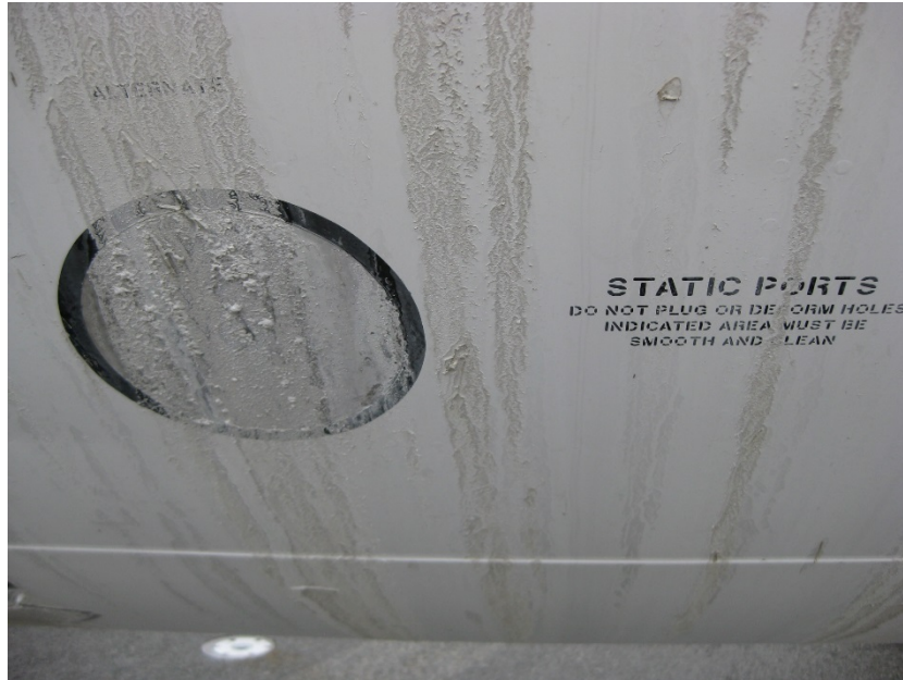
Figure 7 - Example of EMAS debris on Static Port.
