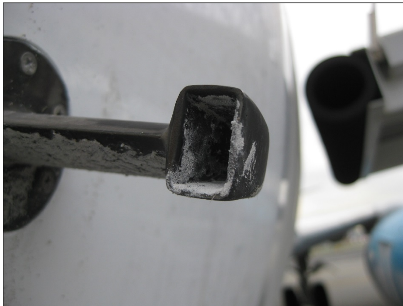
Figure 8 - Example of EMAS debris on External Port.
