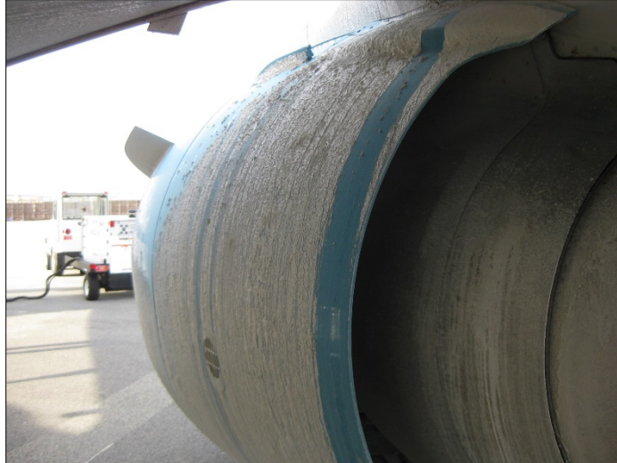
Figure 26 – Inboard (left) side of Engine 2 with EMAS debris
