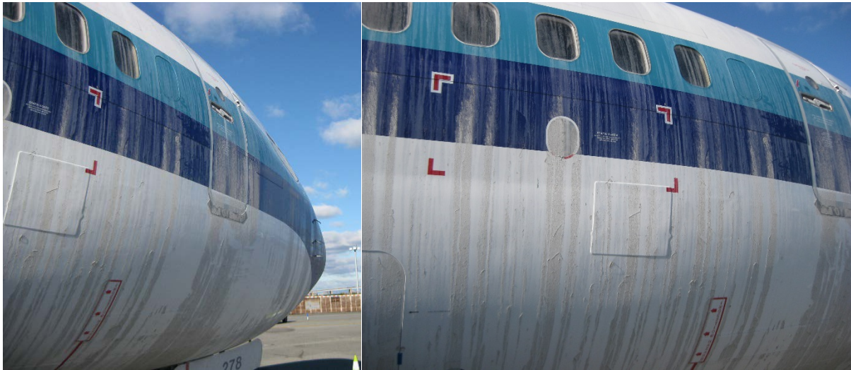
Figure 16A/B - Dried EMAS Material and Grass on Right Hand Side of Fuselage
