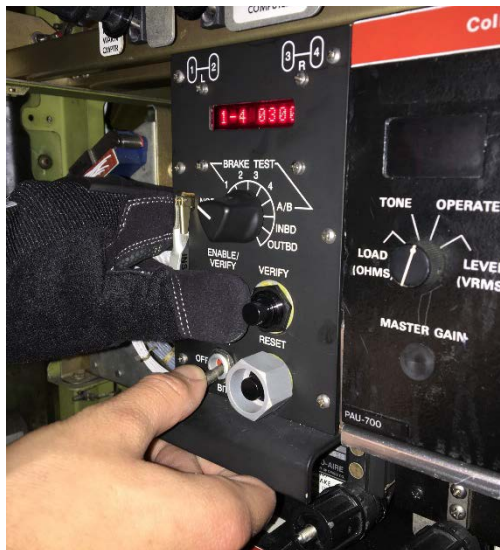
Figure 15 - Testing the Antiskid/Autobrake Control Unit (AACU) Using the BITE Function. A Software Revision Display Message is shown on the AACU Display.
