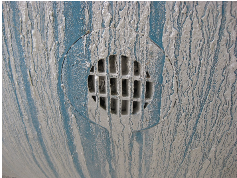
Figure 27 - Port with EMAS debris on inboard Number 2 (right) Engine.
