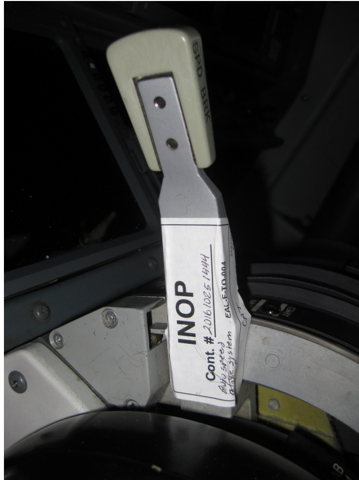
Figure 2 - Close Up of the Speedbrake Handle and INOP Sticker.
