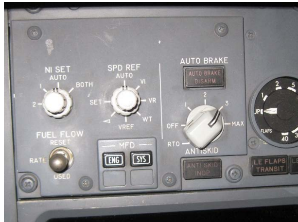
Figure 5 - Autobrake Control Panel with Position 3 Selected
