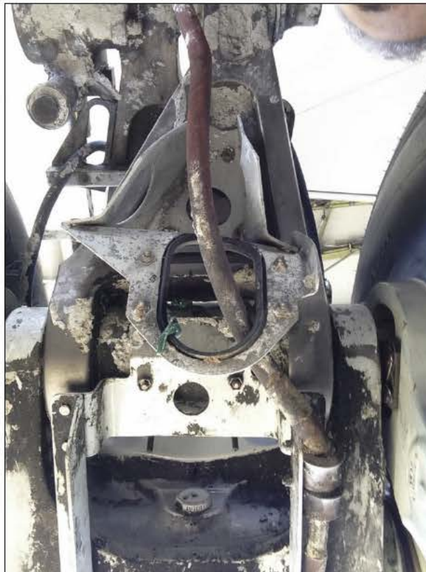
Figure 13- Damage to underside of Right Main Landing Gear Lower Wire Bundle Bracket.
