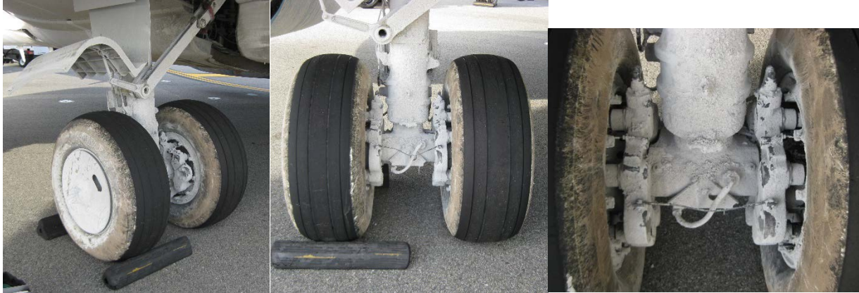
Figure 10A, B, and C - Left Main Landing Gear and EMAS Debris
