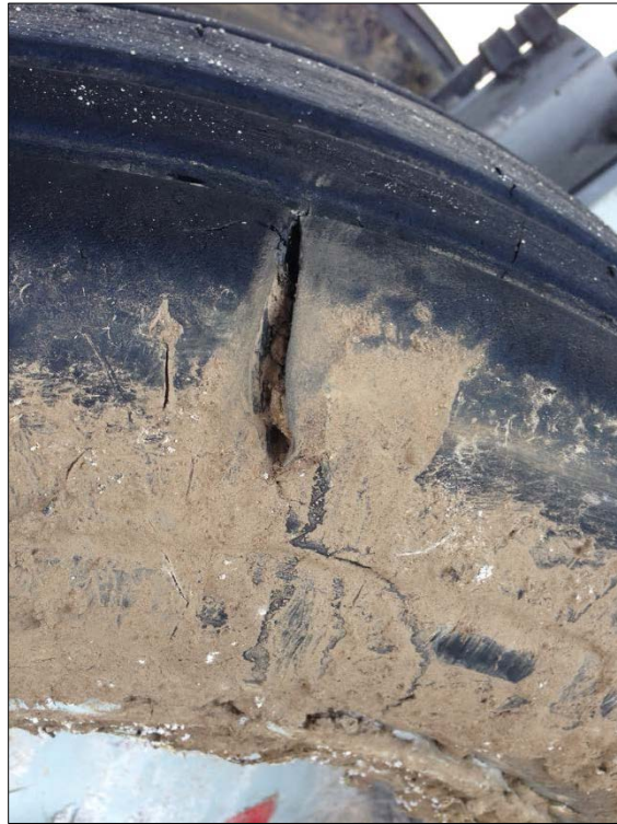
Figure 14 - Cut on the outboard sidewall of Tire Number 1.
