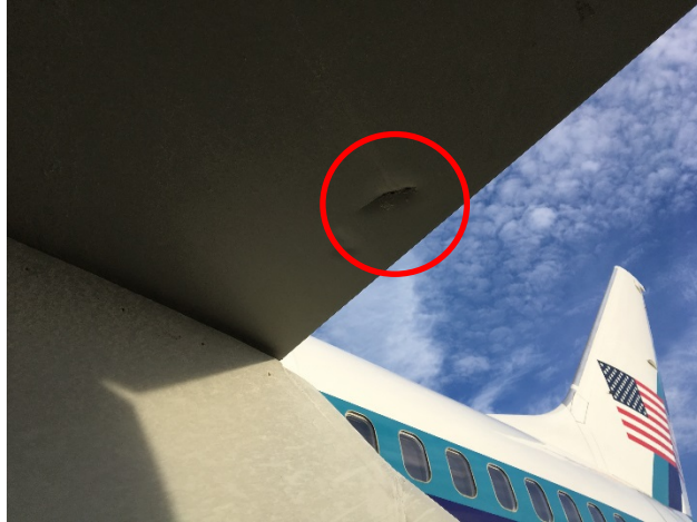
Figure 21 - Impact Damage Noted on Underside of Number 3 Trailing Edge Flap Surface
