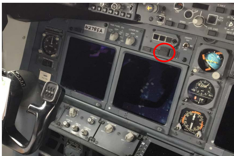
Figure 4 - The "SPEEDBRAKE ARMED" and "SPEEDBRAKE DO NOT ARM" lights on the P1 Panel (circled).
