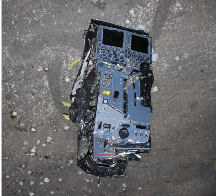
Figure 3 - Center Pedestal, including throttle quadrant, at hangar, prior to shipment to manufacturer.
