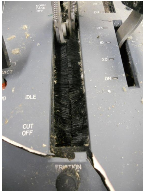
Figure 4 - FOD brushes near the Idle/Cut Off area, before the brushes were cut.
