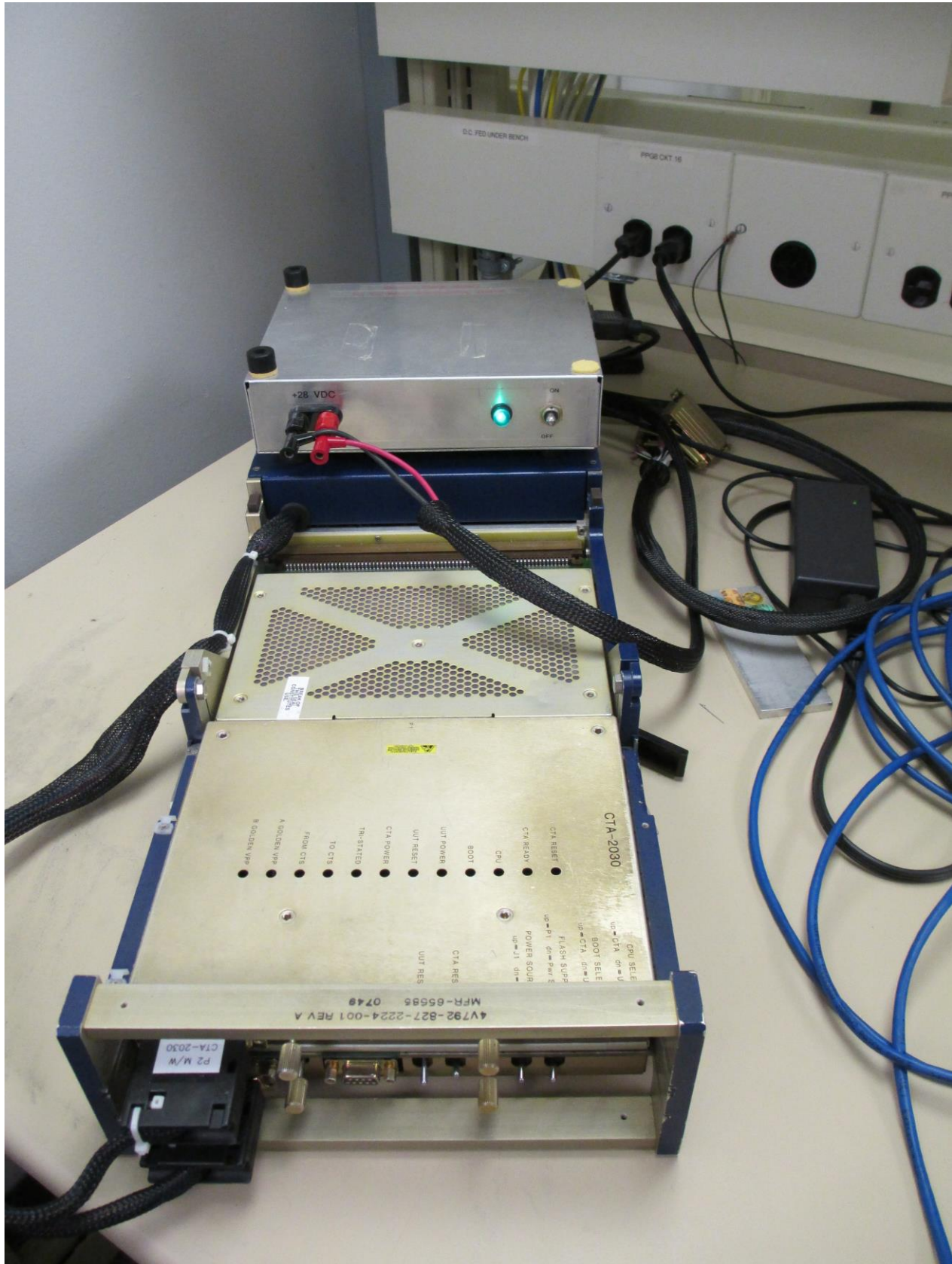
Figure 2: FMC-3000 in the mount used for extracting NVM
