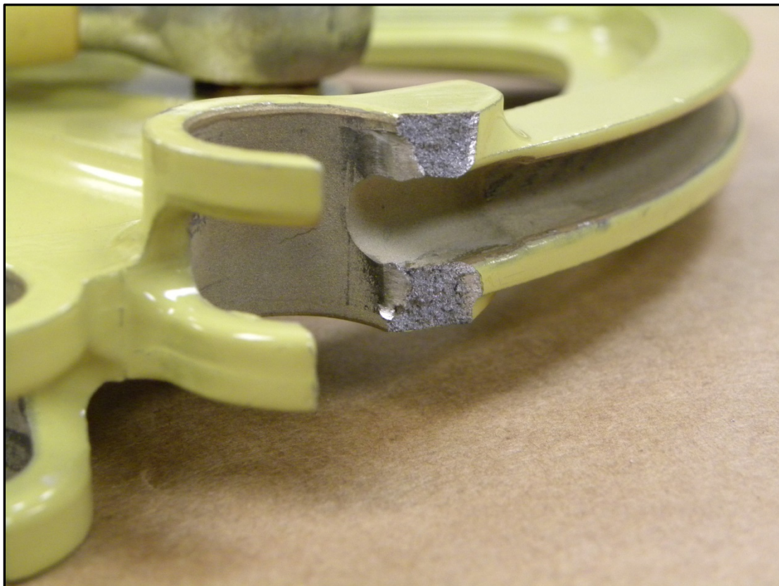
Figure 5: Cable Link Failure on -16 Bellcrank
