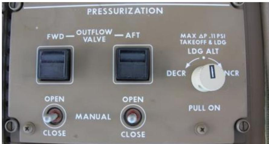
Figure 11 - Pressurization Panel
