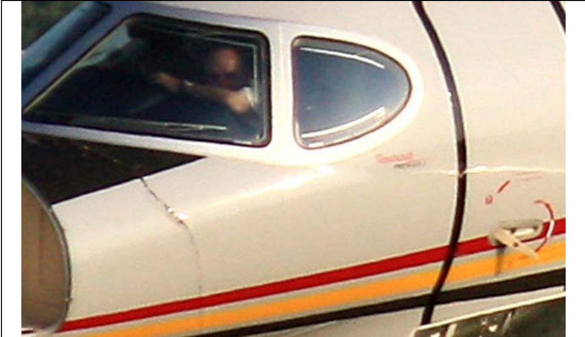
Figure 10. Cropped section of an attached photo that shows the airplane colliding with the drainage ditch, showing the captain's arm stretched forward of the shoulder. The person in the first officer seat is not similarly visible. Also shown are displacement of the main cockpit door handle and a fuselage fracture near the forward pressure bulkhead.
