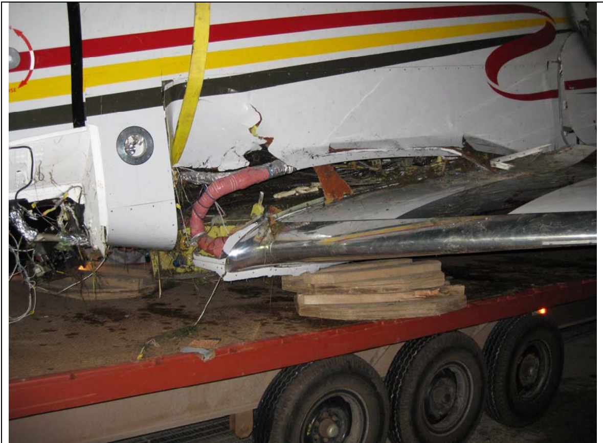
Figure 6. Separated leading edge of left wing root beneath fuselage. (Nose is to the left)
