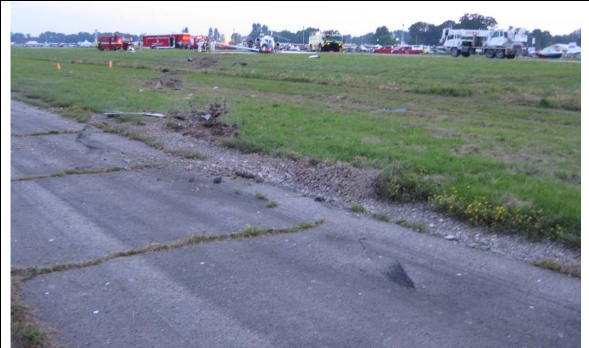
Figure 1. View toward the airplane from left and right main landing gear tire marks. The first point of ground contact by the wingtip was at the right edge of the photo and is not visible in this view.
