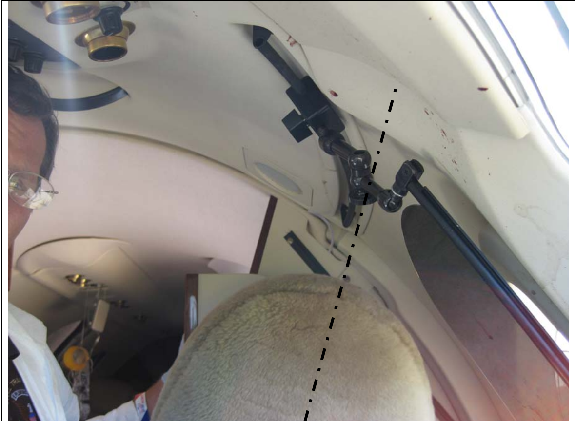
Figure 15. Sun visor mounting assembly and adjustment knob, as viewed aft and from above the centerline of the control yoke. The photo is slightly rotated and the dashed line has been added to provide vertical orientation, as copied from the door frame.
