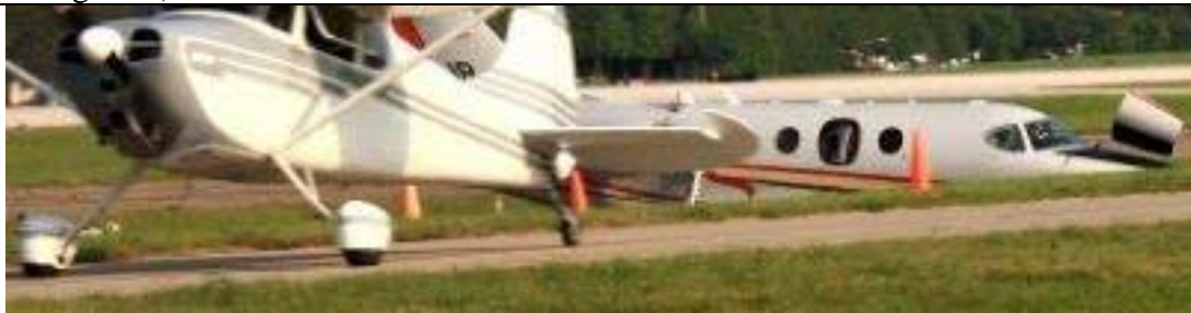
Figure 8. Cropped section of photo shows the overwing escape hatch opening during the impact sequence.
