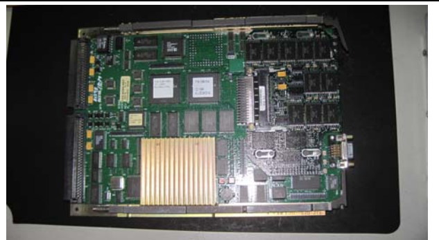
Photo 2: View of the internal PCB that contains the flash memory chips.
