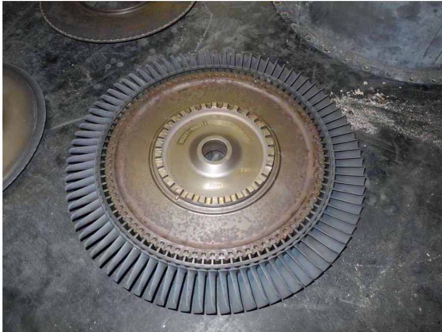
Figure 17. The first stage turbine rotor from the No. 2 engine.
