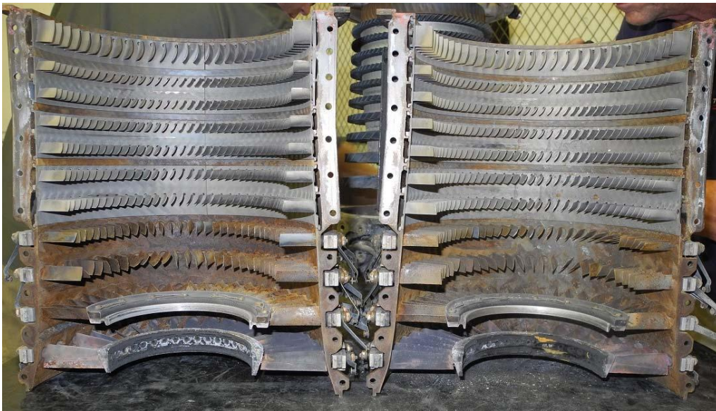
Figure 19. Compressor case halves from the No. 2 engine.
