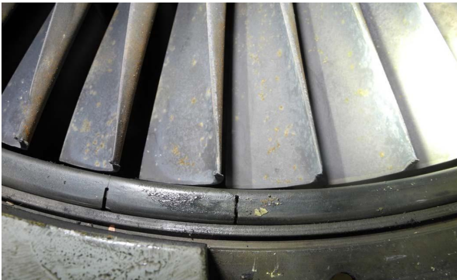
Figure 21. Damage observed on the leading edge tip ends of the power turbine blades from the No. 2 engine.
