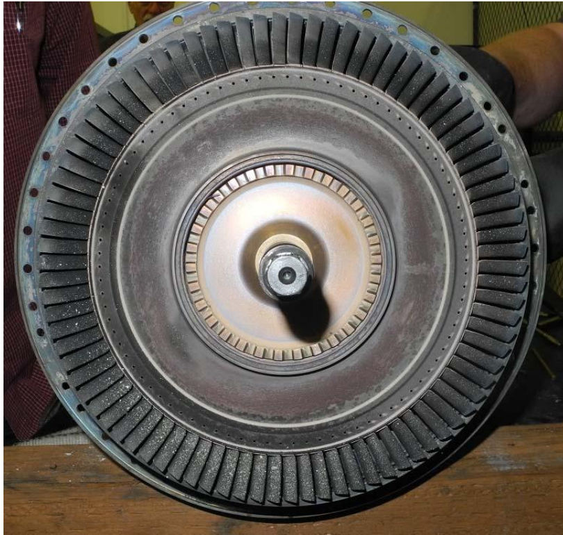
Figure 12. The first stage turbine rotor from the No. 1 engine.
