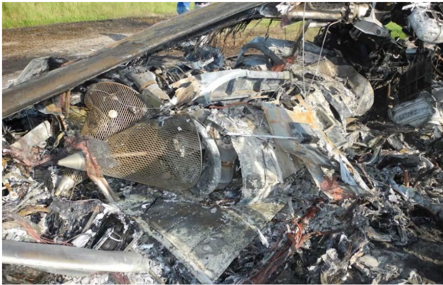
Figure 2. The engines and conical inlet screens at the accident site (No. 2 engine partially viewable).
