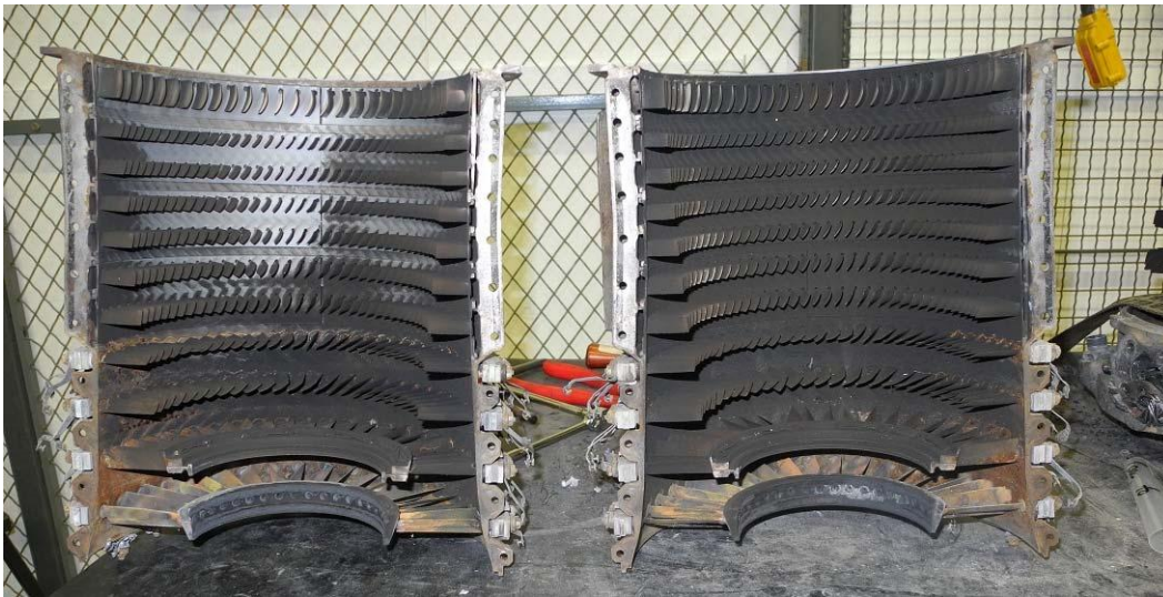
Figure 14. Compressor case halves from the No. 1 engine.
