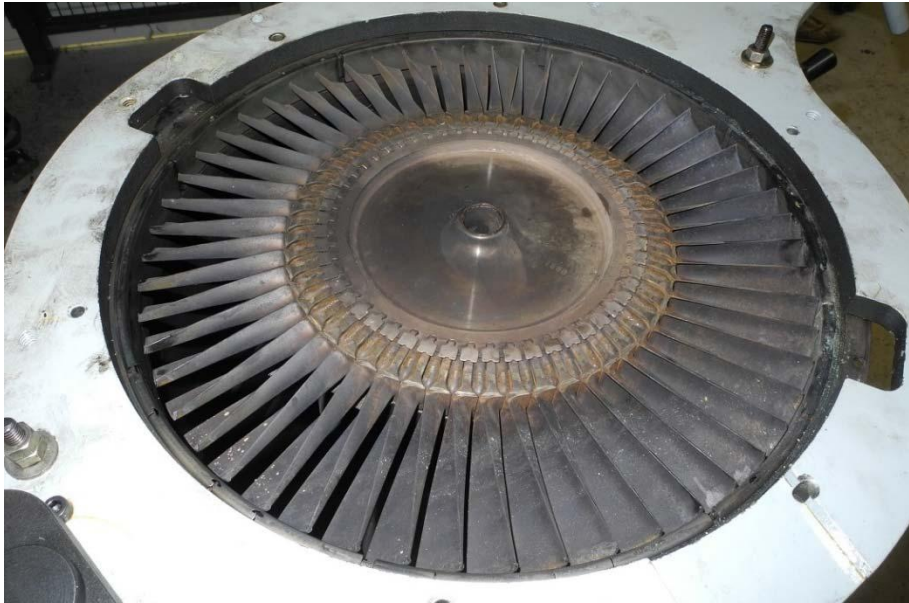
Figure 20. The power turbine rotor from the No. 2 engine.
