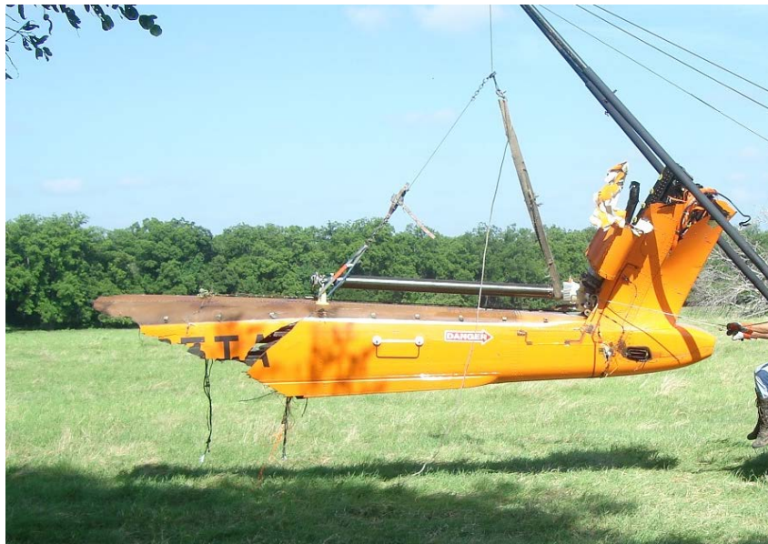
Figure 5. Angled cut line at the forward end of the aft section of the tail boom. (photo courtesy of GE Aviation)
