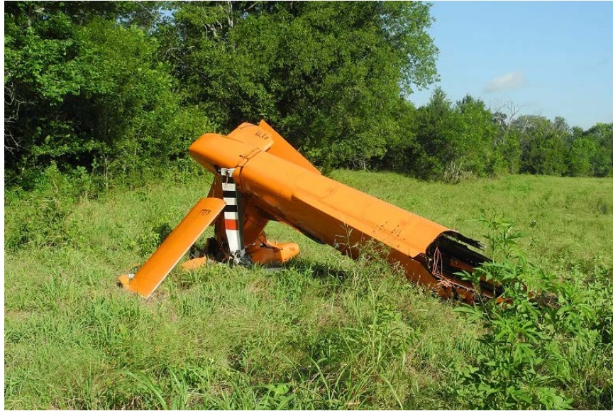
Figure 4. The aft portion of the tail boom.
