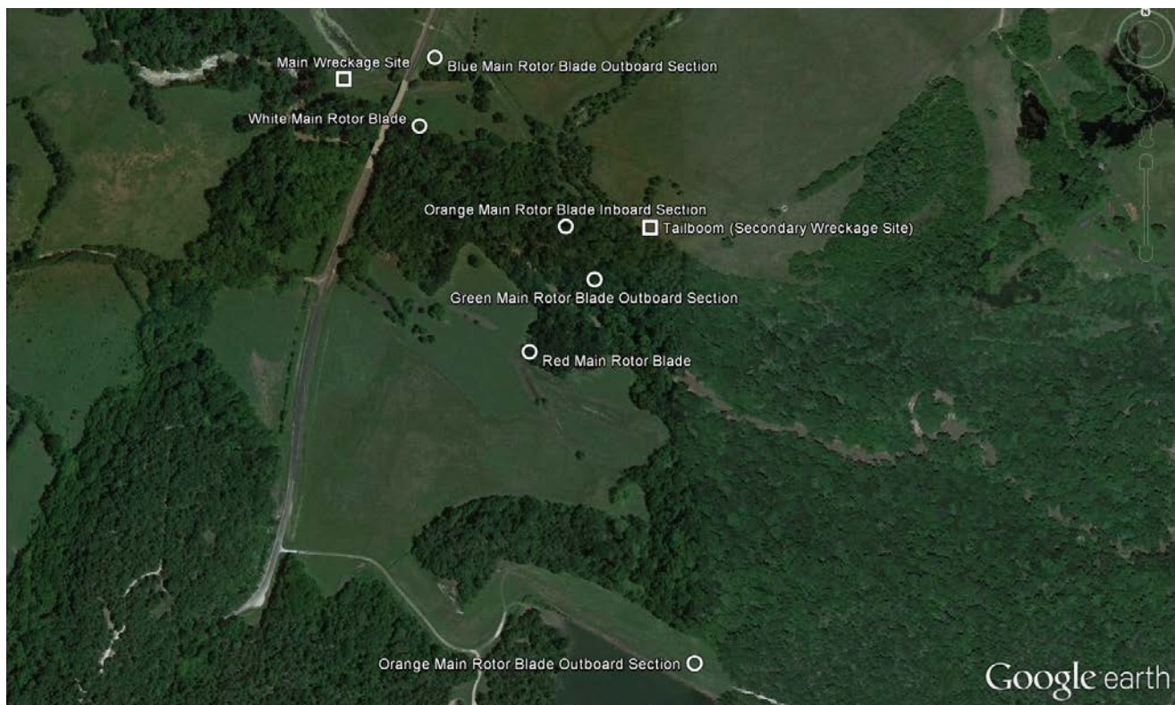
Figure 3. The location of main rotor blade sections.
