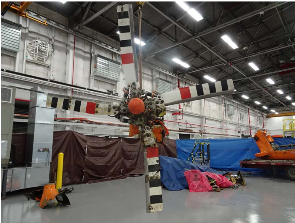
Figure 8. The recovered tail rotor head with all four tail rotor blades attached. (Photo courtesy of Bell Helicopter)
