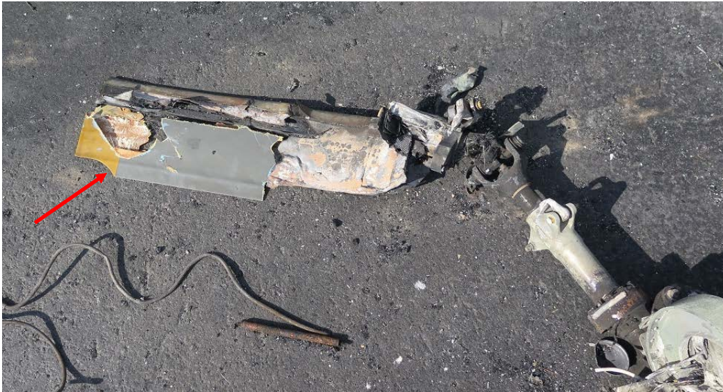
Photo 4. The 'red' tail rotor blade afterbody laid next to the 'red' tail rotor blade. A red arrow points to the afterbody. (Photo courtesy of AHI)
