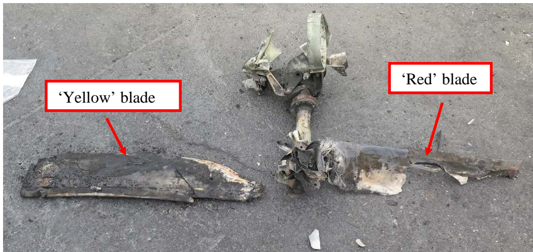
Photo 2. Tail gearbox laid out with both tail rotor blades. (Photo courtesy of AHI)
