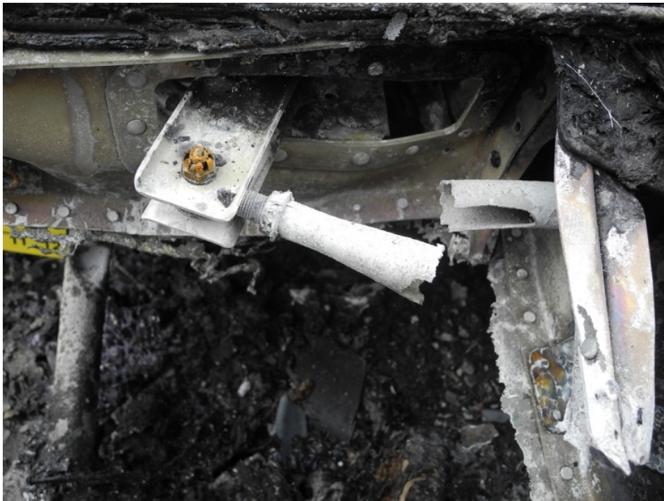
Photo 5. Fractured and heat distressed push-pull tube for the right pedal.
