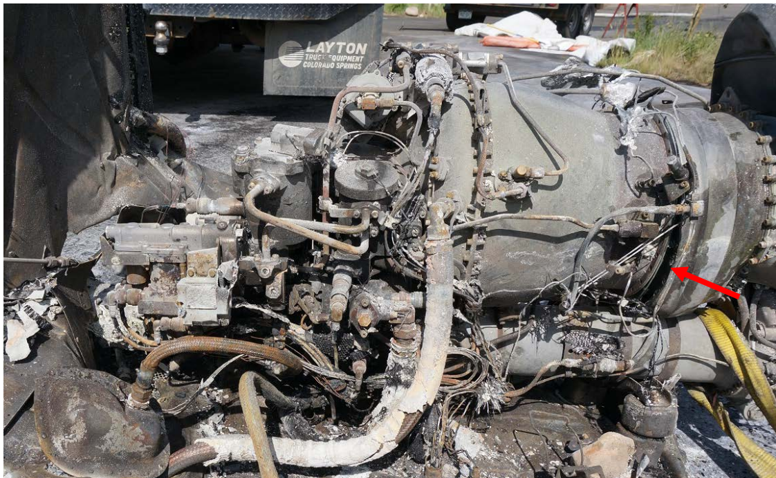
Photo 10. The left side of the engine after extraction from the main wreckage. The red arrow points to the partially separated flanged connection between the free turbine case and the gas generator case. (Photo courtesy of AMC)
