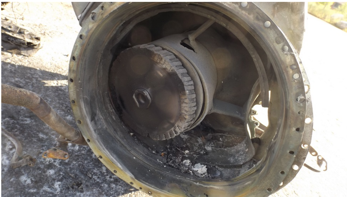
Photo 12. Free turbine rotor exhibiting evidence of blade shedding (module was removed from engine). (Photo courtesy of Turbomeca)
