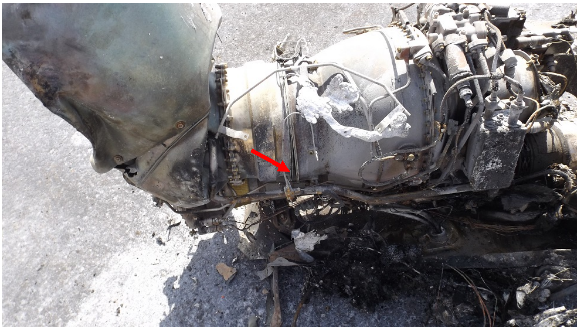
Photo 9. The right side of the engine after extraction from the main wreckage. The exhaust duct was observed to be deformed upward. The red arrow points to the partially separated flanged connection between the free turbine case and the gas generator case. (Photo courtesy of Turbomeca)
