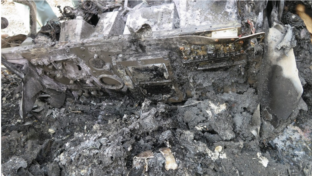
Photo 7. Cockpit instruments exhibiting heat distress.
