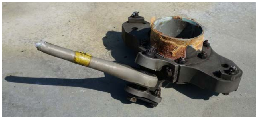
Photo 3. The recovered 'yellow' pitch change link attached to the blade horn and boss weights. (Photo courtesy of AMC)
