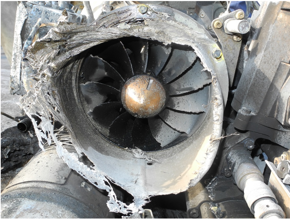
Photo 11. Axial compressor blade leading edges exhibiting evidence of hard body impact damage.
