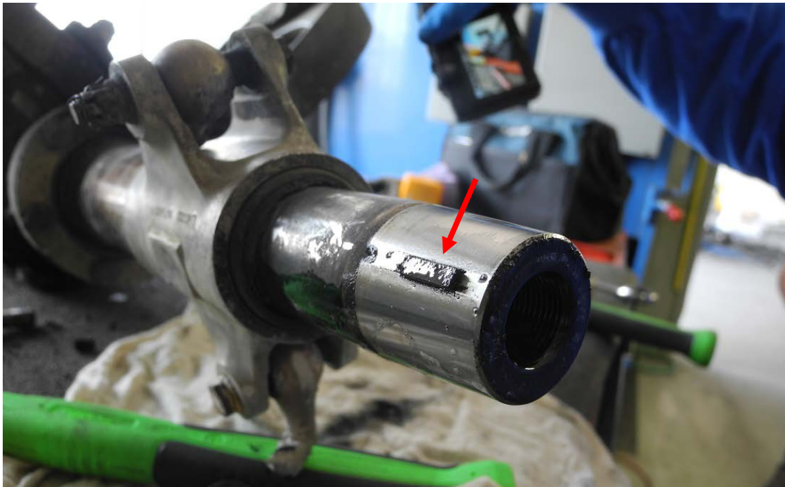
Photo 14. Output shaft key (red arrow) on the tail gearbox output shaft.
