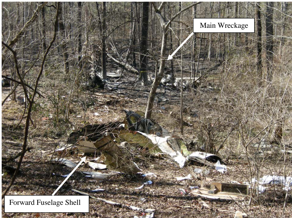
Figure 1: Accident Site with Forward Fuselage Wreckage in Foreground and Center Wing Area/Empennage Wreckage in Background
