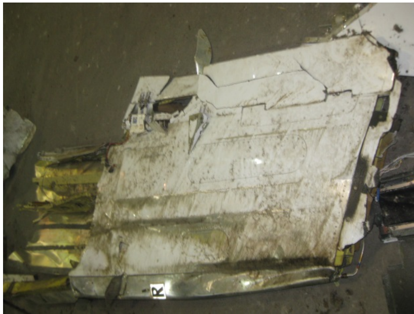
Figure 9 - Abrasions on Lower Wing Surface
