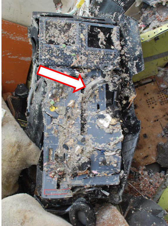
Figure 7 - Center Pedestal and Throttle Quadrant (Arrow points to thrust levers)
