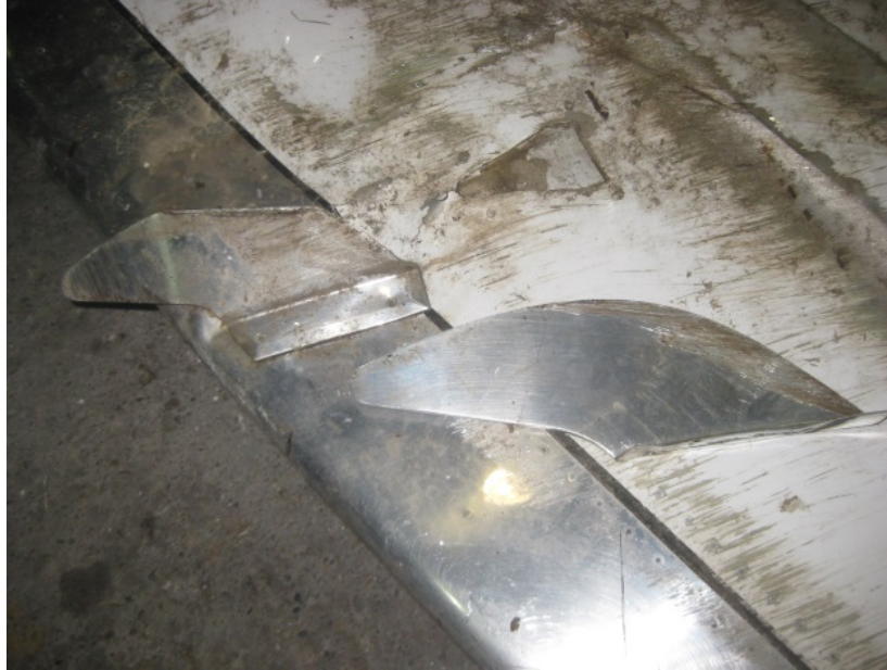
Figure 8 - Abrasions on Lower Wing Surface
