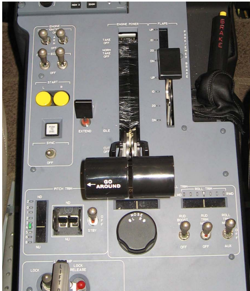
Figure 6 - Throttle Quadrant and Engine Controls, including IDLE and CUT OFF positions (picture taken in sister ship).
