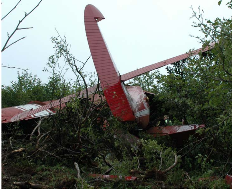
Figure 27A. Aft view of airplane, showing tail control surfaces, including trim. The right float is beneath the right side of the fuselage with the keel toward the camera.
