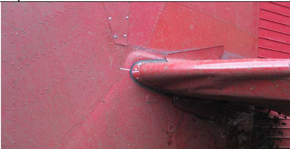
Figure 27B. Left side of horizontal stabilizer that is shown in Figure 27A, showing closeup of trim setting found.
