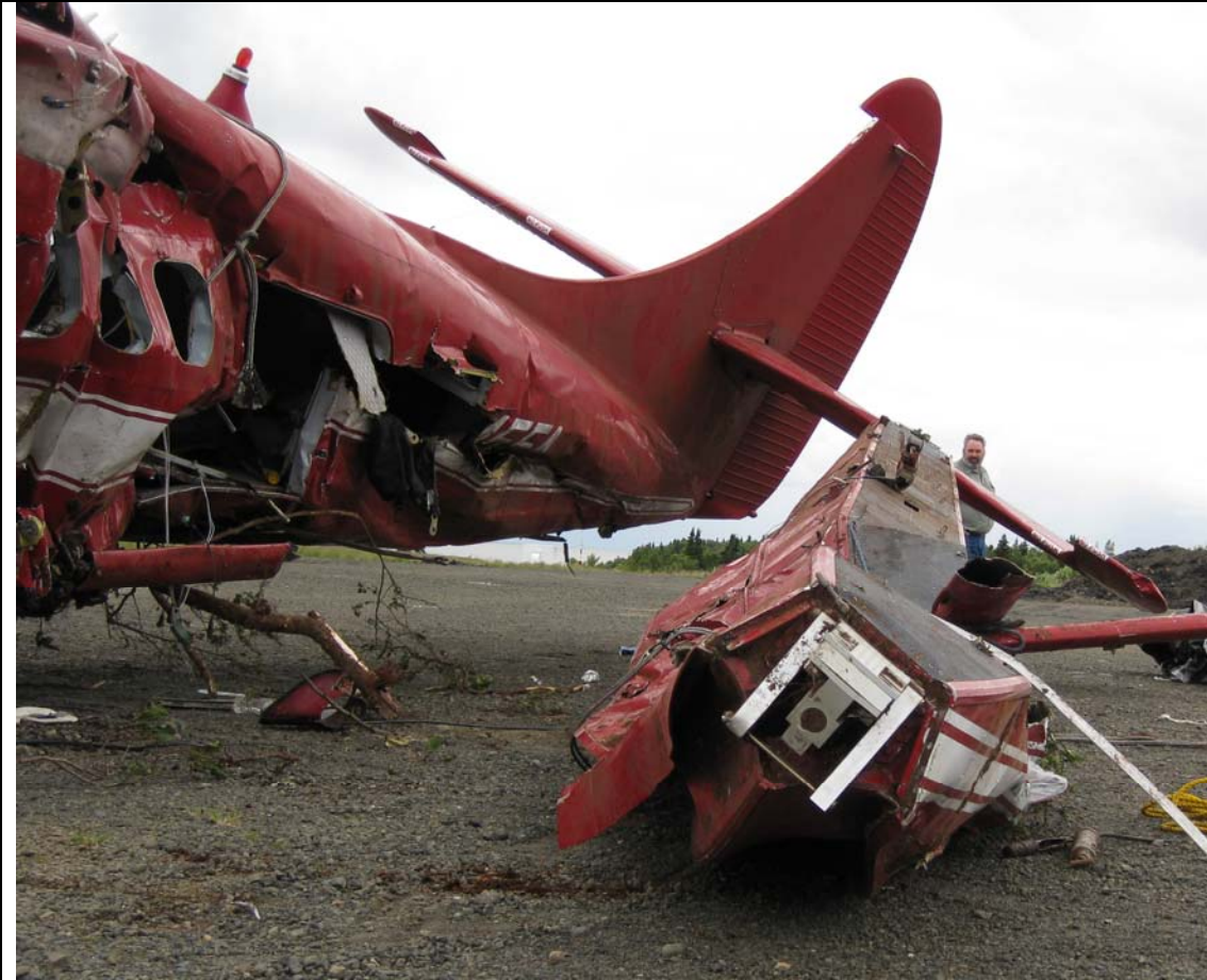
Figure 13. Left float, showing crush from front.
