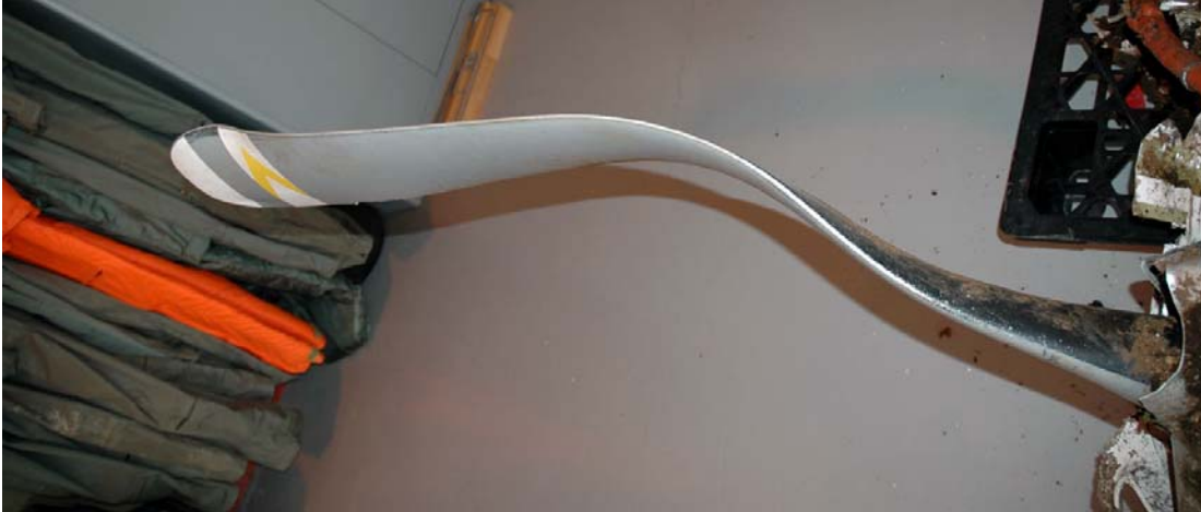
Figure 78. Bending in Propeller Blade, with leading edge toward camera.
