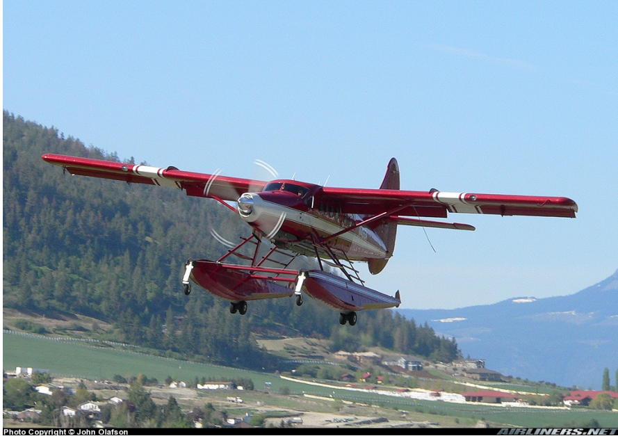
Figures 8. Pre-accident view of the N455A airplane to show the height of the ventral fin above the rear float spreader bar. Note the extended flaps and nose above cruise attitude.
