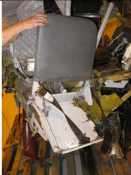
Figure 33. Copilot seat, showing the fractured and missing portions of the seat pan.
