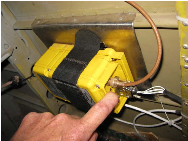
Figure 71. ELT in another Otter, showing gap between the ELT and mount that was created by finger tension. Forward is to the right.
