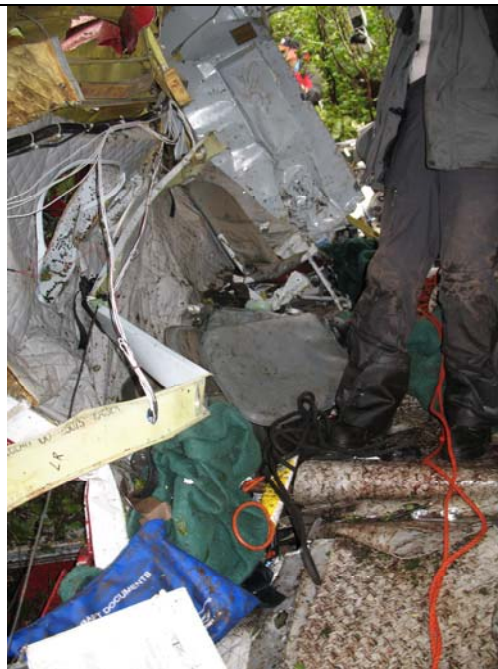
Figure 23. View from aft of cabin to show disruptions to the left cabin side wall and floor prior to recovery. Figure 22 showing the same features from the other end of the cabin was photographed from the where green foliage can be seen at the top of this photo.
