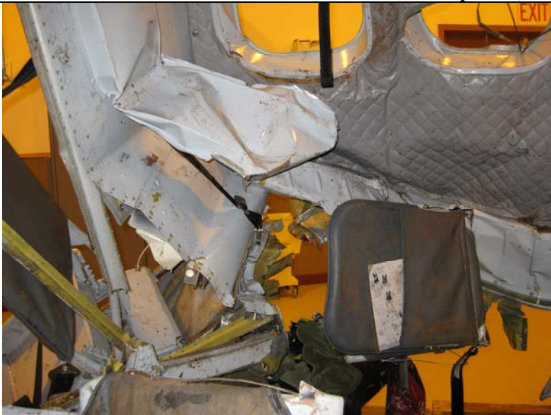
Figure 35. Seat #4, the forward most right cabin position, showing absence of floor structure and upward deformation beneath the seat.
