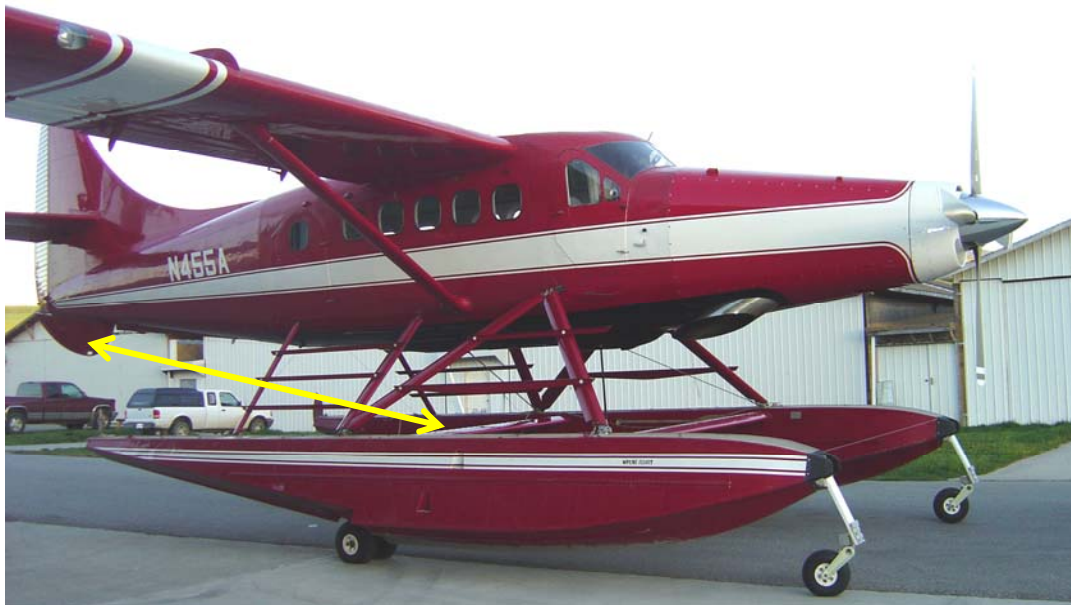
Figure 7. Pre-accident view of the N455A airplane to show the height of the ventral fin above the rear float spreader bar.
