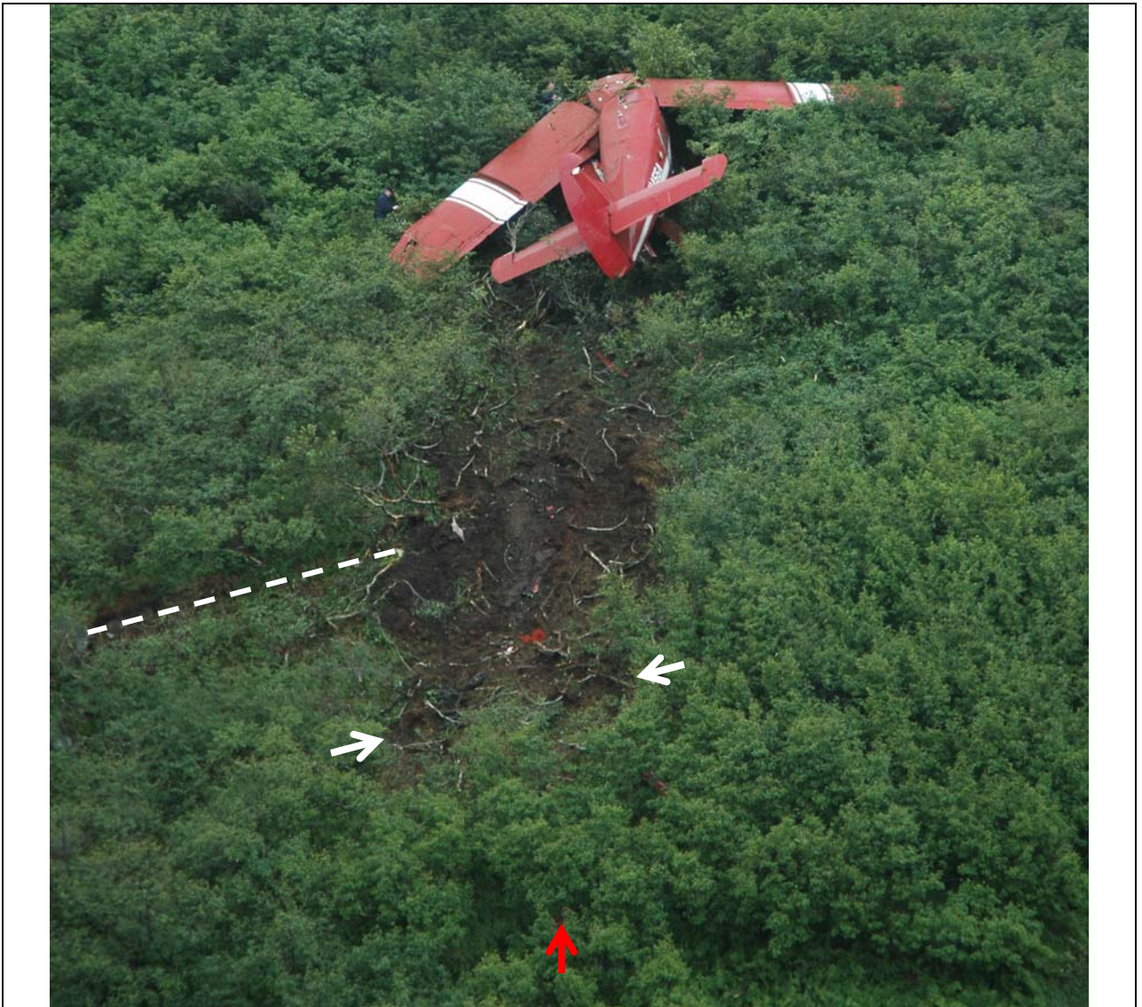
Figure 10. From directly behind the airplane, the small red arrow at the bottom of the photo shows where the first piece of airplane (ventral fin) was found. The white arrows point to the imprints of the floats, the left being the first ground contact. Around the dashed line is a cut in the alders that had the span of the left wing.
