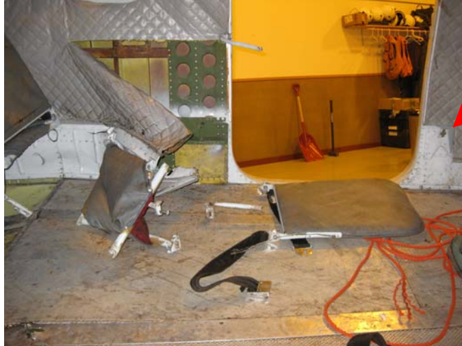
Figure 39. Fragments of seat #9. The arrow points to the broken structure that seat #11 had been attached to.
