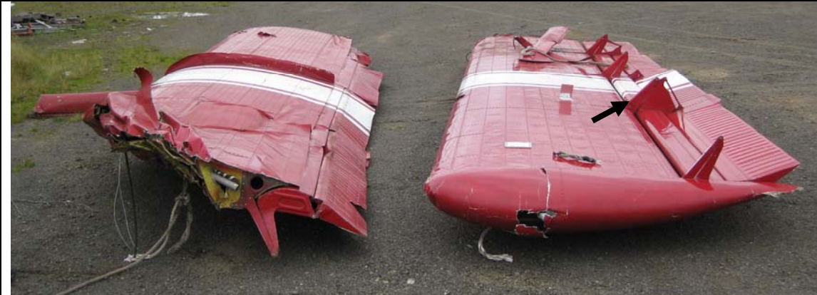
Figure 25. The upper surface of the left wing and bottom of the right wing, shown respectively from the tip ends. The arrow placed on the right wing shows where a broken control rod was found.
