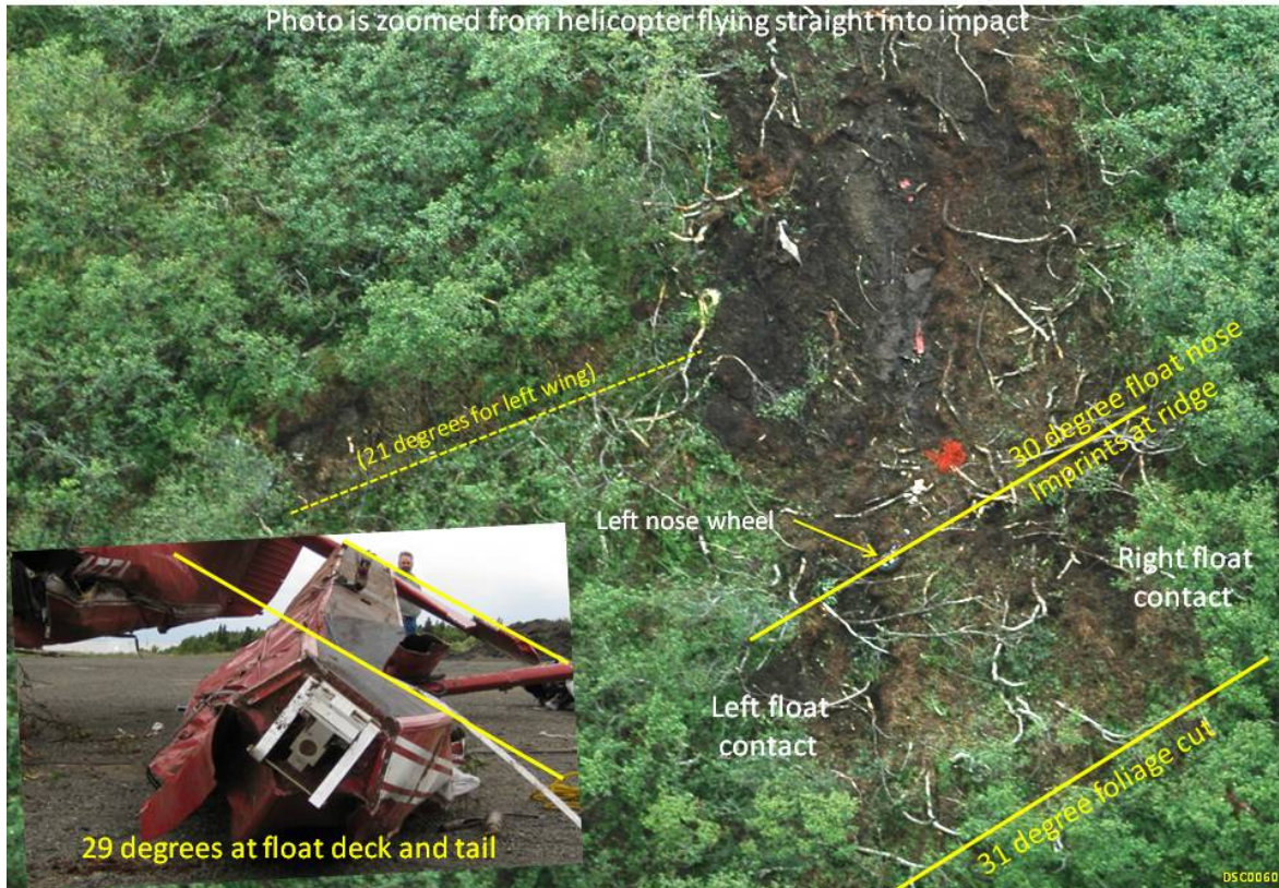
Figure 11. The above figure shows bank angle damage measurements. The float photo is cropped from Figure 13.
