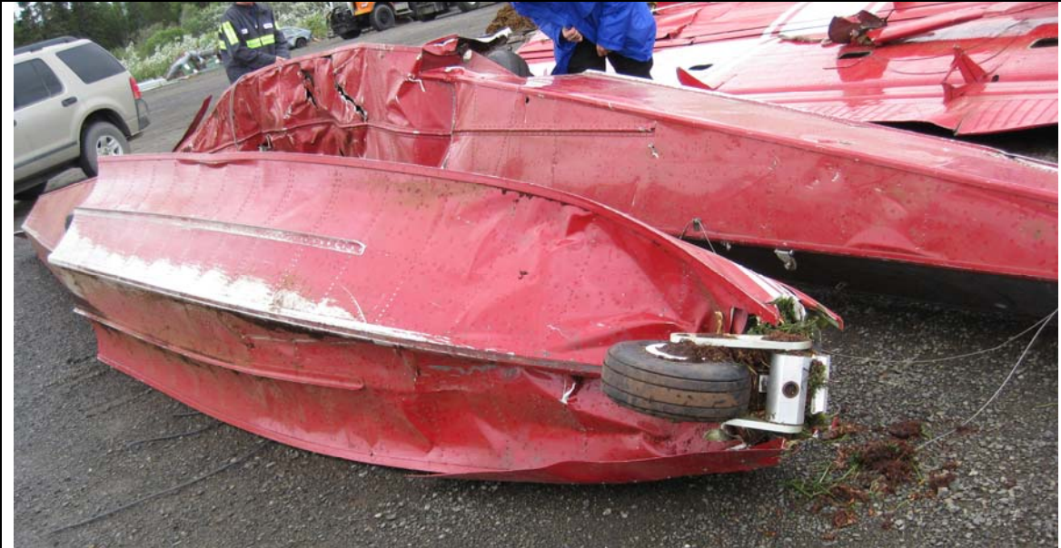
Figure 15. Forward features of the right float. The left float is behind the right float, illustrating the difference in extent of crush damage to the bottom surfaces.
