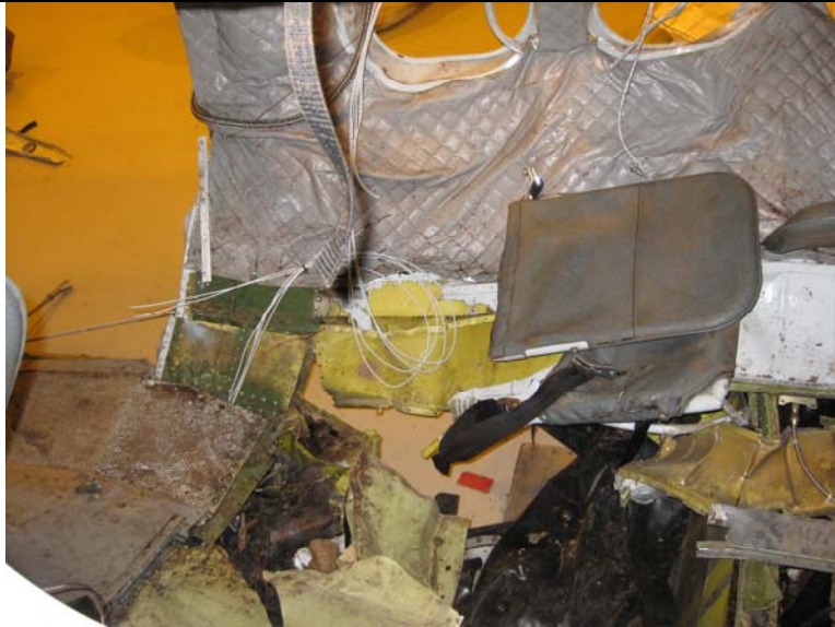
Figure 36. Seat #5, this was the second cabin seat on the left and the photo shows absence of floor structure. Seat #7 had been aft of this seat and fell away during recovery.
