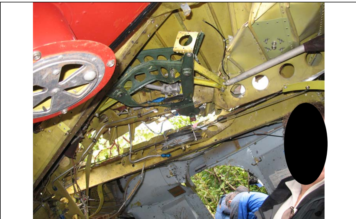
Figure 26. Extensive component and structural damage at the fuselage breach near the flap actuator and control quadrant above what had been the cabin ceiling.
