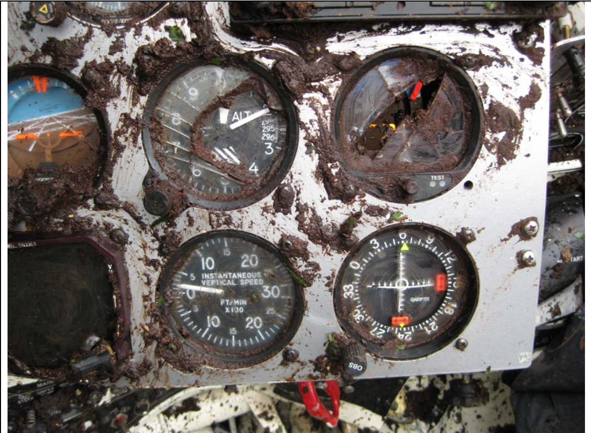
Figure 44. Primary flight instruments, after wiping away some of the mud that is visible in Figure 42B.
