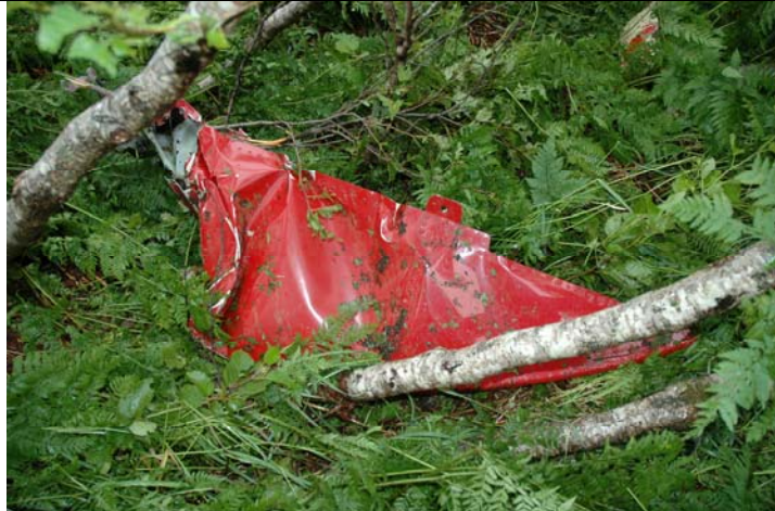
Figure 6. Left side of N455A ventral fin, showing impact marks on leading edge (left edge of what is visible).
