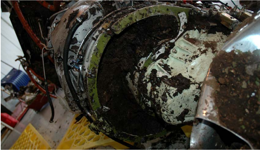
Figure 74. Dirt found in engine inlet
