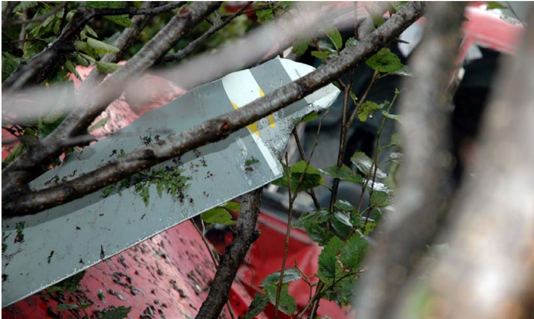
Figure 79. Propeller blade tip damage.
