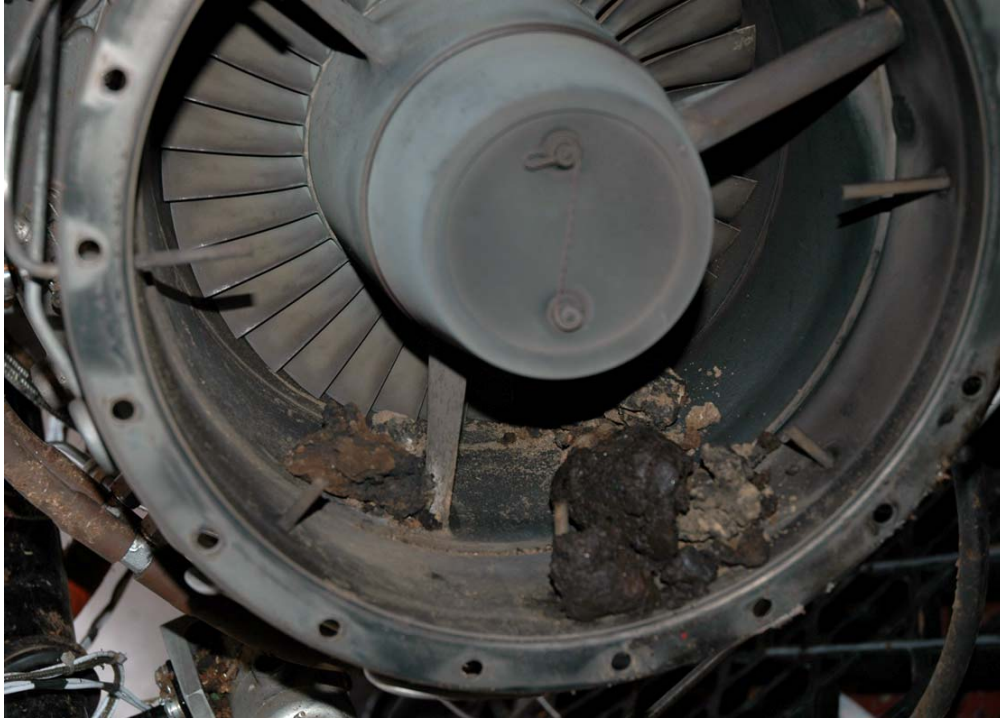
Figure 76. Engine exhaust area and third-stage turbine wheel.
