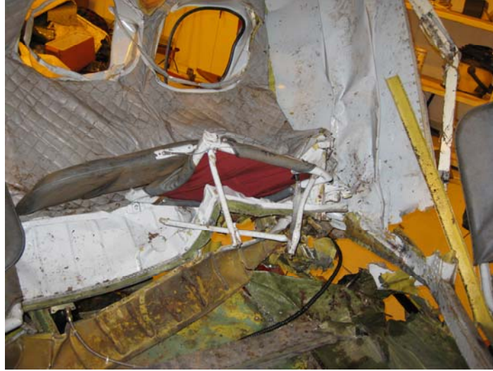
Figure 34. Seat #3, the forward most left cabin position, showing absence of floor structure and upward deformation beneath the seat.
