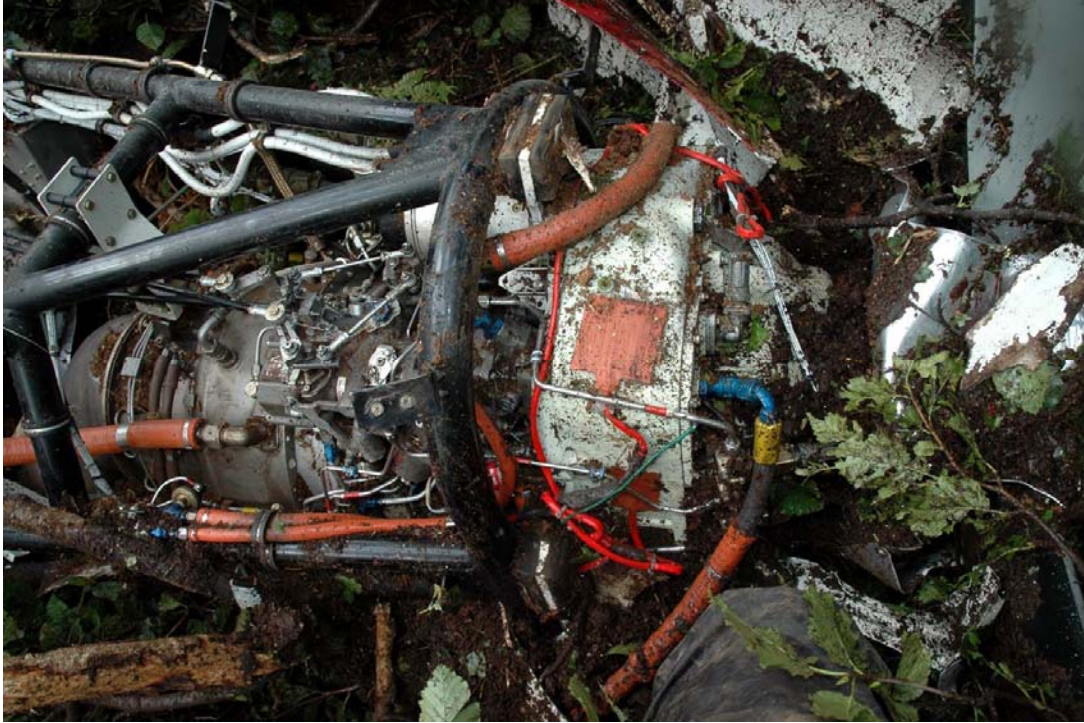
Figure 72. Engine after the cowling was removed
