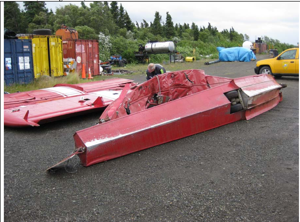
Figure 16. Right float appears to be relatively intact when compared to the bottom of the left float (behind the right float).
