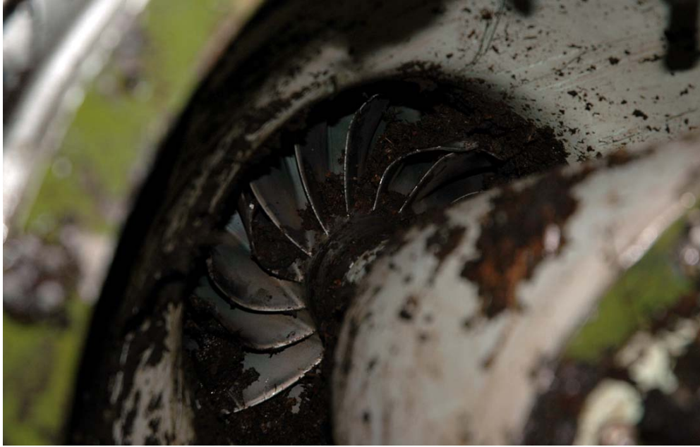
Figure 75. Damage to the first-stage compressor impeller.
