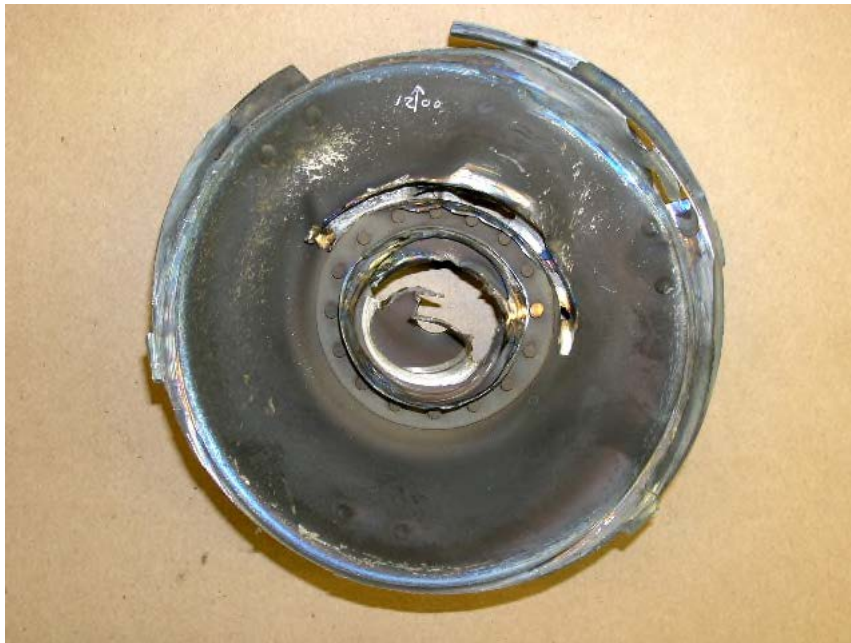
Photo No. 44 Interstage baffle, upstream side.
