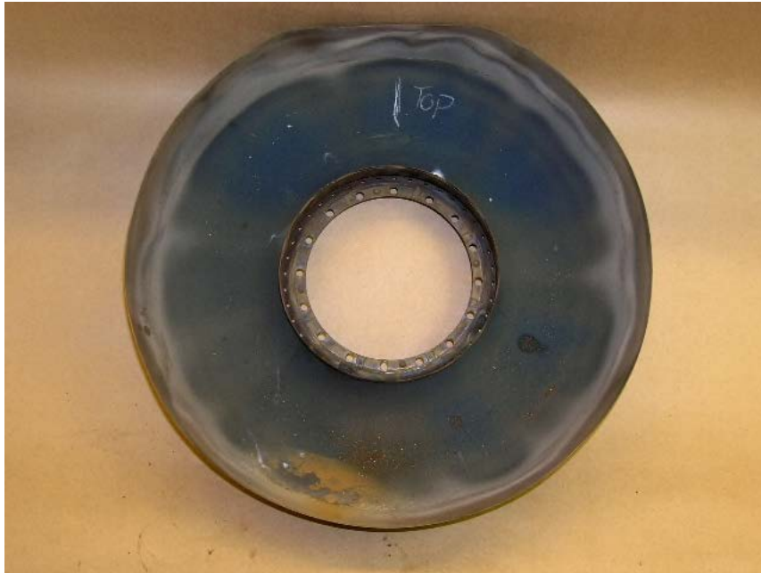
Photo No. 23 Large exit duct.
