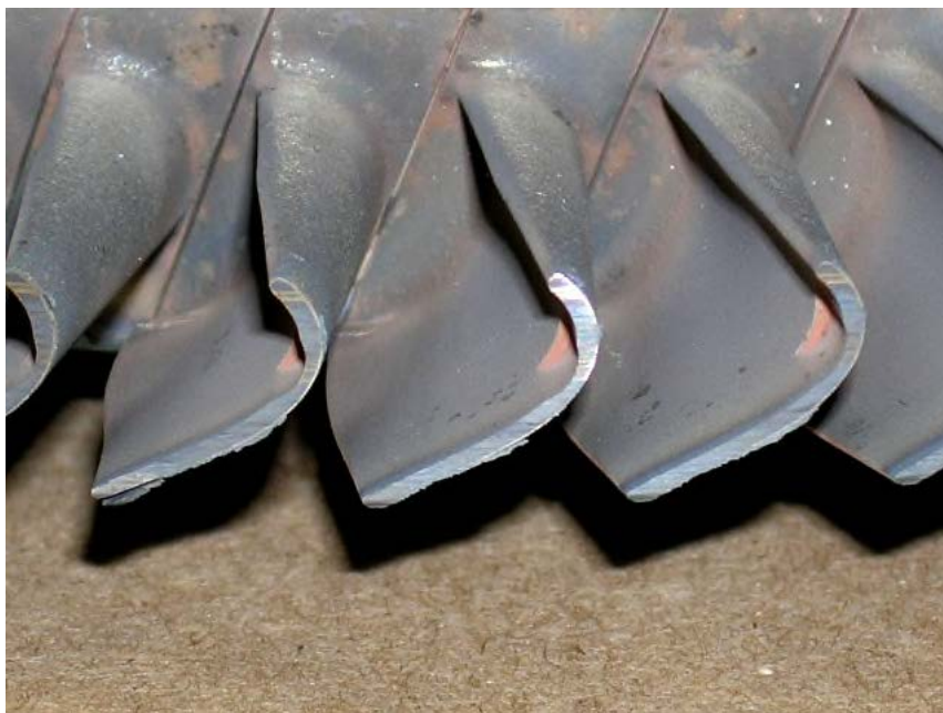
Photo No. 34 Compressor turbine blade tips, detail.
