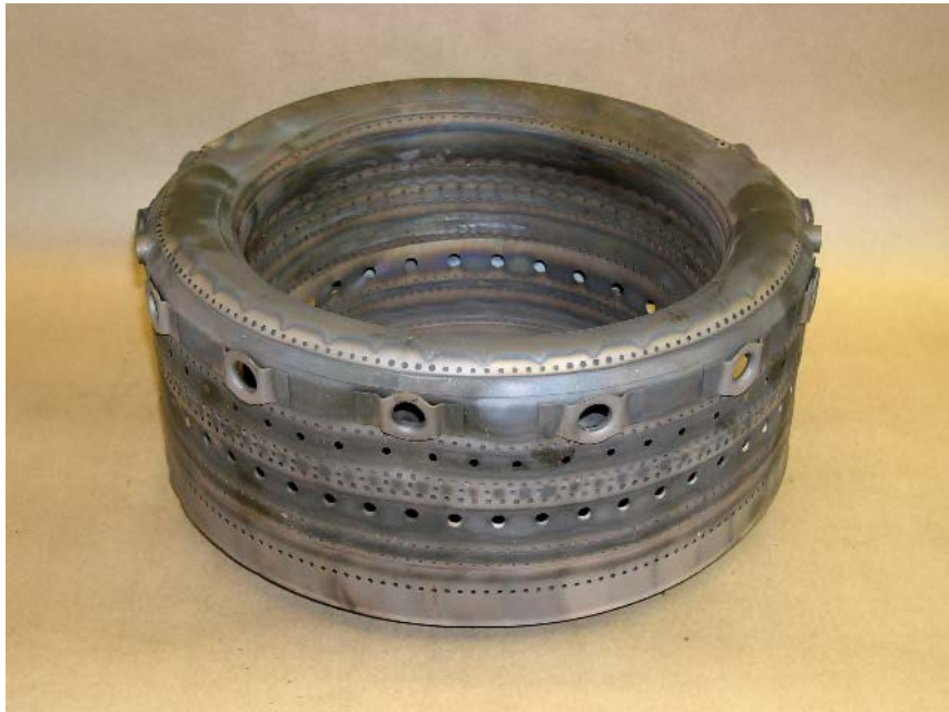
Photo No. 24 Combustion chamber liner.
