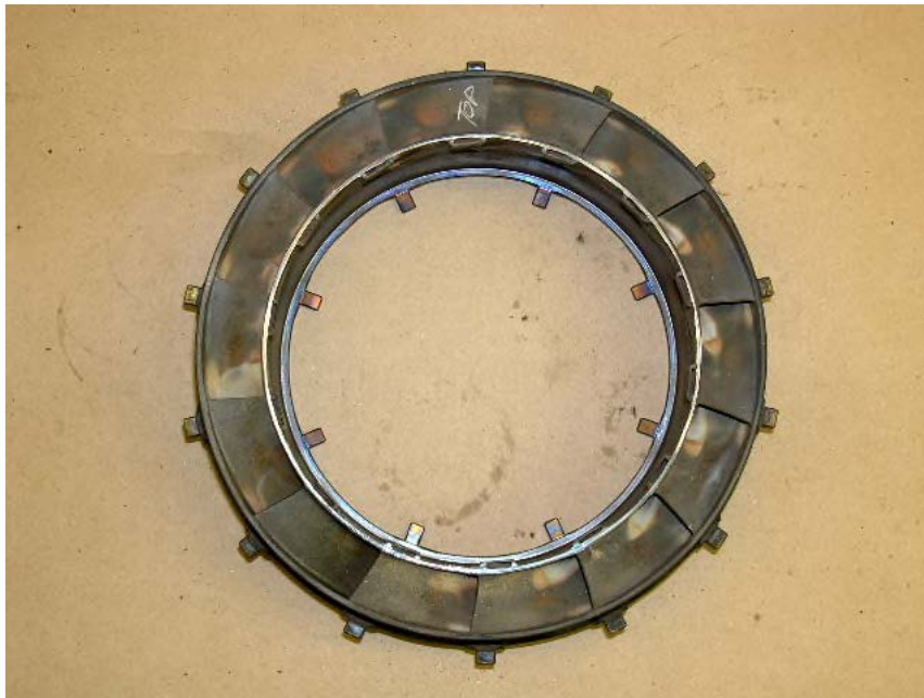
Photo No. 26 Compressor turbine guide vane downstream side.
