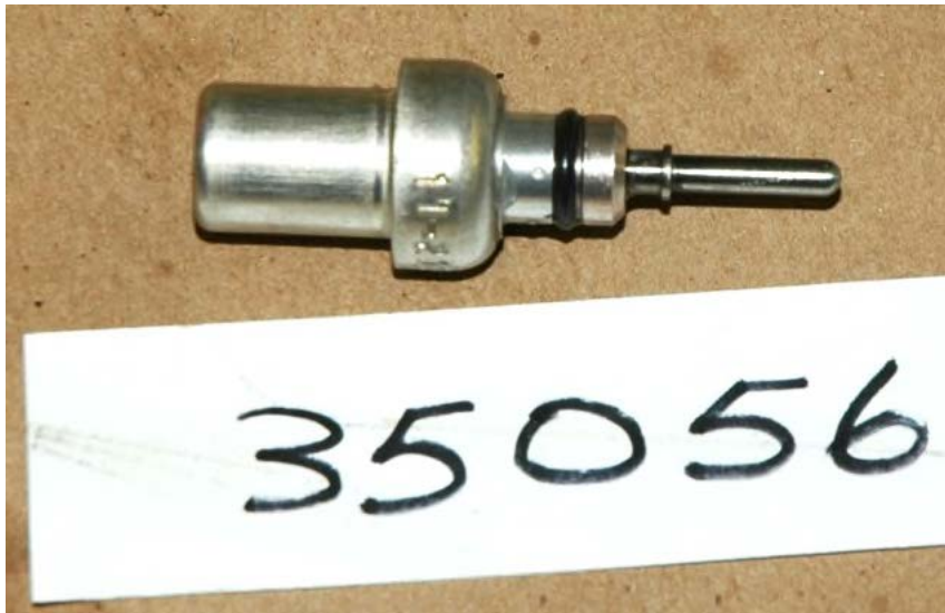
Photo No. 65 Fuel heater thermal element.
