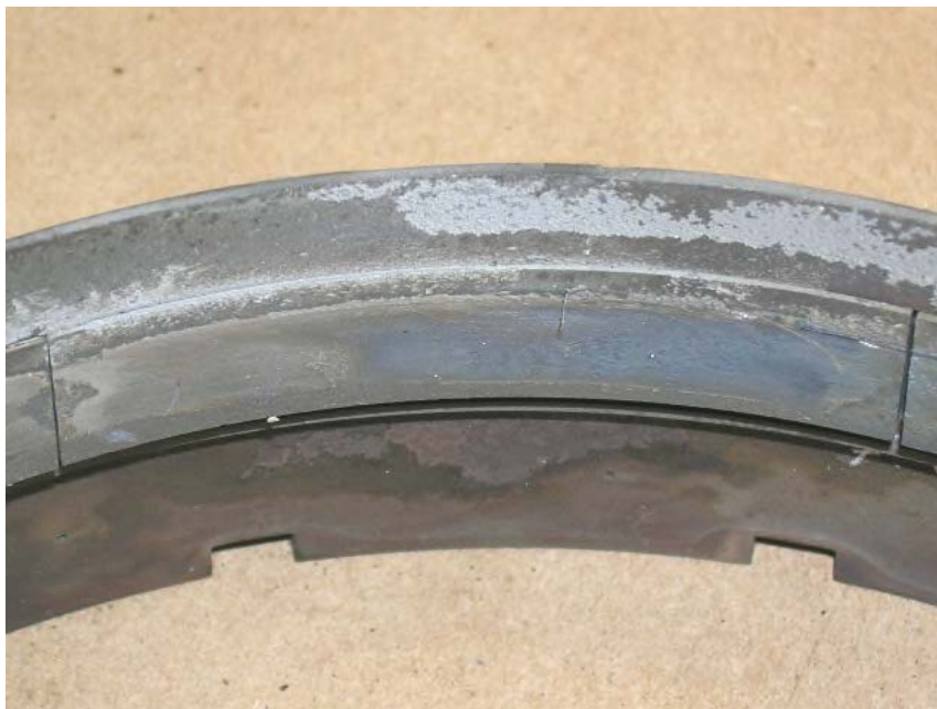
Photo No. 29 Compressor turbine shroud lower circumference, detail.
