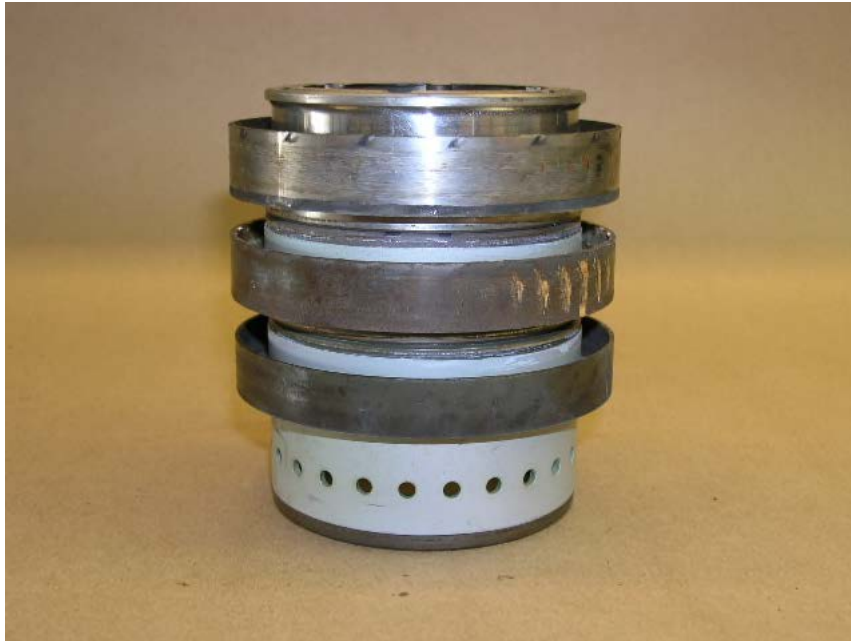
Photo No. 14 Compressor 1 st , 2 nd and 3 rd stage spacers.
