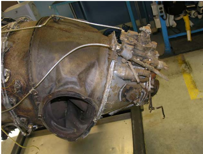
Photo No. 5 Reduction gearbox and exhaust duct, right hand top view.
