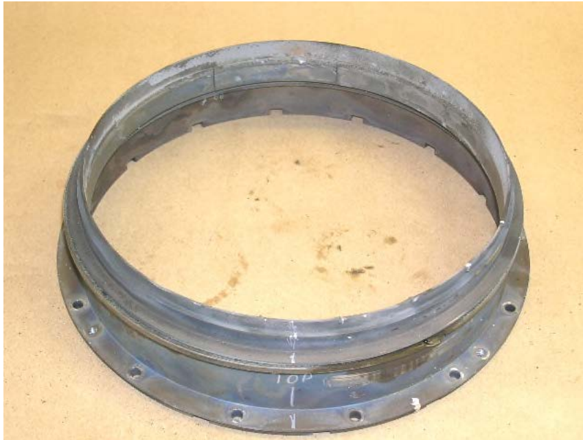
Photo No. 28 Compressor turbine shroud.
