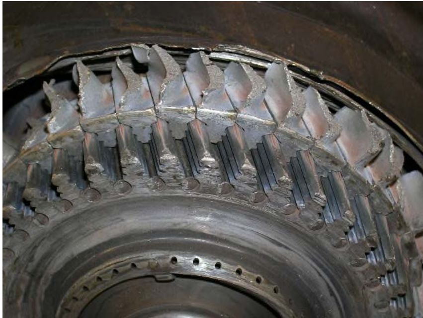
Photo No. 51 Power turbine downstream side, in-situ, detail.
