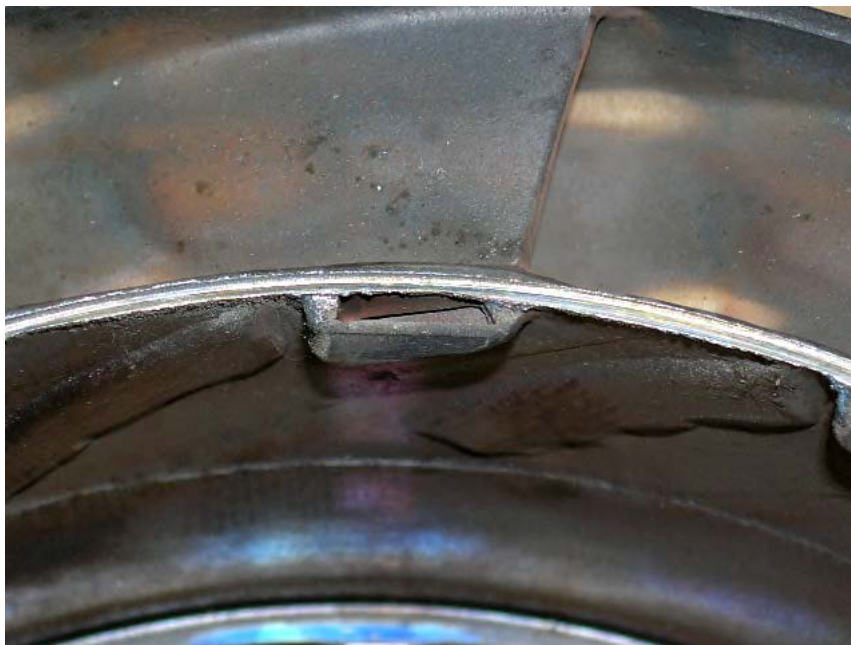
Photo No. 27 Compressor turbine guide vane ring downstream side, detail.
