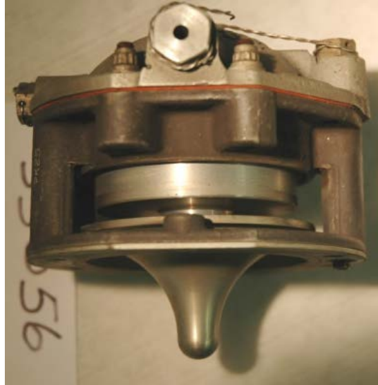
Photo No. 71 Compressor bleed valve.
