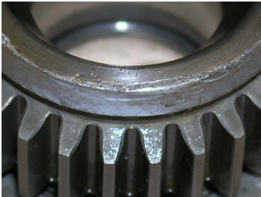
Photo No. 57 1 st stage planet gear carrier hub 2 nd stage sun gear input spline, detail.
