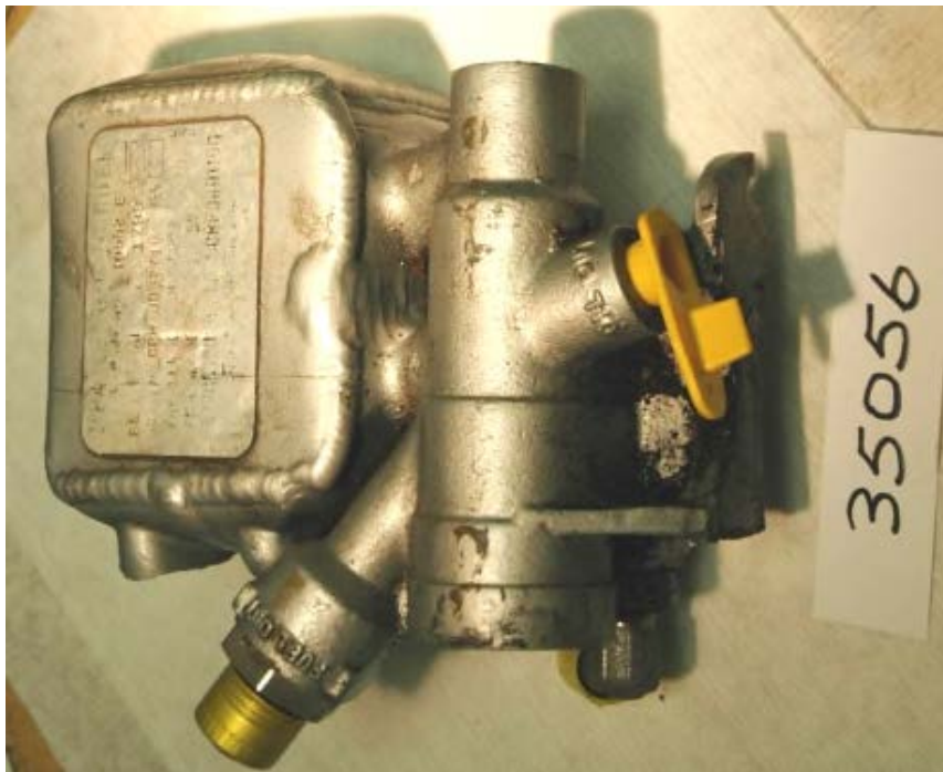
Photo No. 64 Oil to fuel heater.
