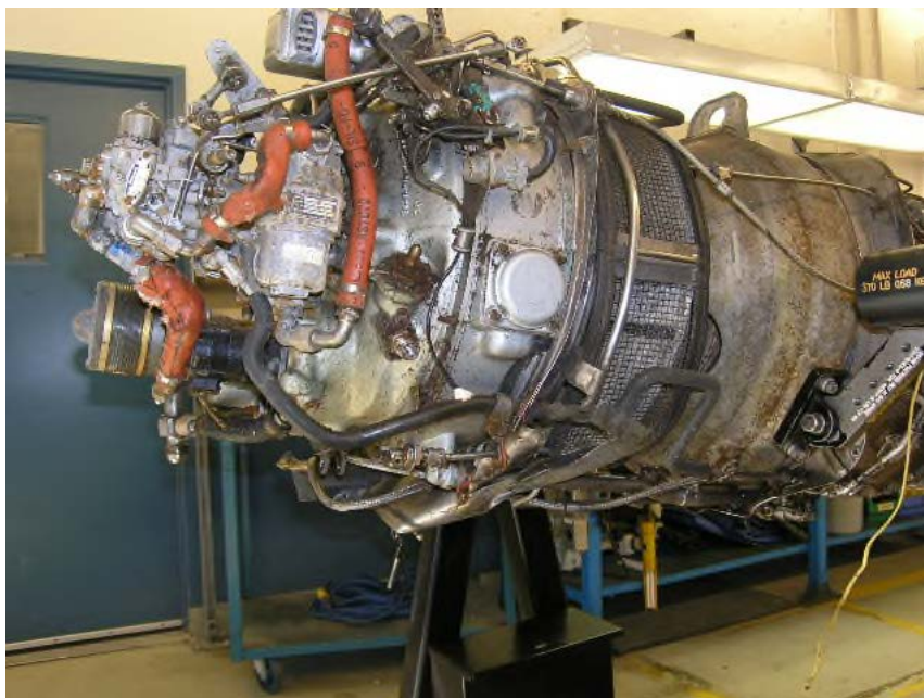
Photo No. 6 Aft gas generator case and accessory gearbox, lower right hand view.
