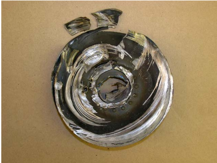
Photo No. 46 Interstage baffle, downstream side.
