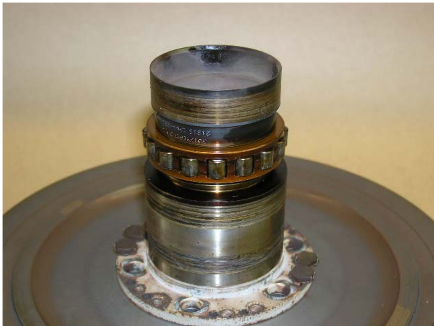
Photo No. 21 No. 2 bearing and air seal rotors, in-situ.
