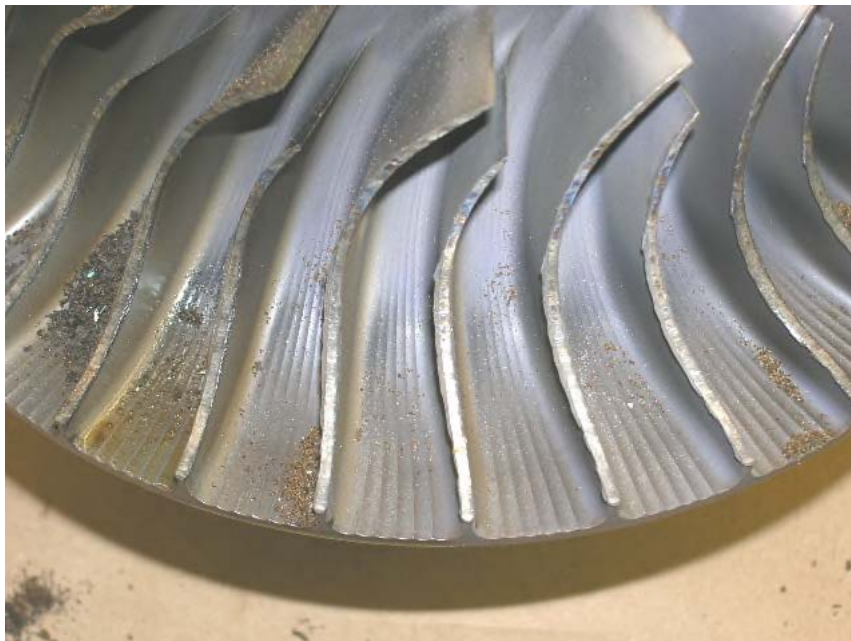
Photo No. 18 Centrifugal impeller, detail.
