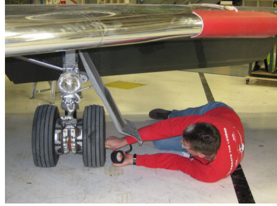
Figure 26. Checking outboard tire pressure at the Learjet factory.
