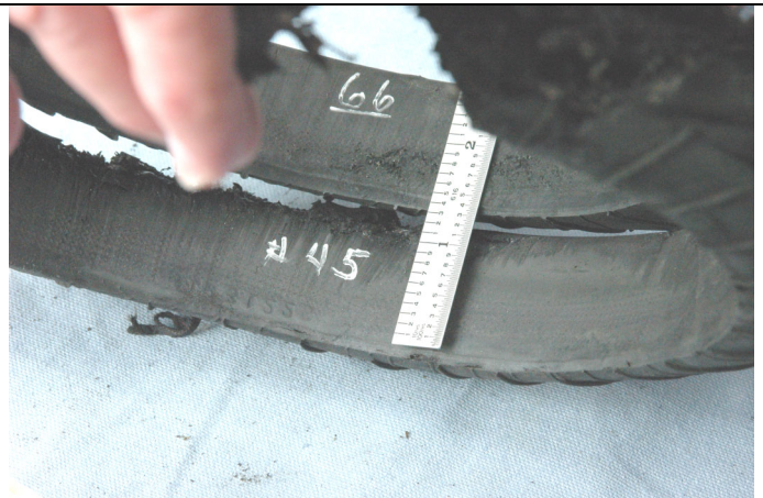
Figure 29. These fragments from N999LJ show the tire beads (Fragments #45 and 66), and the lack of heat-type damage that is visible in the photo to the left. Specifically, note the lack of damage under the lettering "45" and "66." The ragged edges visible in this photo are where the bead material had rolled on the grooved pavement.
