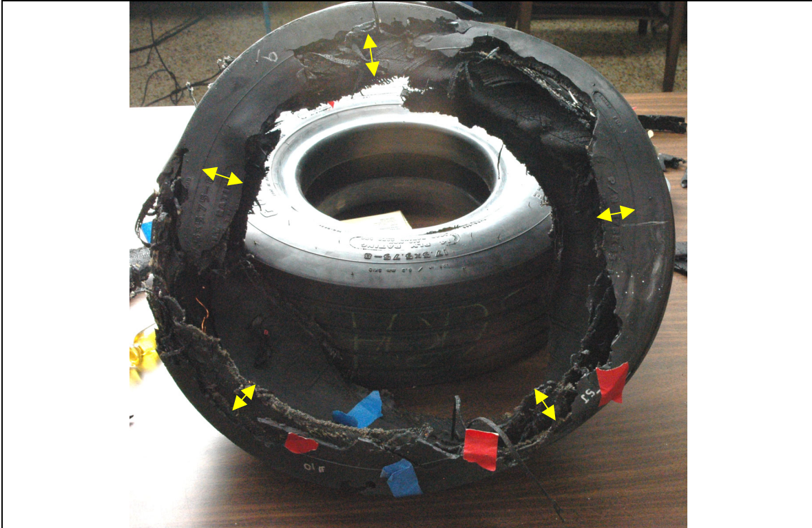
Figure 21. Overall photograph of the reconstruction of the right outboard tire, on the outboard sidewall. 21 Visible is the generally ragged or torn appearance of the edge that is at a relatively constant radius from the hub. The added arrows show the relatively constant distance from a decorative rib.
