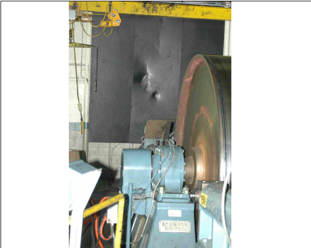
Figure 4. Dents in the diamond-plate steel on the walls of the Goodyear dynamometer test room. For scale reference, the large steel wheel is 120 inches in diameter and the smaller dent is fully the size of a man's fist.
