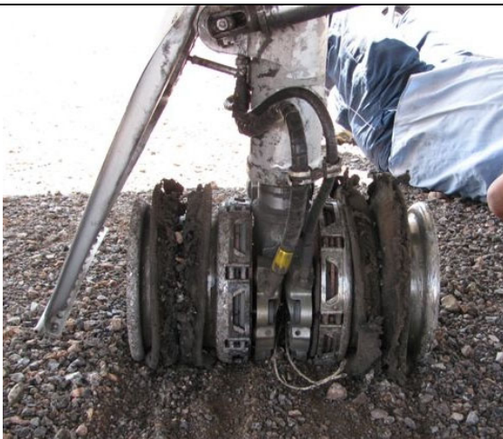
Figure 14B. View from the rear of the airplane, XB-MYG, showing the left wheels and tire remnants.
