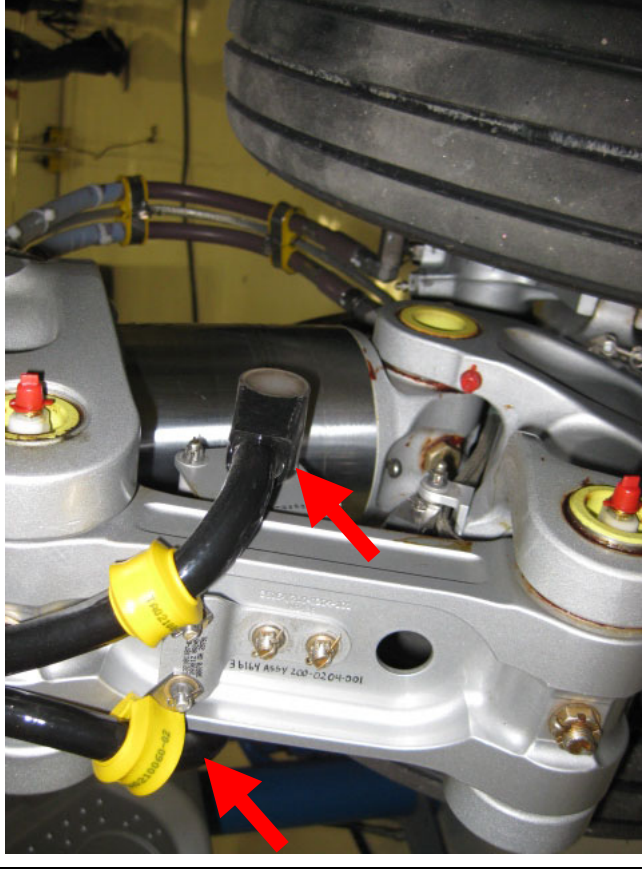
Figure 37A. Learjet Model 45 right main landing gear. The arrows point to the dual squat switches located within the forward scissors assembly.
