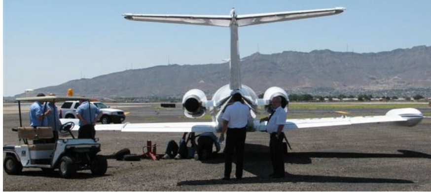
Figure 14A. XB-MYG displays 1.8 to 1.9 degree airplane roll angle that existed with flat right tires and resting on left wheel rims.
