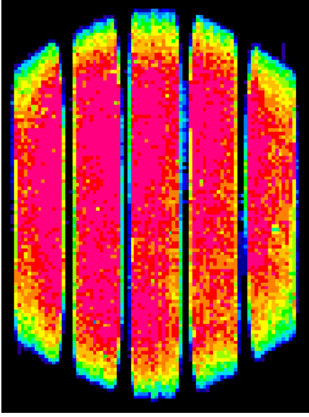
Figure 15E. Footprint at 0.55 degrees camber 7.67 inch SLR, 25.3% deflection, 30.48 sq in gross area
