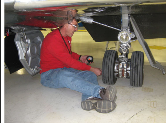
Figure 25. Checking inboard tire pressure at the Learjet factory.
