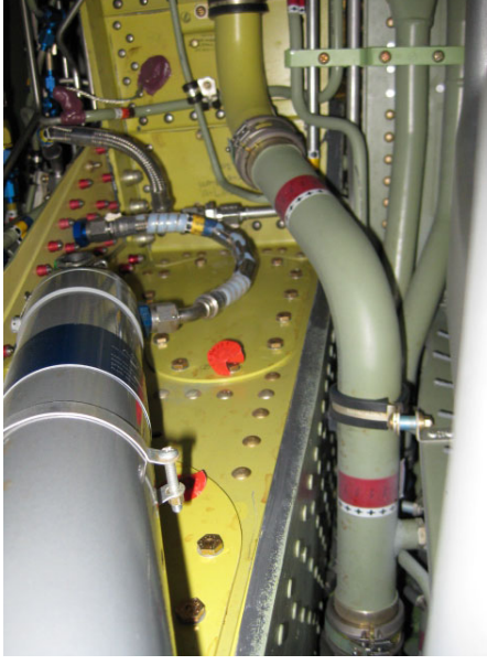
Figure40D. Learjet Model 60: View shows exposed hydraulic components on the front and inboard walls of right wheel bay inboard. (Composite of two photos)
