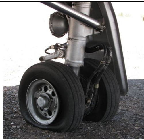
Figure 14B. View from the rear of the airplane, XB-MYG, showing the right wheels and deflated tires.
