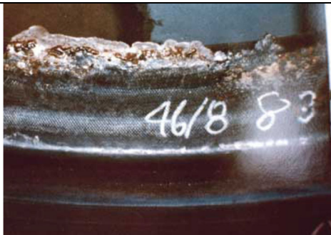
Figure 28. As copied from the Bridgestone Tire Care and Maintenance publication and as a comparison for the photo to the right. This photo shows how a tire bead with evidence of brake overheating could appear.
