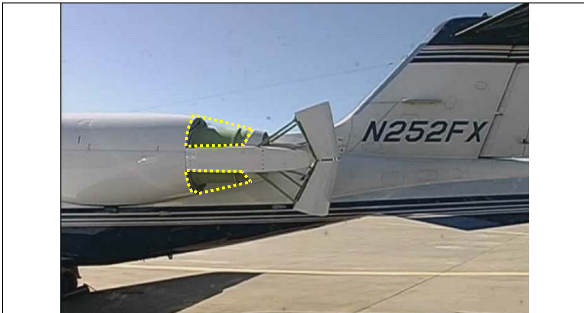
Figure 1. For reference and context of the following photographs, this shows the upper and lower thrust reverser doors in the deployed positions on a test airplane. The dotted lines show the stowed/closed positions for the doors, which can also be seen in Figure 2.
