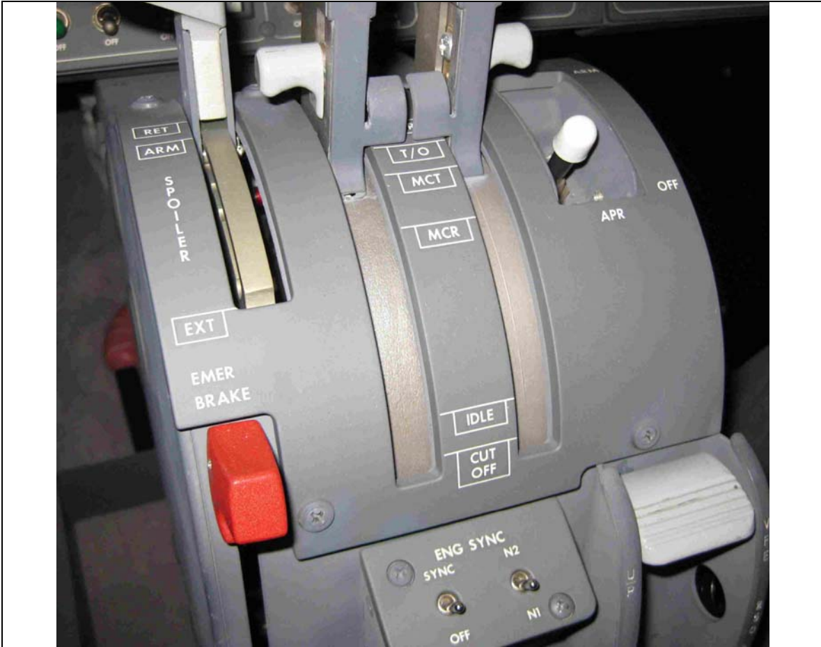
Figure 5. The throttle detent positions marked on the pedestal. The marked positions relate to the ranges shown in the next Figure. (Photo of airplane similar to N999LJ)
