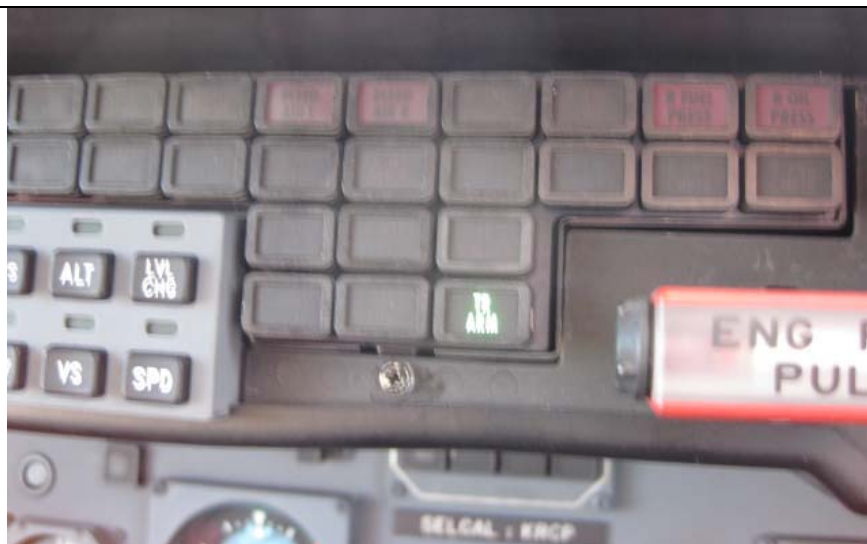
Figure 16. Illuminated right engine TR ARM green annunciation during ground test. (Photo of airplane similar to N999LJ)
