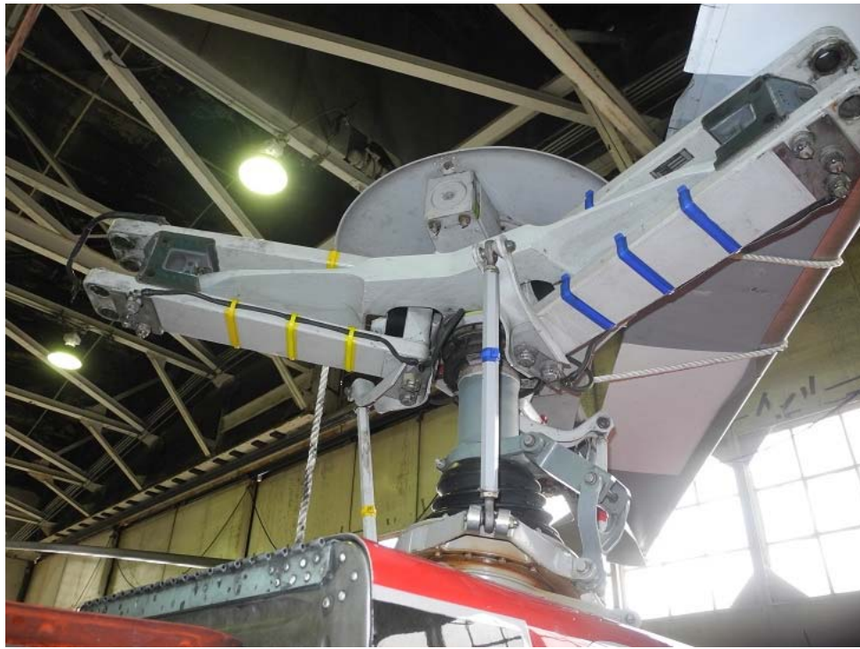
Figure 3. Main rotor Starflex and the 'yellow' and 'blue' sleeve assemblies.
