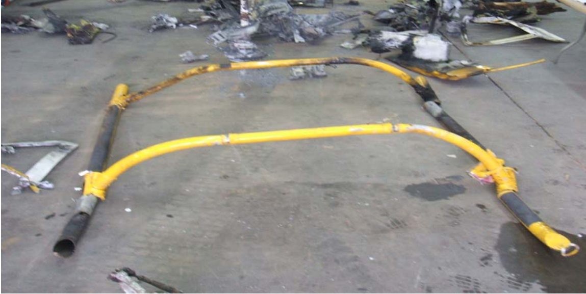
Photo 21: Main Landing Skid System.
