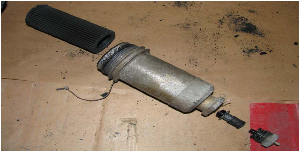
Photo 20: Hydraulic Fluid Filter
