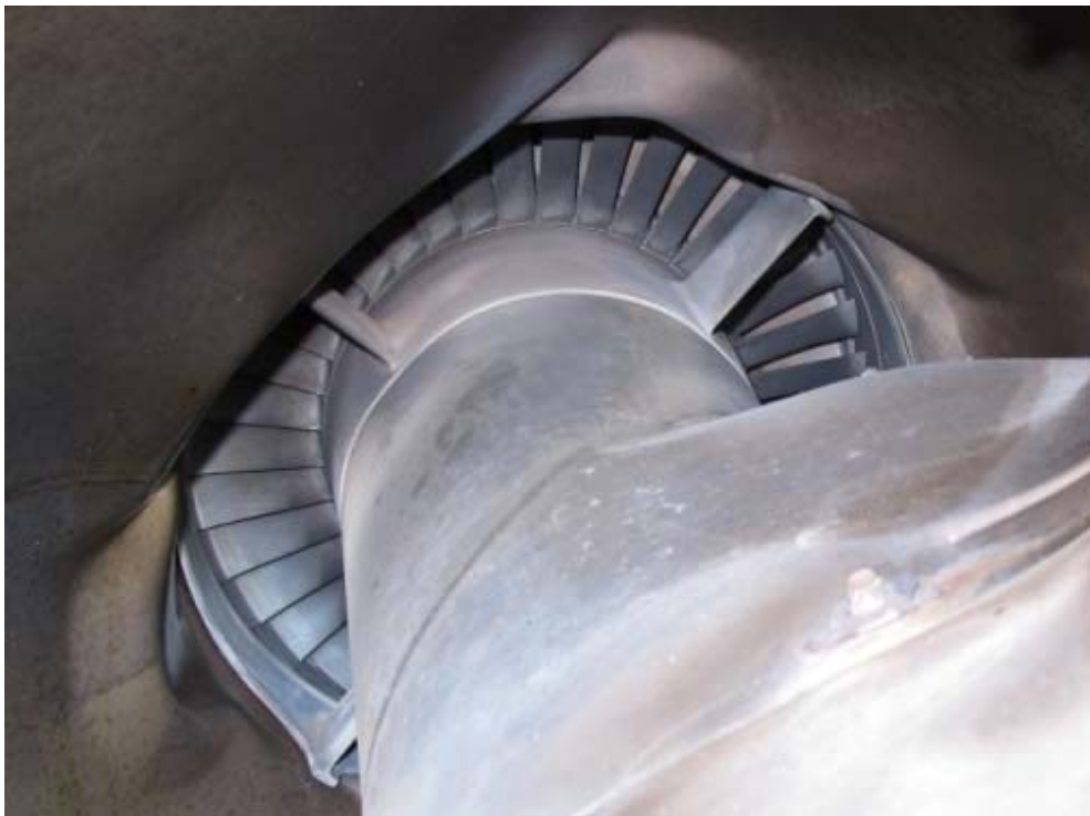
Figure 12: Photo the of power turbine blades viewed through the exhaust pipe
