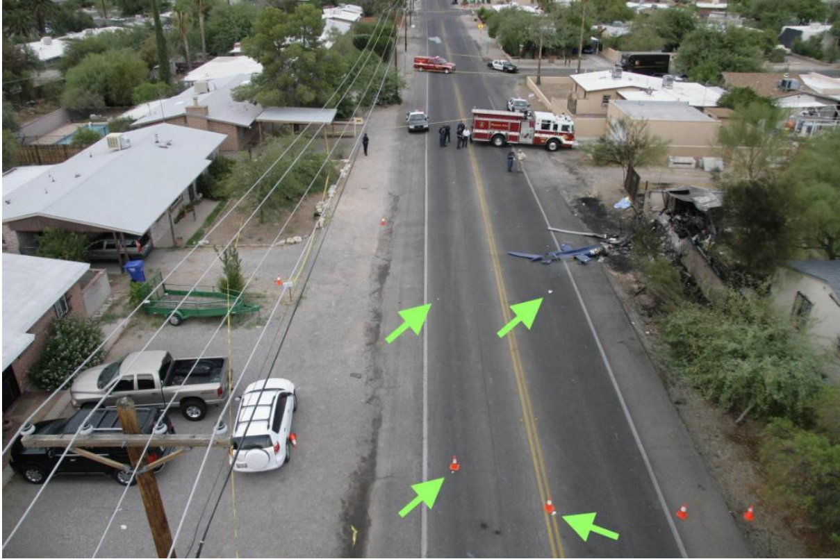
Figure 2: Photo of accident location viewed from above and to the north. Power lines are to the left, with fuel tank fragments indicated by green arrows. The tail boom is visible lying on the right side of the road.
