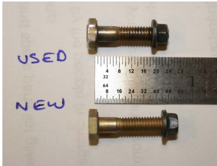
Figure 13: Photo of new and used union attachment nuts and bolts, with the nuts tightened by hand.
