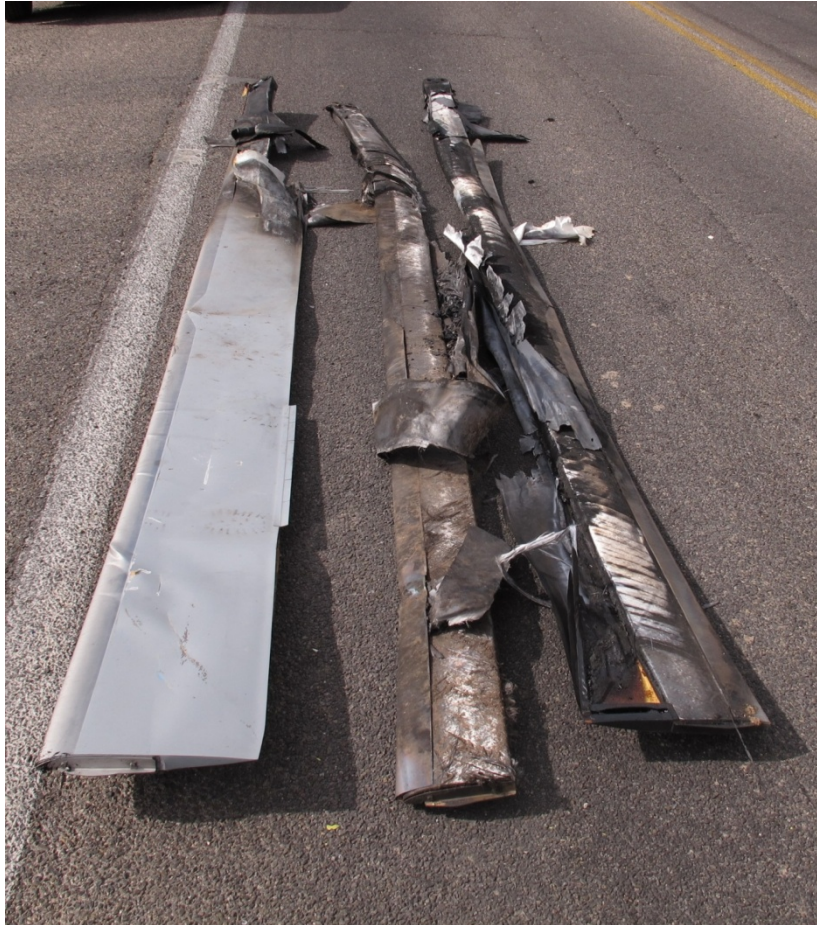
Figure 6: Photo of main rotor blades after removal from immediate accident site.
