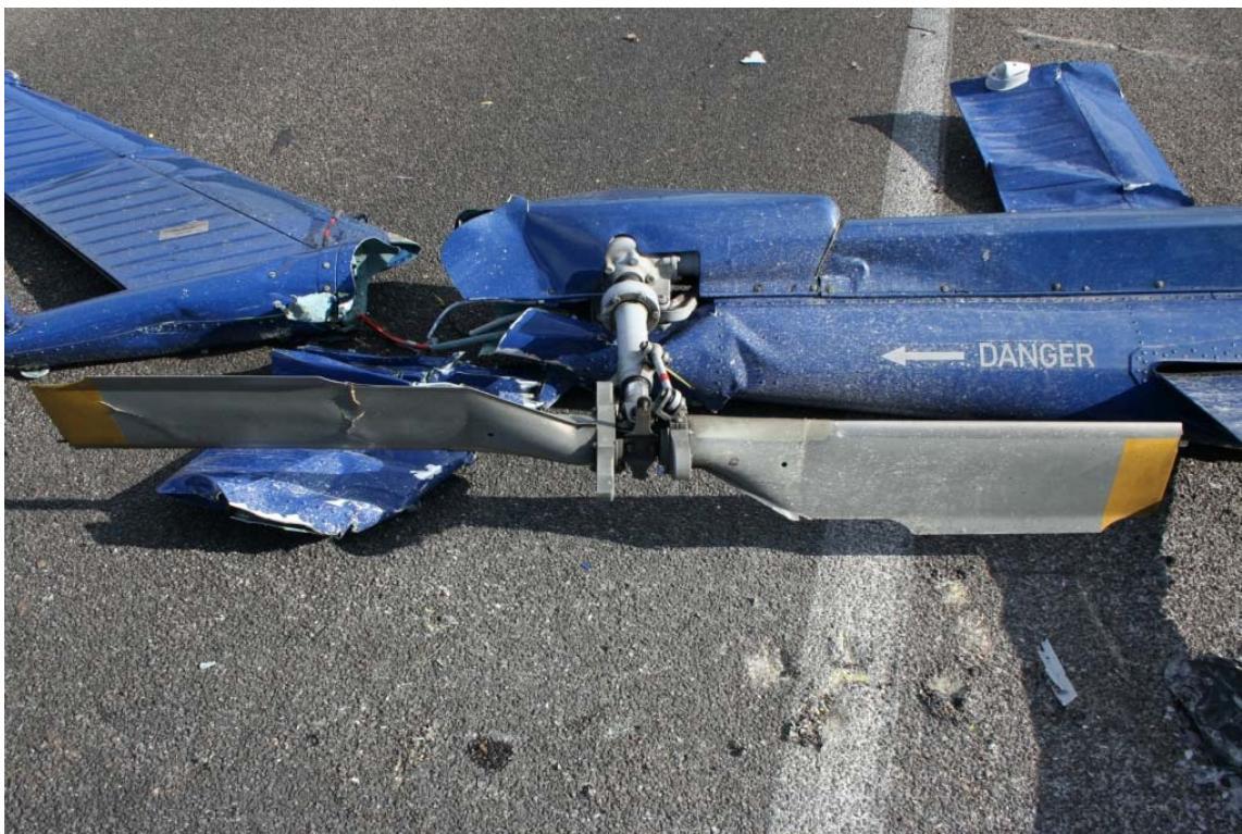
Figure 5: Photo of tail rotor blades and gearbox affixed to aft tailboom. The lower right hand corner of image displays ground scars corresponding to balance weight contact.
