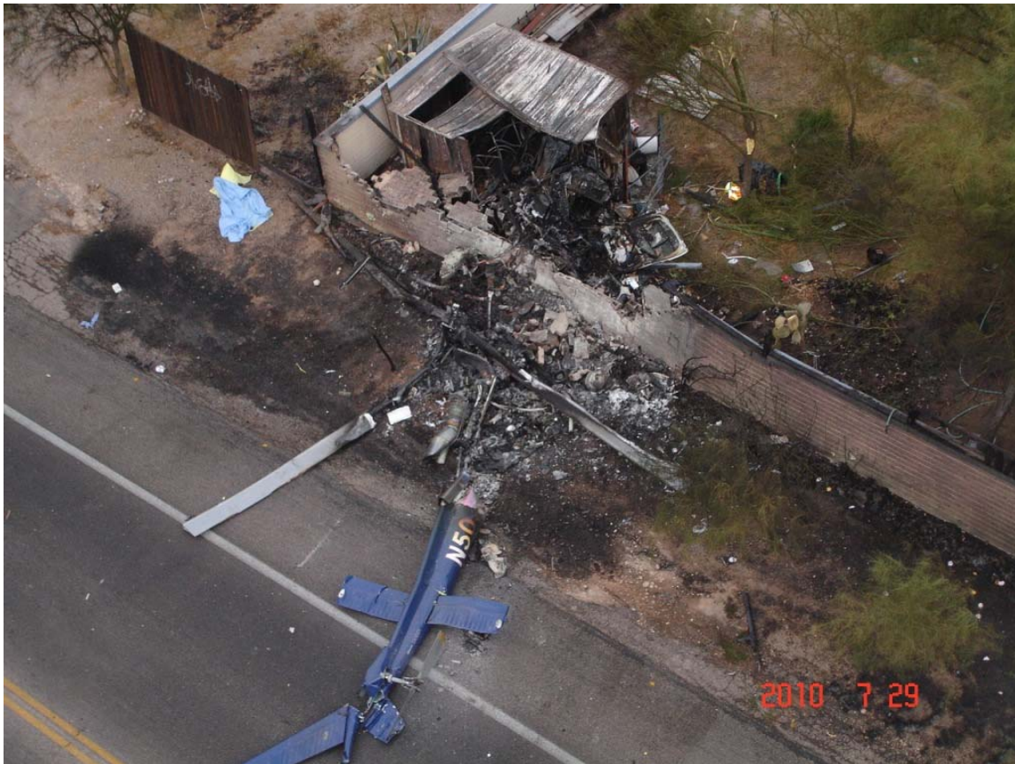
Figure 3: Photo of accident location viewed from above. The center fuselage structure is situated on the brick wall, which runs diagonally across this image. All three main rotor blades and the engine are visible in the center of image.
