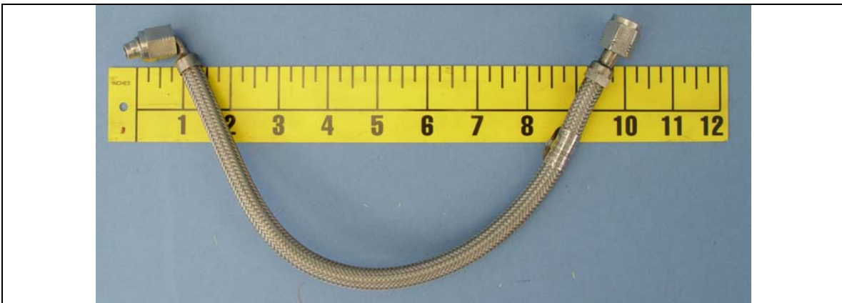
Figure 27. Detail of the Titeflex convolute hose from N799AX. (See Figure 22) The hose had an outer braid of stainless steel wire and welded end fittings.
