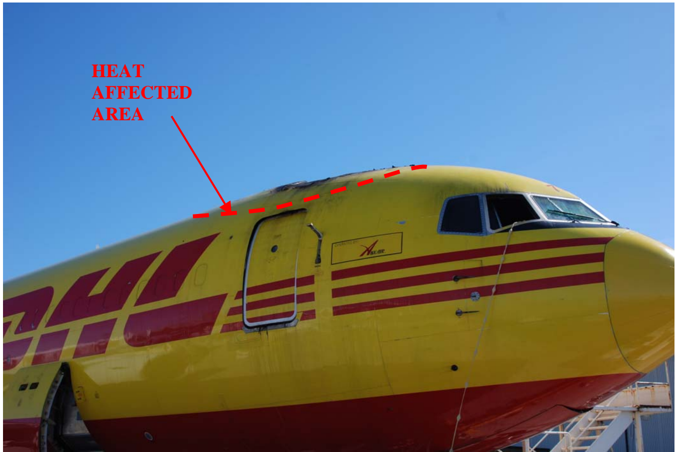
Figure 3. Heat damage to the right side of the fuselage, above the R1 door.
