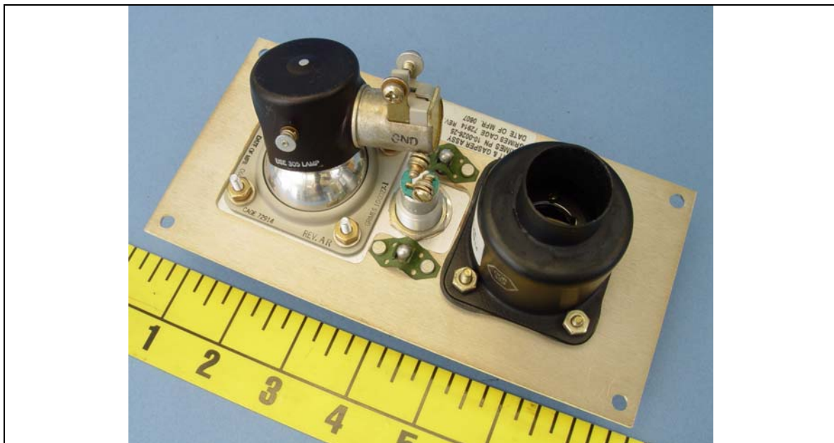
Figure 14. The same light assembly after rotating until the lighting shell contacted a potentially powered screw at the light switch.
