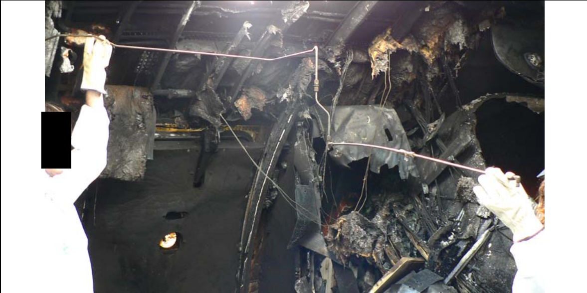
Figure 23. N799AX: The metal oxygen tube remained intact in the supernumerary compartment. The R1 door is in the background.
