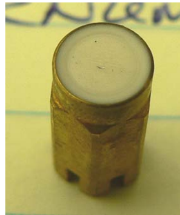
Figure 33. N799AX: The overpressure valve poppet from the supernumerary regulator
