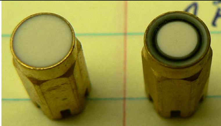
Figure 32. N799AX: New overpressure valve poppet on left. On the right is an overpressure valve poppet which was subjected to 140 psig for about 30 seconds and a darkened annular ring is visible.
