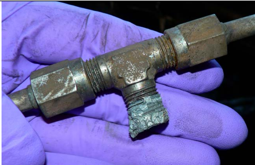
Figure 21. N799AX: Resolidified aluminum filled the threads of the center supernumerary seat threads. The flexible hose to the mask box would have hung from this fitting.
