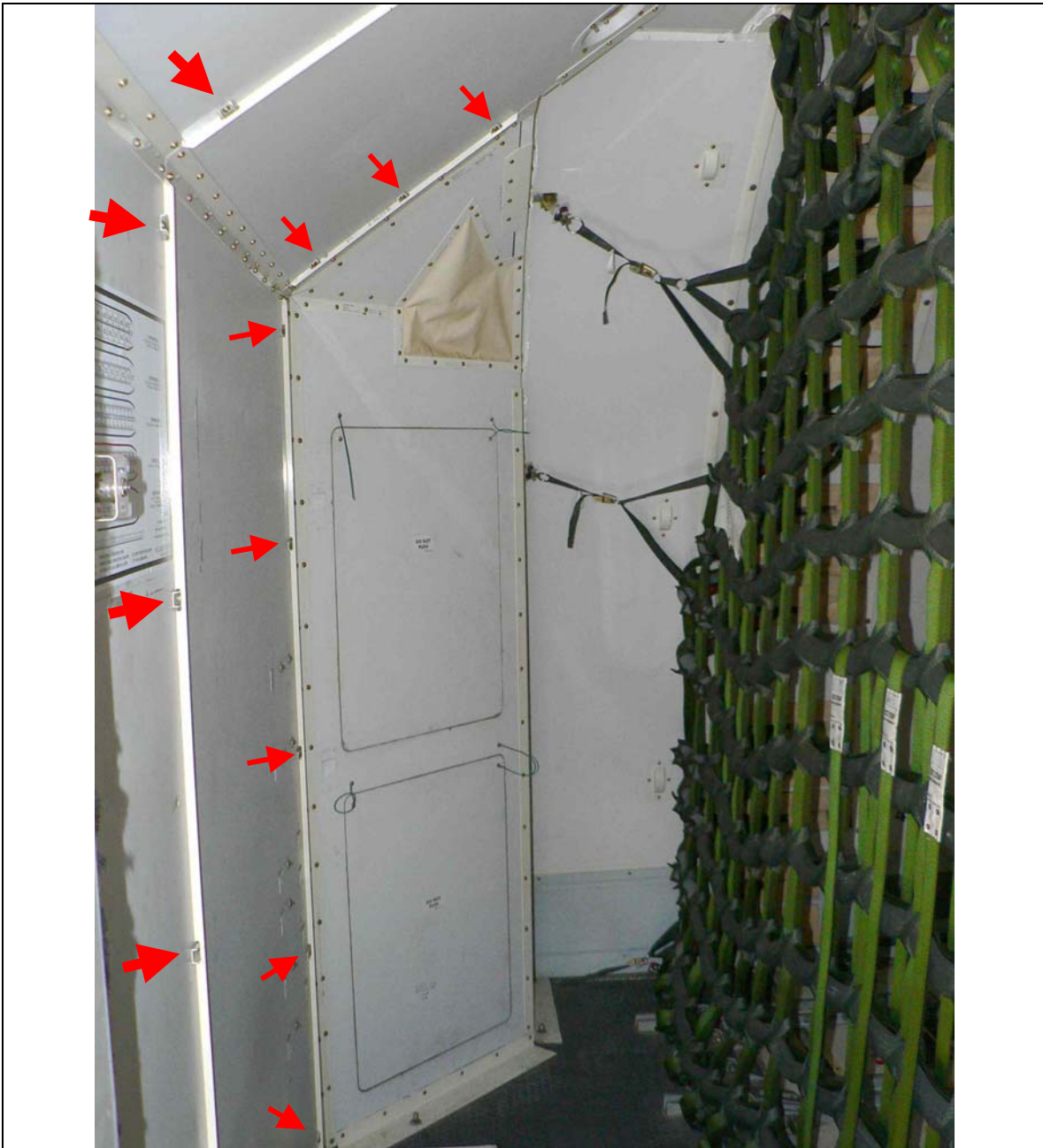
Figure 4. Photo of the aft side of the smoke wall in an exemplar aircraft. The supernumerary compartment and cockpit would be to the left of this wall. The net is the 9-G cargo barrier and the tail is to the right of this photo. The arrows show clips installed through T-strip in a similar airplane, holding the left and right smoke wall panels together. The center-wall clips and T-section had been consumed in the accident aircraft.
