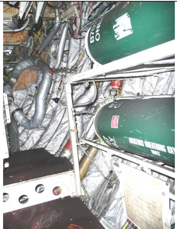
Figure 10. N799AX. The green oxygen bottles circled in Figure 9A are shown from the rear. The upper bottle supplied the supernumerary oxygen system. The top of this compartment is the cockpit floor and the nose landing gear compartment was to the left of this photo.
