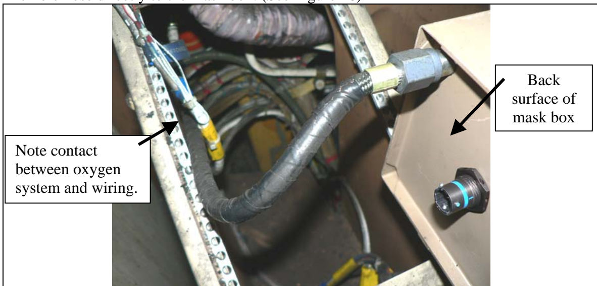
Figure 18. The PVC hose connecting the N799AX left observer's cockpit supplemental oxygen mask box and the stainless steel supply tube. The stainless steel supply tube at the hidden end of this PVC hose is not visible. This tube had been
