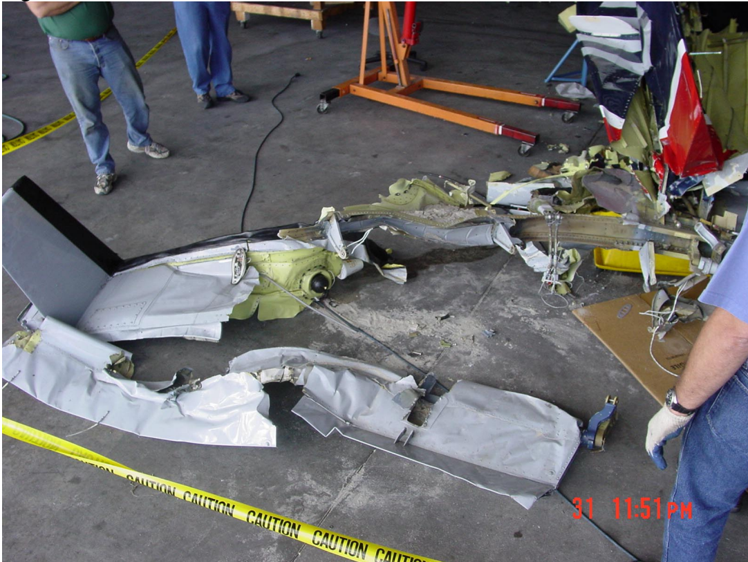
Figure 9. Right Elevator parts after removal from the Horizontal Stabilizer.
