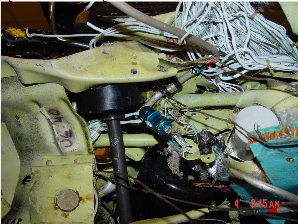
Figure 28. Elevator trim cable drum support and cover.
