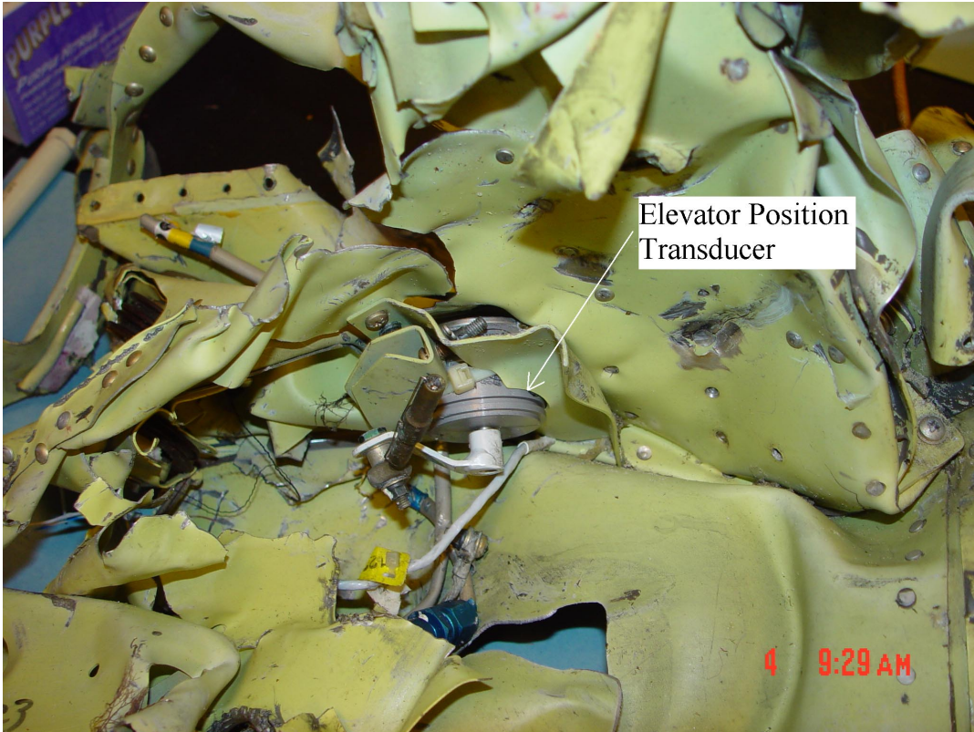
Figure 6. FDR Elevator Position Transducer.
