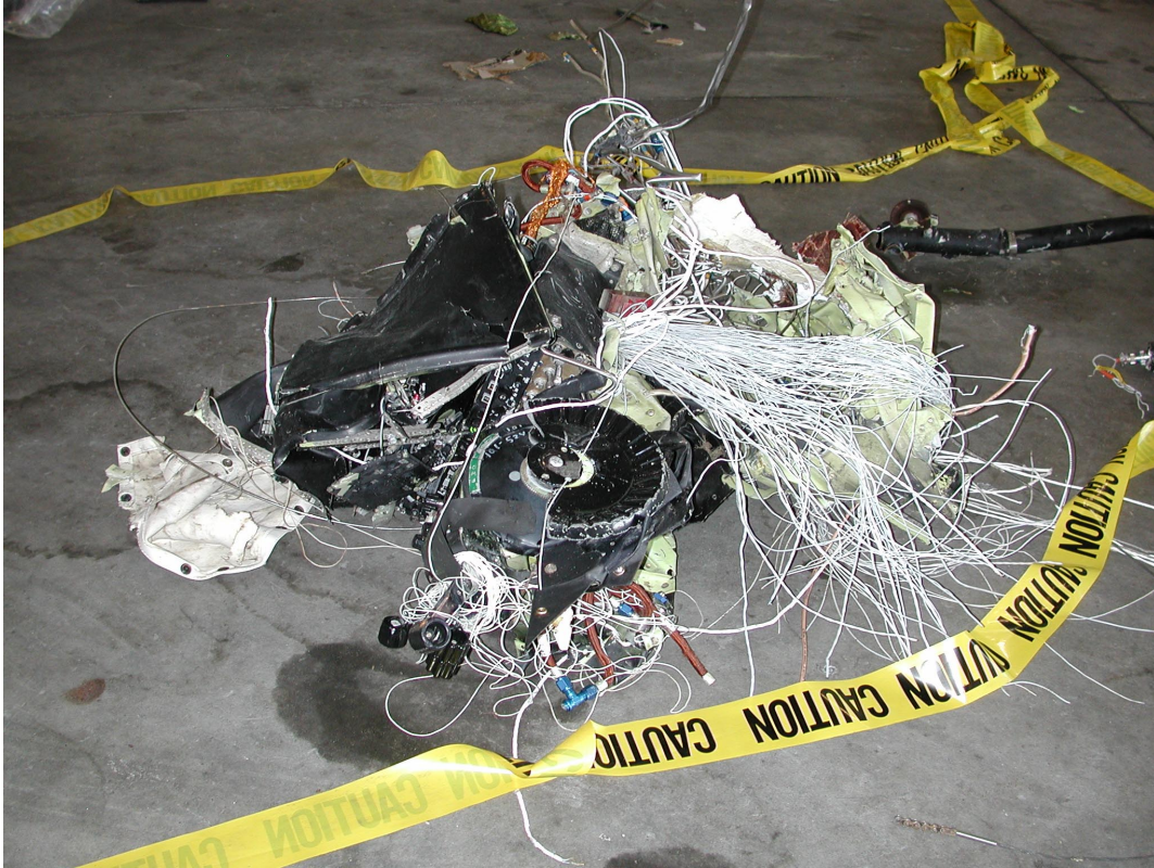
Figure 23. Pedestal as Recovered from Wreckage
