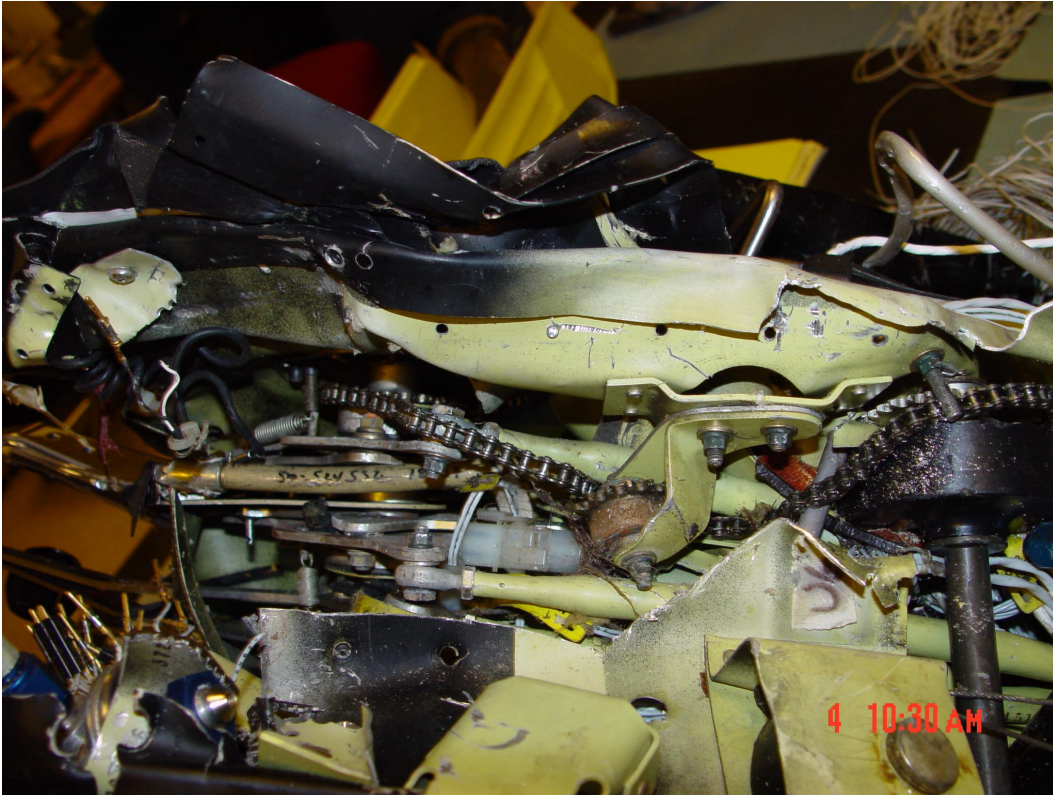
Figure 29. Elevator Trim Drive Chain.
