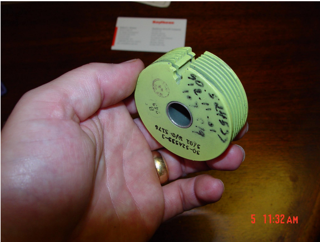
Figure 14. Picture of Non-Slotted Side of New Cable Drum.
