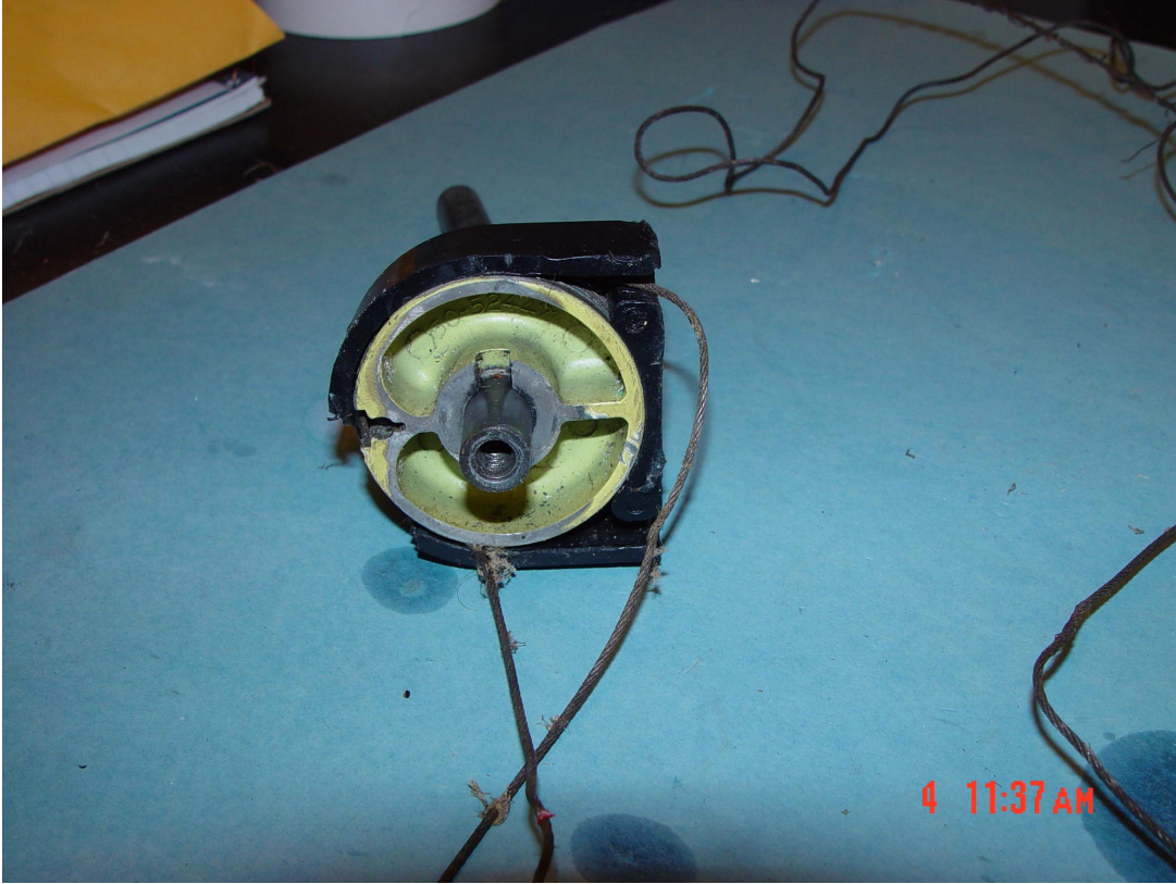
Figure 30. Cable Drum Assembly with Sprocket Removed.
