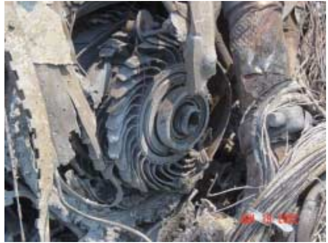
Photo 9: Bent 1 st - & 2 nd -Stage Compressor Blades
