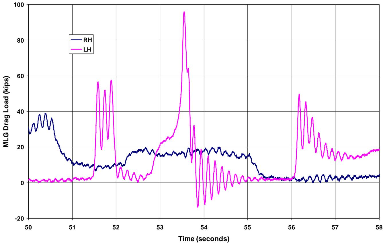
Figure 2 – MLG Drag Load, Flight 1205, April 7, 2007, ID 10.23
