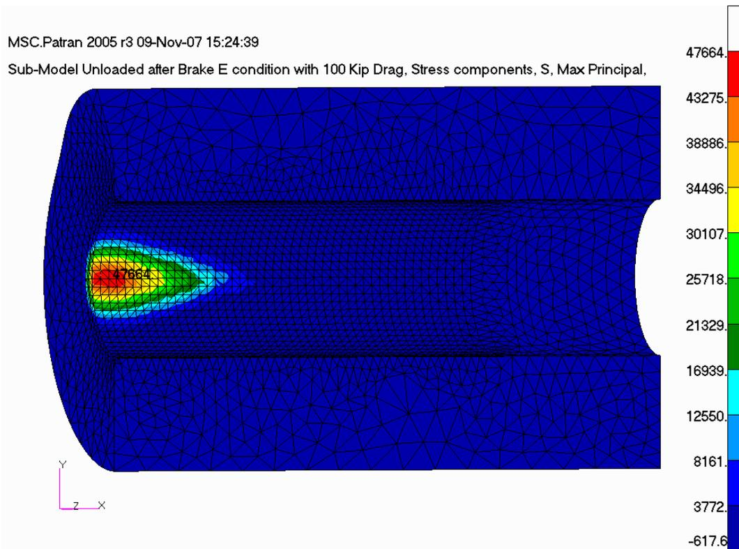
Figure 6 – FEM Results for Residual Stress due to Brake E Condition with 100kips Drag Load
