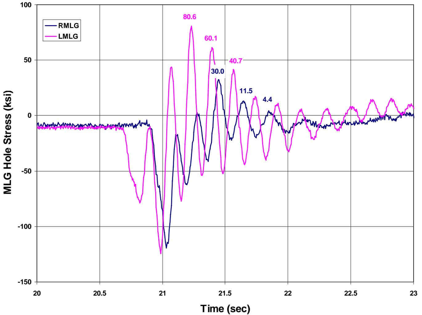
Figure 9 – MLG Hole Stress, Flight 842, February 13, 2007, ID 12.52
