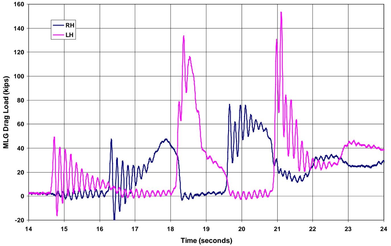
Figure 8 – MLG Drag Load, Flight 308, April 4, 2007, ID 10.14
