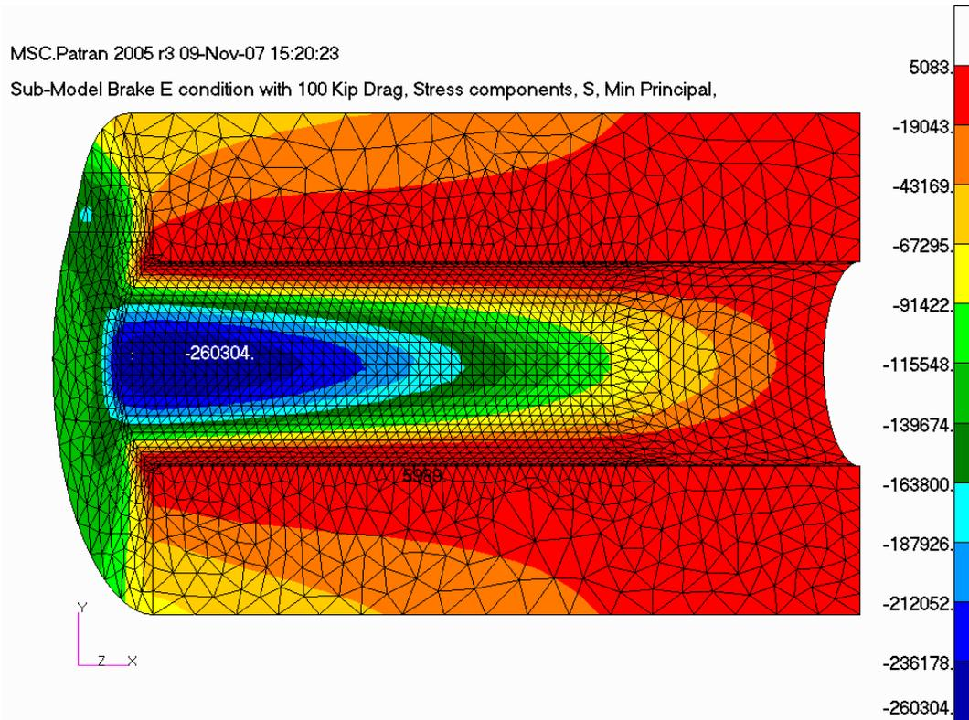
Figure 5 – FEM Results for Brake E Condition with 100 kips Drag Load
