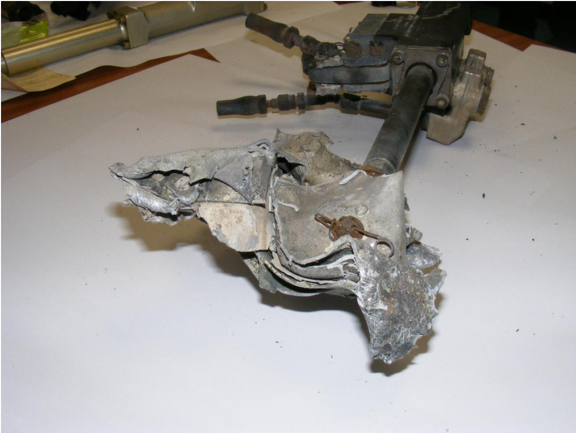
Figure 2 - Safety Pin on Tail Rotor Servo Connection
