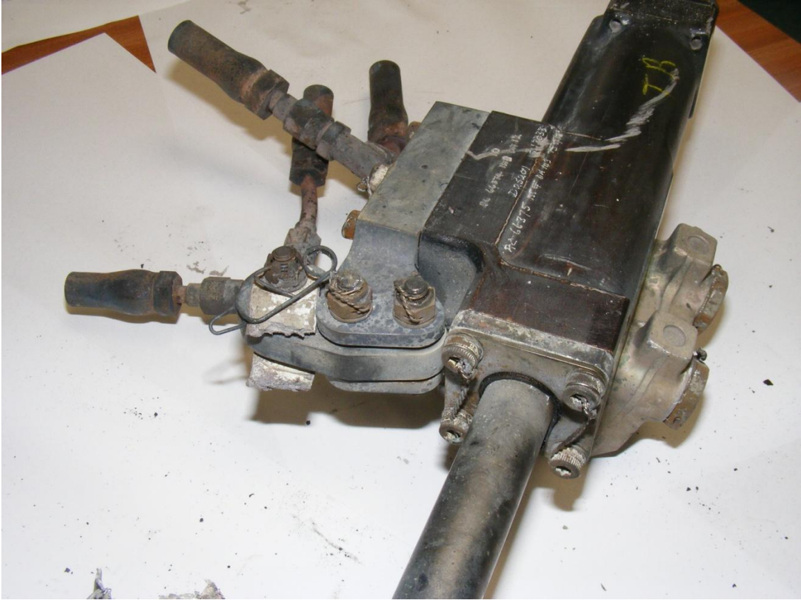
Figure 1 - Safety Pin on Tail Rotor Servo Input Linkage
