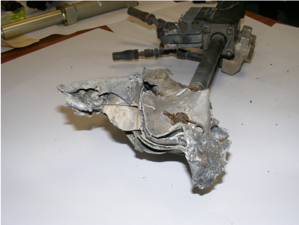
Figure 2 - Safety Pin on Tail Rotor Servo Connection
