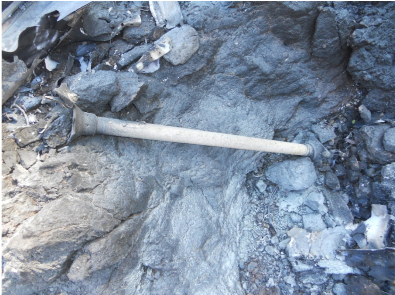
Figure 7 - Tail Rotor Short Shaft
