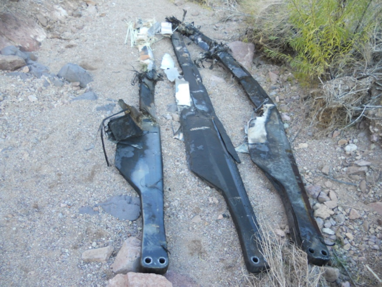
Figure 4 - Main Rotor Blades after removal from the main rotor mast
