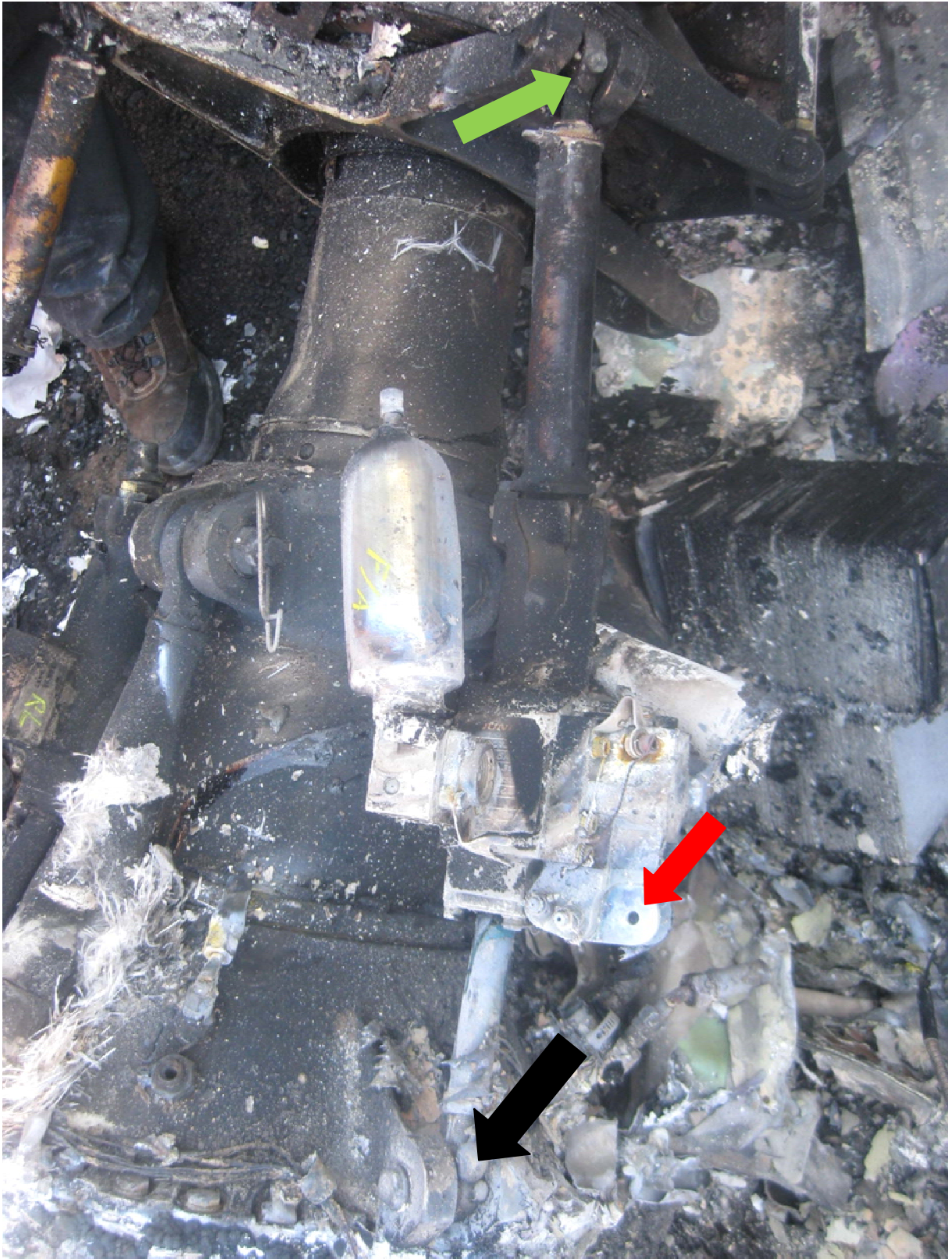
Figure 1 - Fore/Aft Servo Commande Unit, as found in wreckage, noted with connection to swash plate (green arrow), main transmission (black arrow), and input linkage connection (red arrow).
