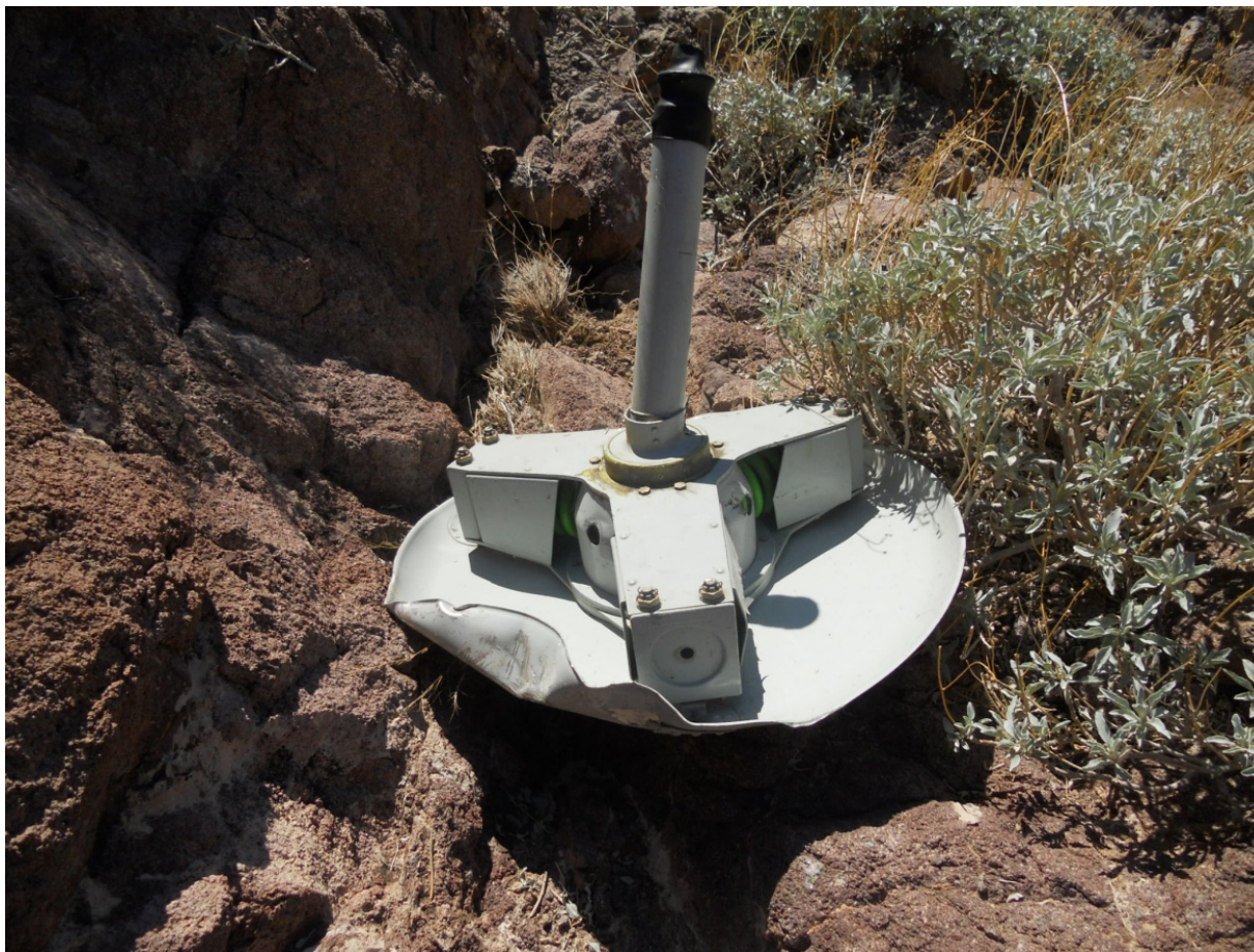
Figure 5 - Main rotor head vibration absorber
