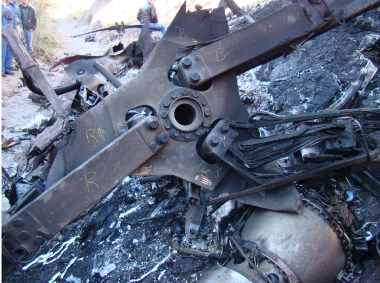
Figure 3 - Main Rotor "Starflex" Hub with letters to indicate each of the star arms (Yellow, Blue, or Red).
