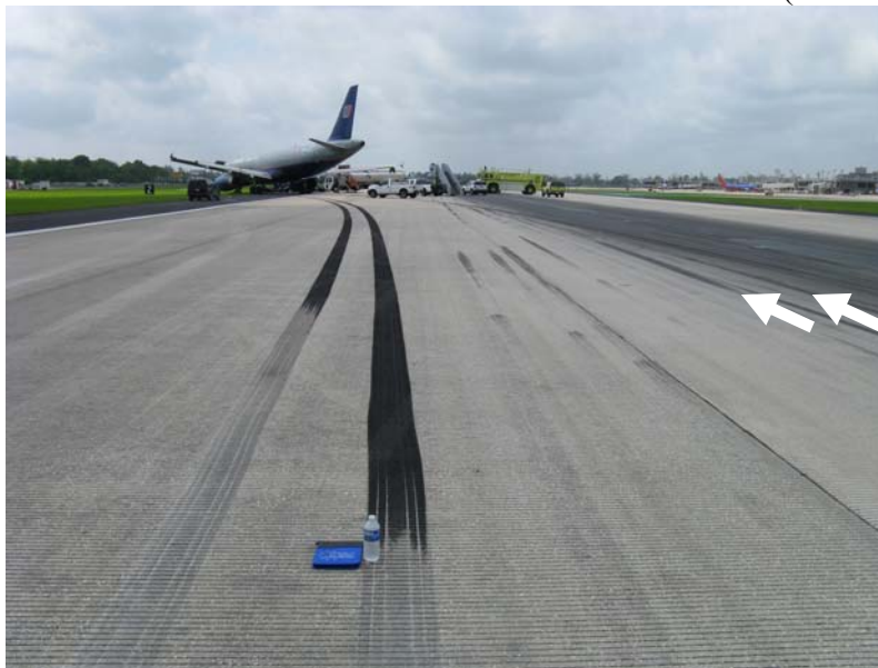
Figure 2. The water bottle is where the overhead photo in Figure 1 is labeled “Heavy Braking Begins – Left Turn.” The white pickup truck is parked on the tire marks that lead to the right set of tires, also shown at the pair of white arrows.
