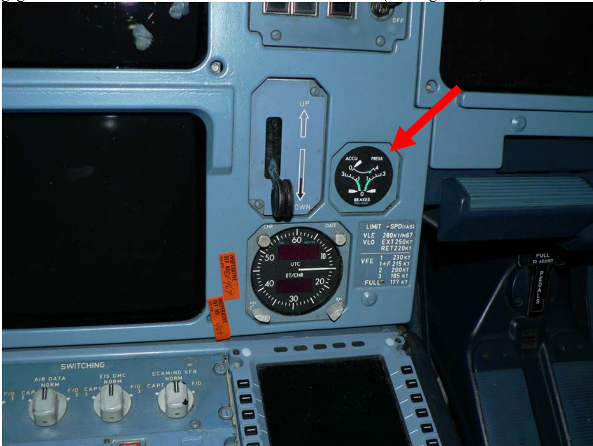
Figure 14. The red arrow points to a gage with three needles that is used to determine brake pressure when landing without the antiskid system.
