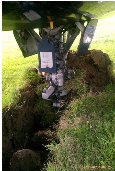
Figure 4. Close up of buried nose landing gear.
