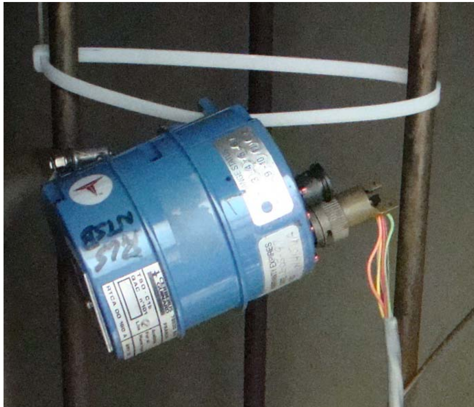
Figure 11. Smoke detector undergoing testing at the FAA Fire Laboratory.
