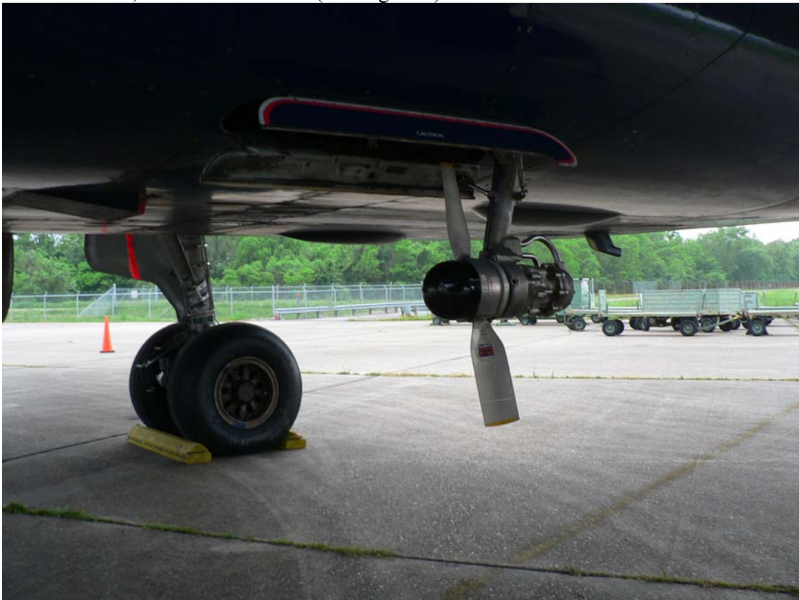
Figure 9. Ram Air Turbine, as found extended beneath the airplane after flight.
