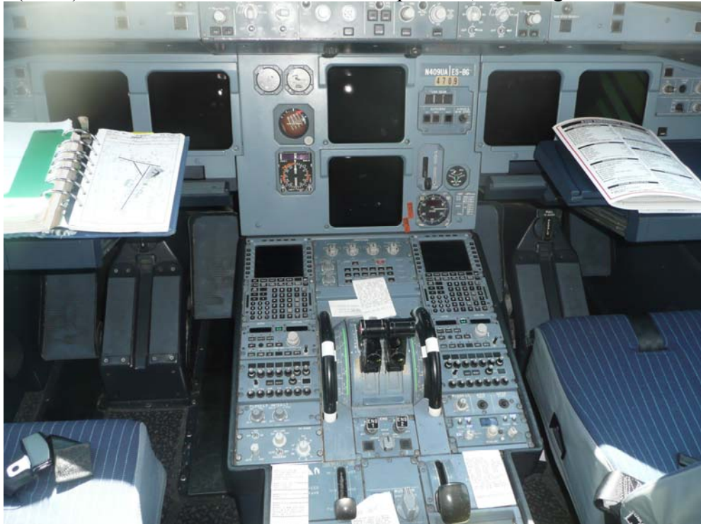
Figure 5. Cockpit, as found. The two vertically oriented Engine Centralized Aircraft Monitoring (ECAM) displays are in the center.
