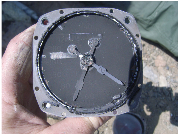
Figure 12 Photograph of the exterior mounted engine torque indicator at the wreckage site
