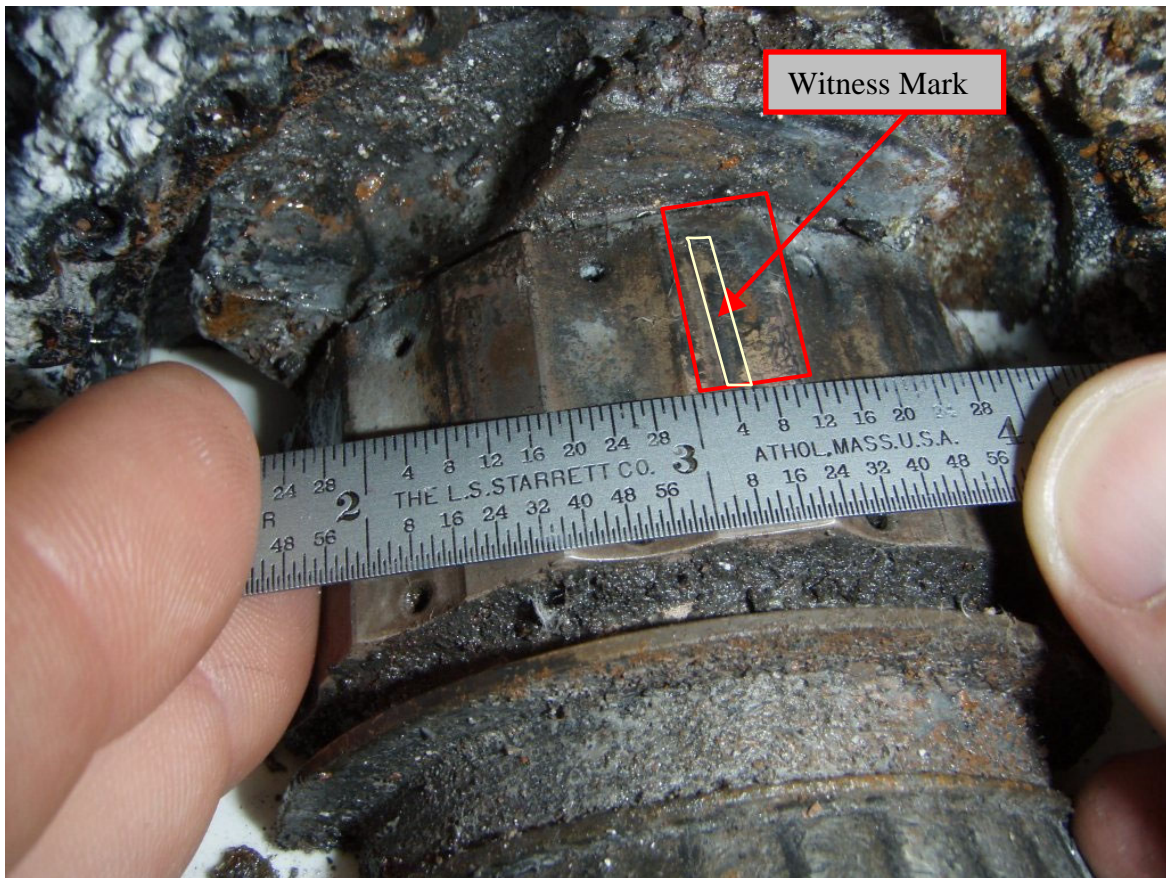
Figure 7 Photograph of the Number 1 IFWU showing the approximate 0.050" witness mark positioned at approximately 0.125" to 0.187" up from beginning of the ramp
