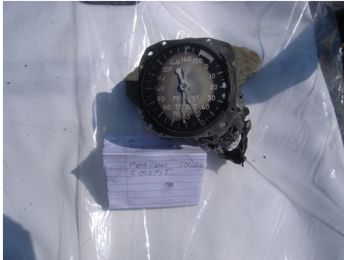
Figure 11 Photograph of a cockpit engine torque indicator at the wreckage site
