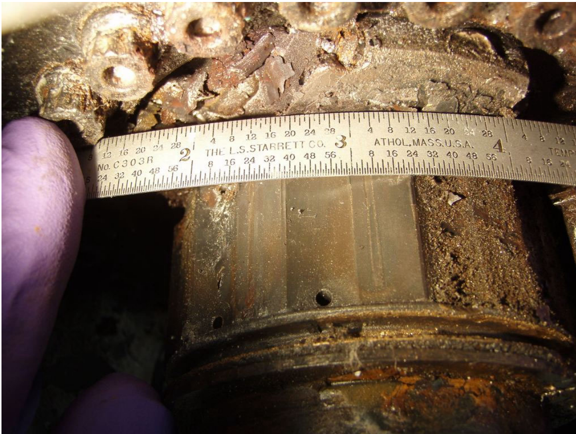
Figure 9 Photograph of Number 2 IFWU showing the 0.050" witness mark positioned at approximately 0.078 to 0.140" up from beginning of ramp
