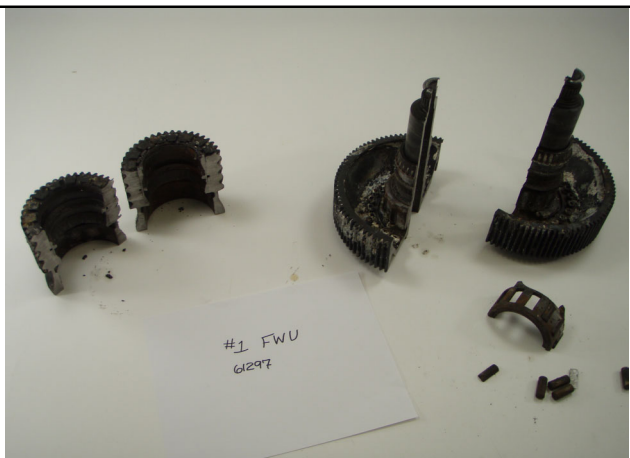
Photograph of Number 1 IFWU after being cut in half
