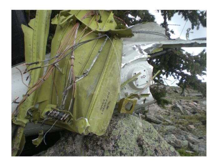
The antenna missing from the fairing shown in the picture below was recovered within 20' of the tail boom.
