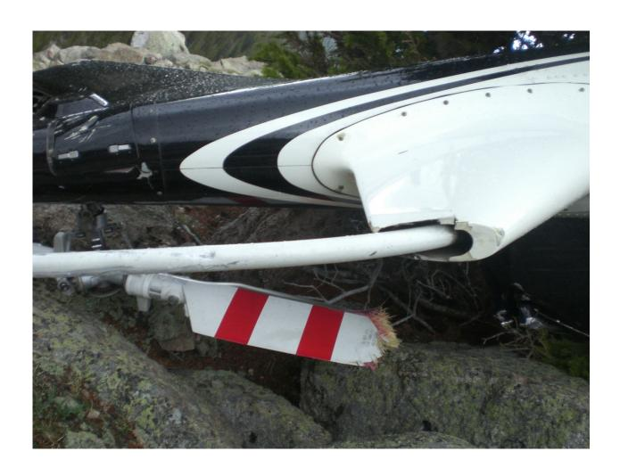
In this photo of the tail boom, you can see that the tail cone is missing. The tail cone was recovered approximately 90' uphill from the tail boom.
