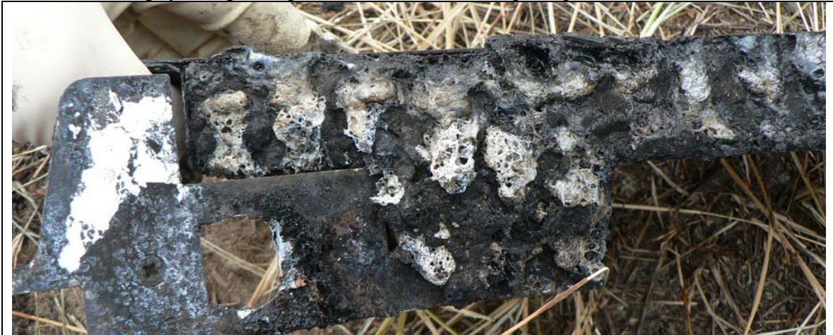
Figure 2A. Left portion of annunciator panel from accident airplane, showing melted and charred annunciators prior to excavation and removal.
