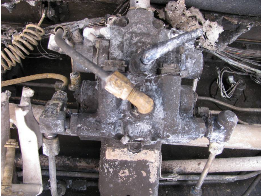
Photo 18. Flap Block Valve
