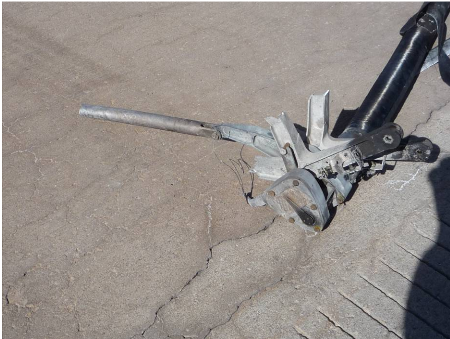
Photo 17. Flap Asymmetry Detector
