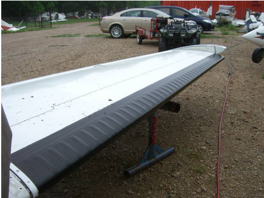
Photo 29. Left Horizontal Pneumatic Boot
