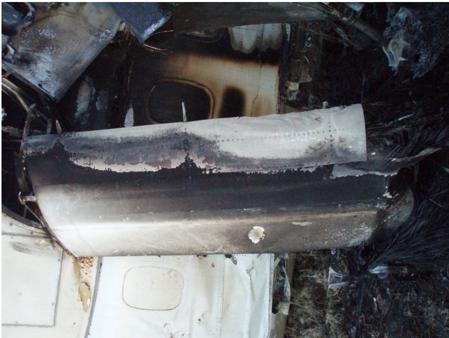
Photo 10. Right Wing Half Inboard Section of Inboard Flap
