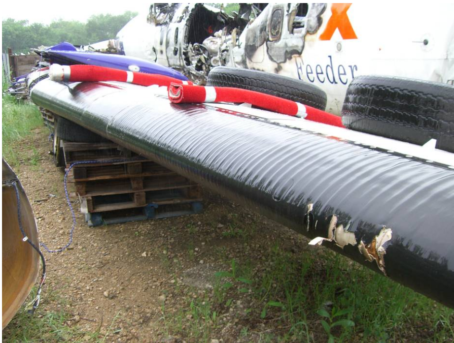
Photo 31. Left Wing Pneumatic Boots
