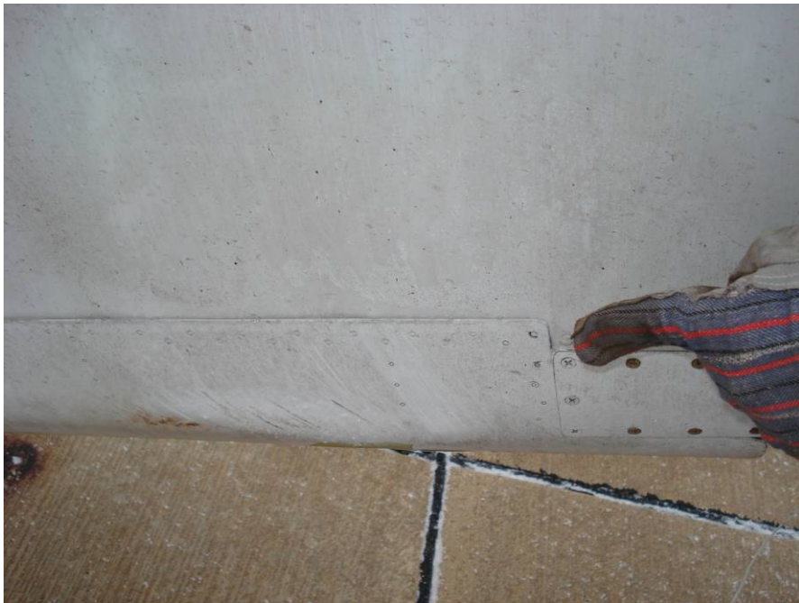
Photo 20. Ice on Underside of Right Aileron (Provided by FAA)
