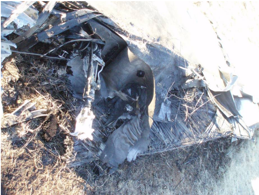
Photo 12. Wing Inboard Portion of Outboard Flap
