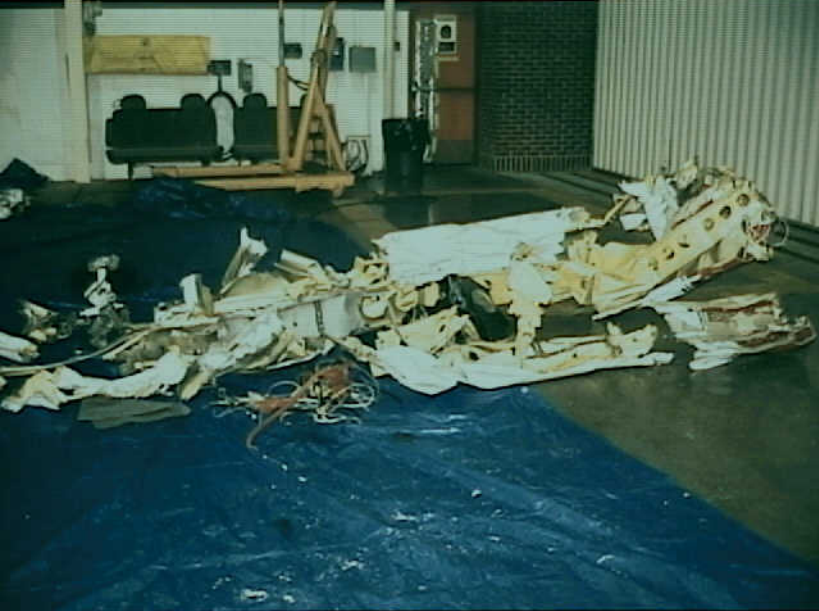
Airworthiness - Photo 9. Close-up view of the leading edge skin of the left wing (view from forward looking aft). Note hydrodynamic deformation in aft direction. (NTSB-I12)
