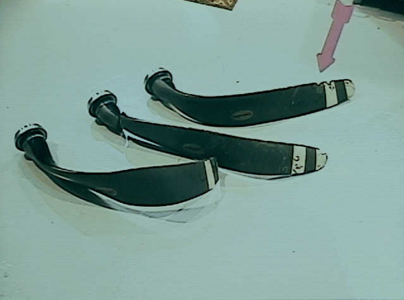
Airworthiness - Photo 25. Close-up view of leading edge damage of propeller blade no. 1. (NTSB-CC)
