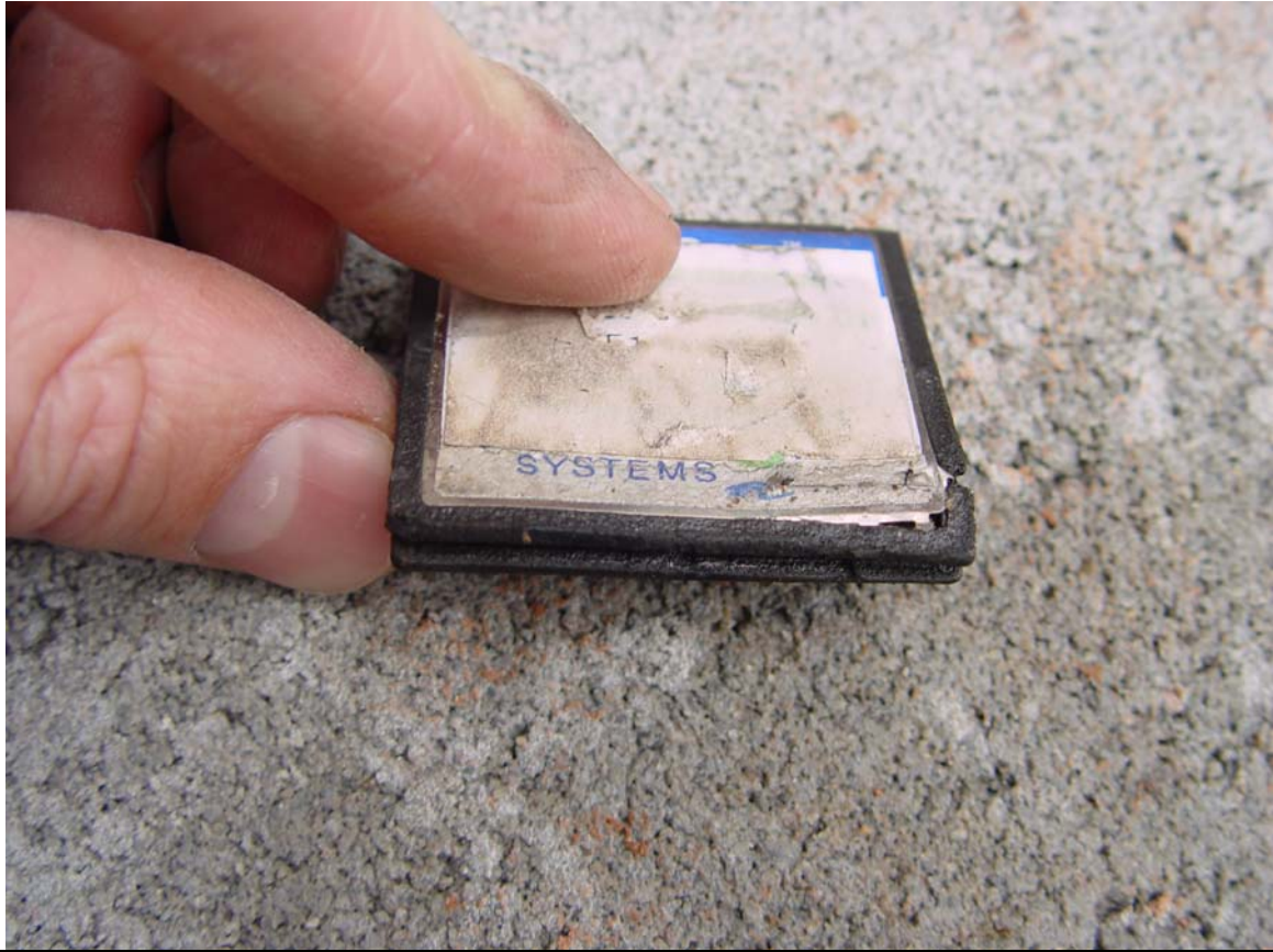
Flash Memory module from MFD
