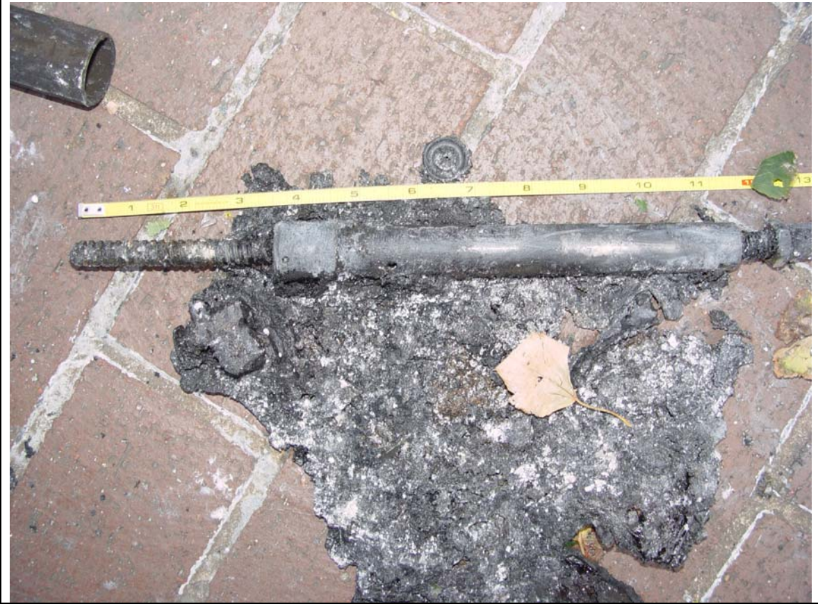
Linear flap actuator as found at the accident site
