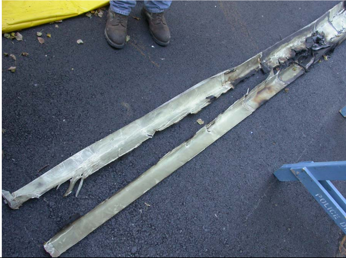
Photograph of Wing Spar showing split
