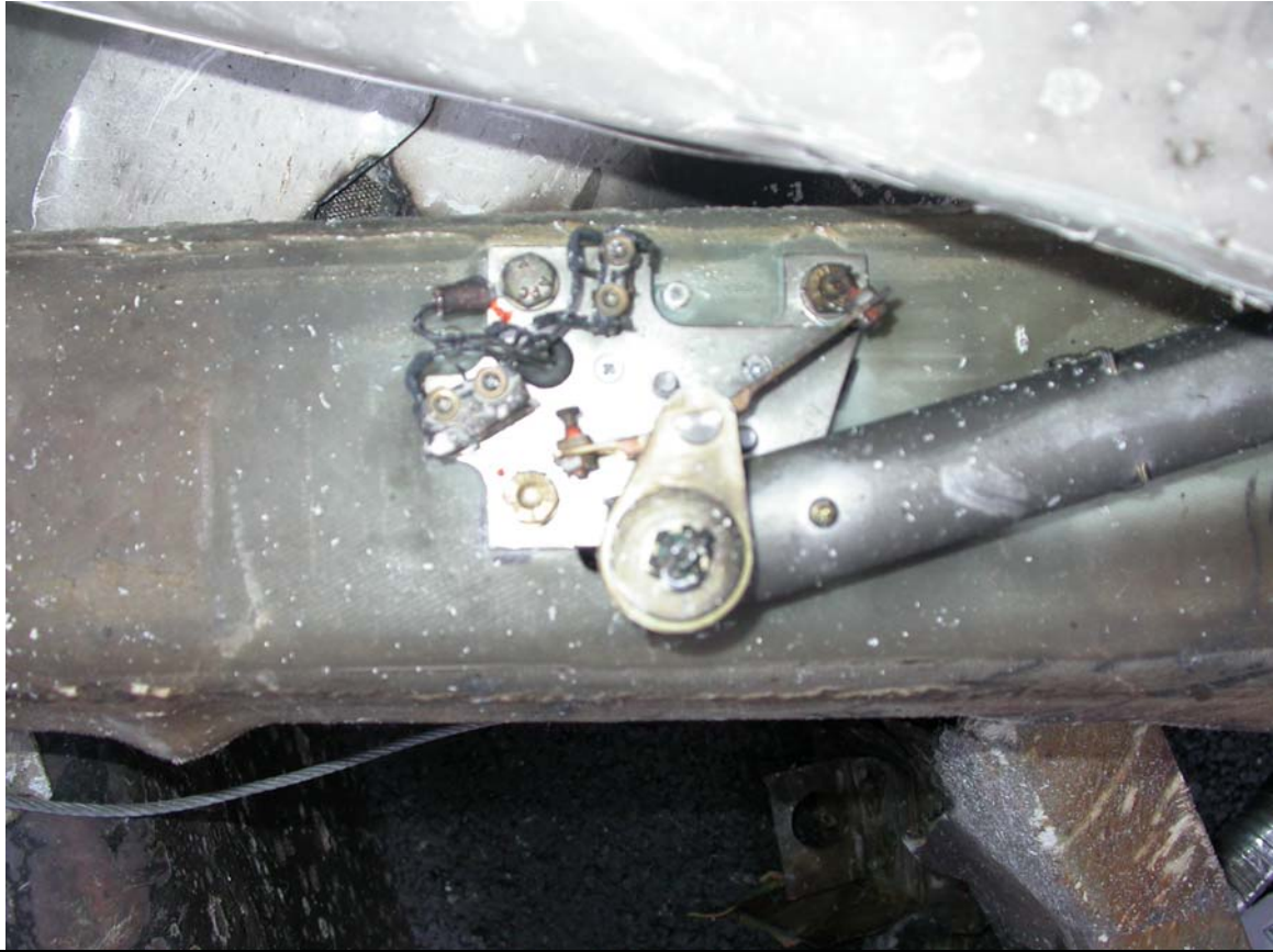
Aircraft N929CD - Left Aileron showing position of roll trim motor
