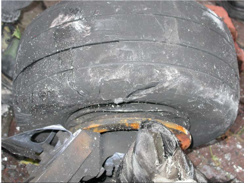
Left Main Gear Wheel Showing Flat Spot
